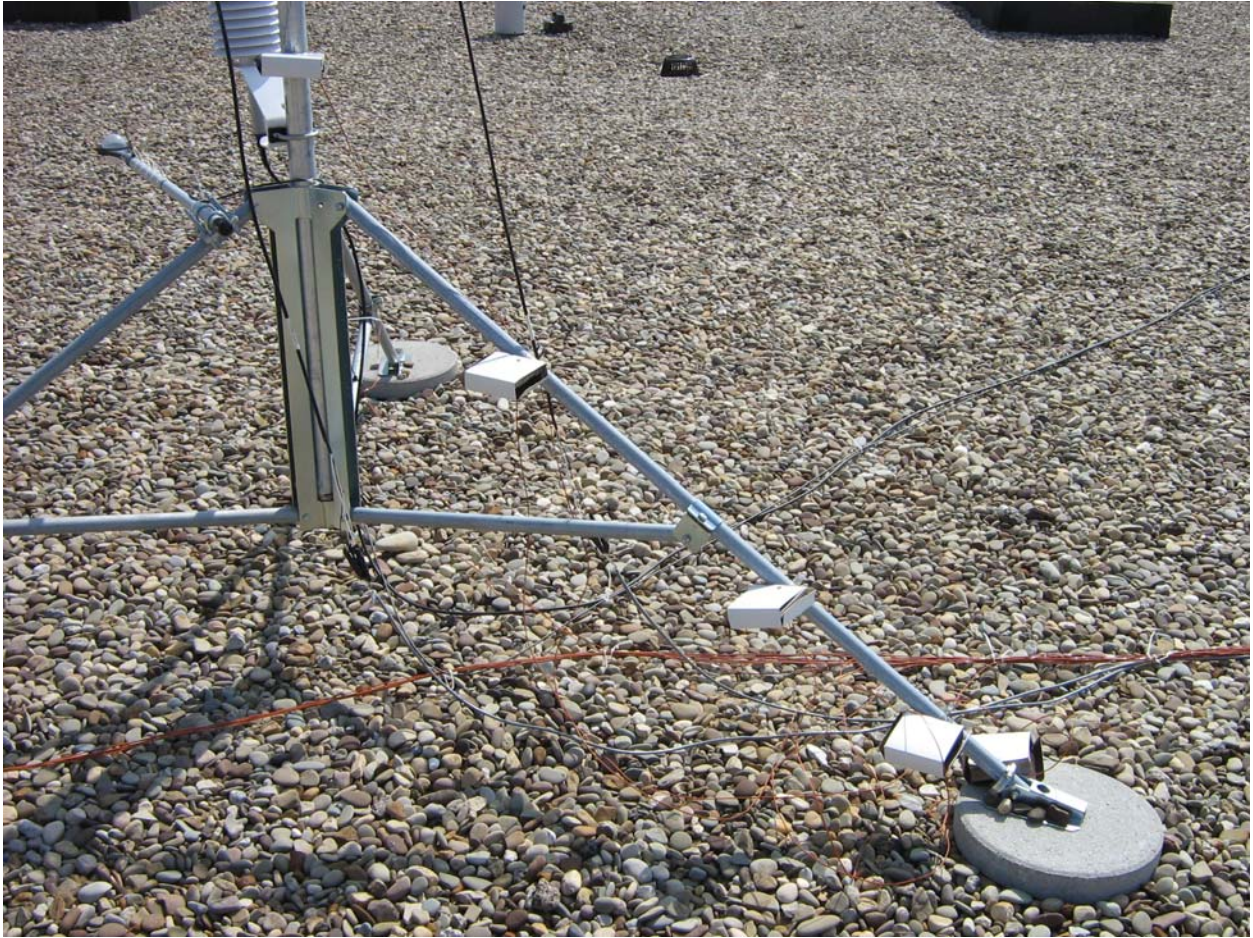
Figure 22 - Thermocouples Installed on a Control Roof Tripod
