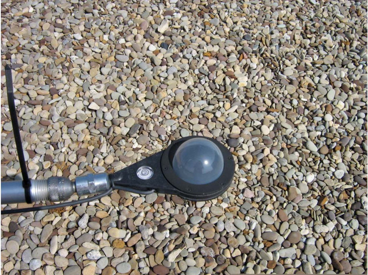
Figure 27 - Net Radiometer Installed on Green Roof Tripod
