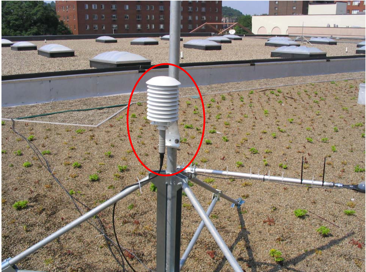
Figure 26 - Temperature/RH Sensor (Circled) Installed on a Green Roof Tripod
