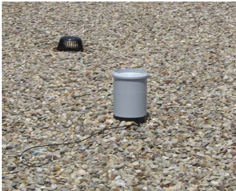
Figure 11 - Rain Gauge Installed on the Green Roof
