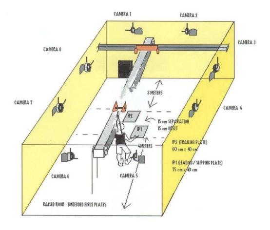
Moore CT. Schematic illustration of the testing area of the Human Movement and Balance Laboratory, University of Pittsburgh, showing eight motion tracking cameras and harness safety system. 2008.
