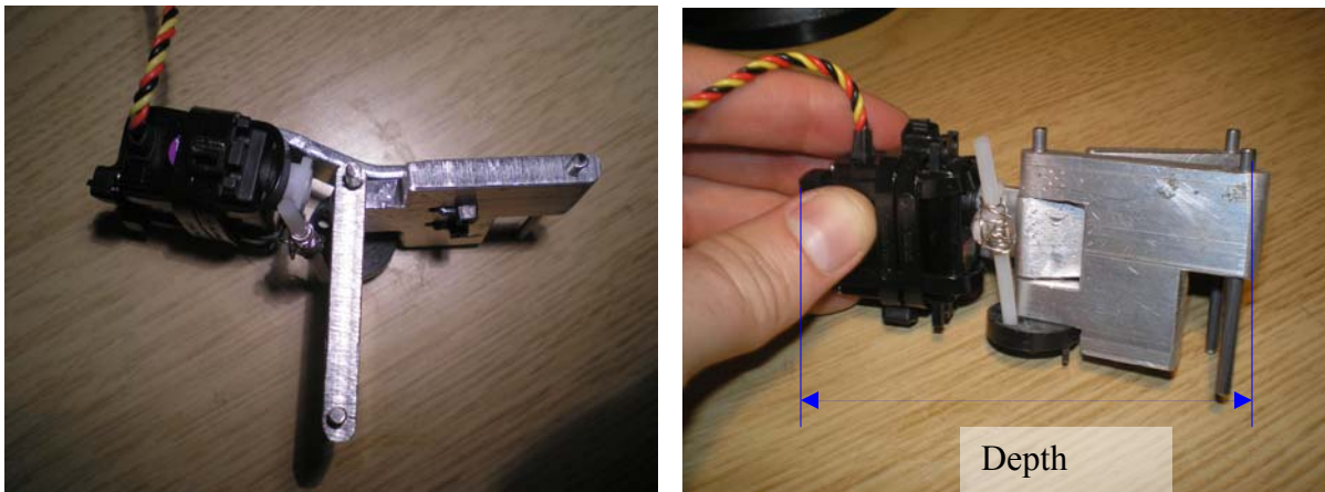
Figure 3.5. Top and side view of Servo Link
