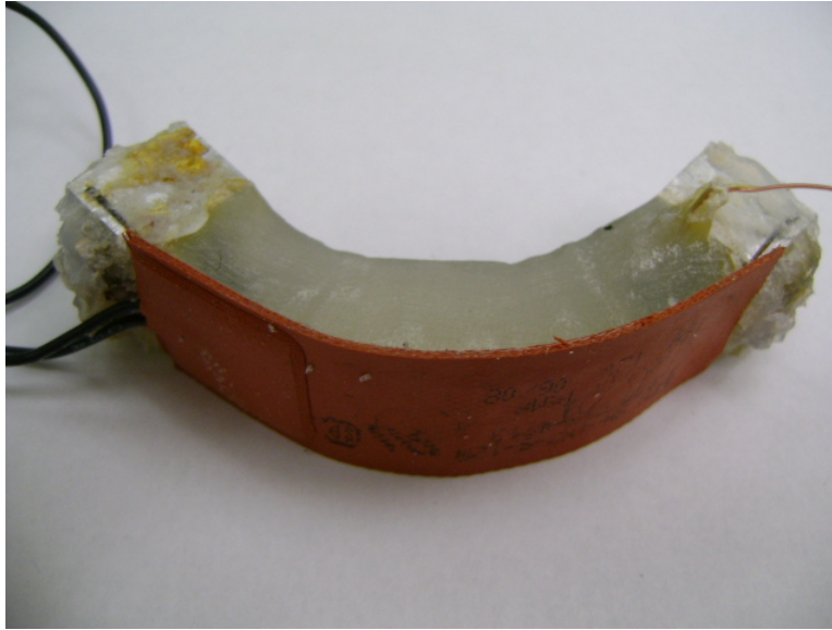
Figure 4.3. Silicone pad butted against nitinol side of Smart Link
