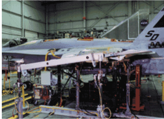
Figure 2.9. Morphing F-18 fighter wing in torsion (AIAA, 2008)
