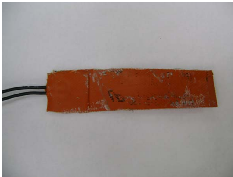
Figure 4.2. 3 inch long silicone heating pad trimmed to approximately 0.71 inches high
