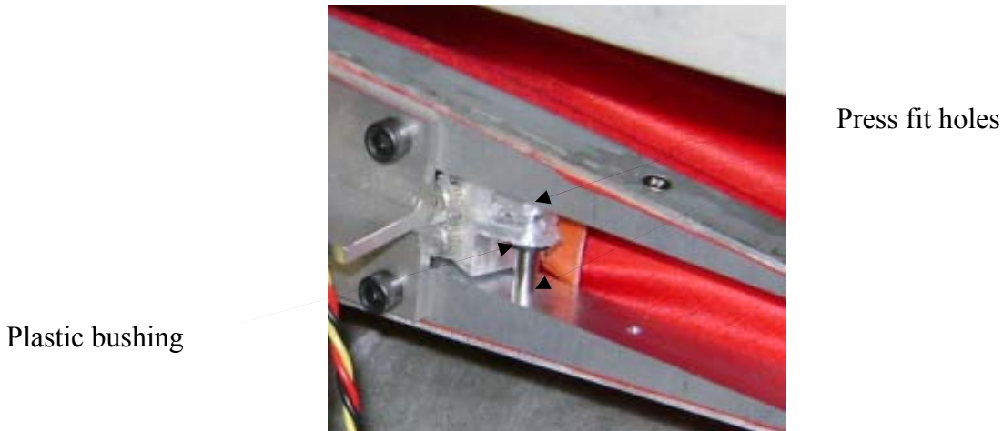
Figure 5.3. Location of press fit holes in rib and bushing in link
