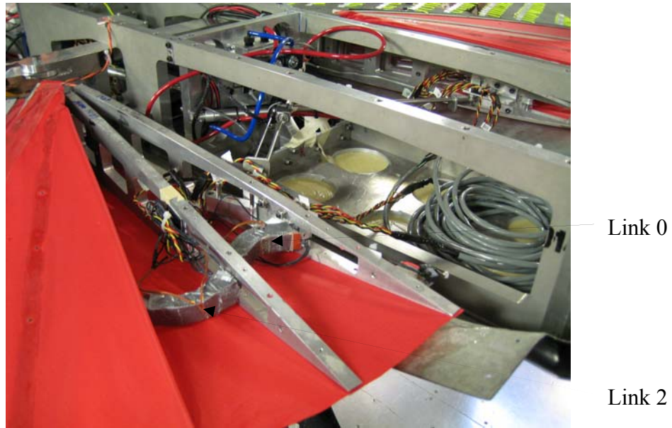
Figure 8.1. Labeled links (one of each pair) situated inside the morphing wing during test preparation
