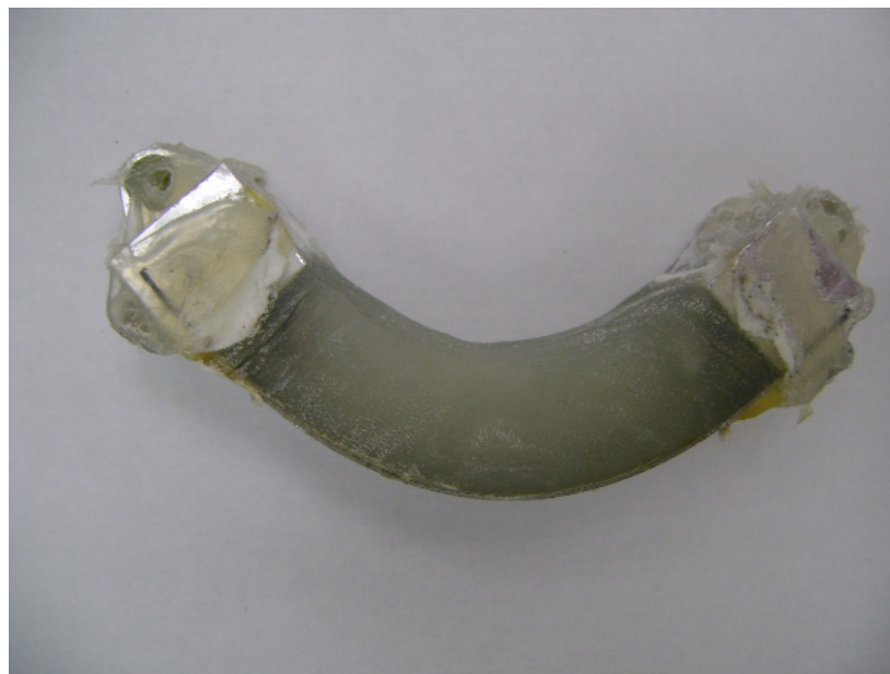
Figure 6.3. Final Smart Link after fabrication process
