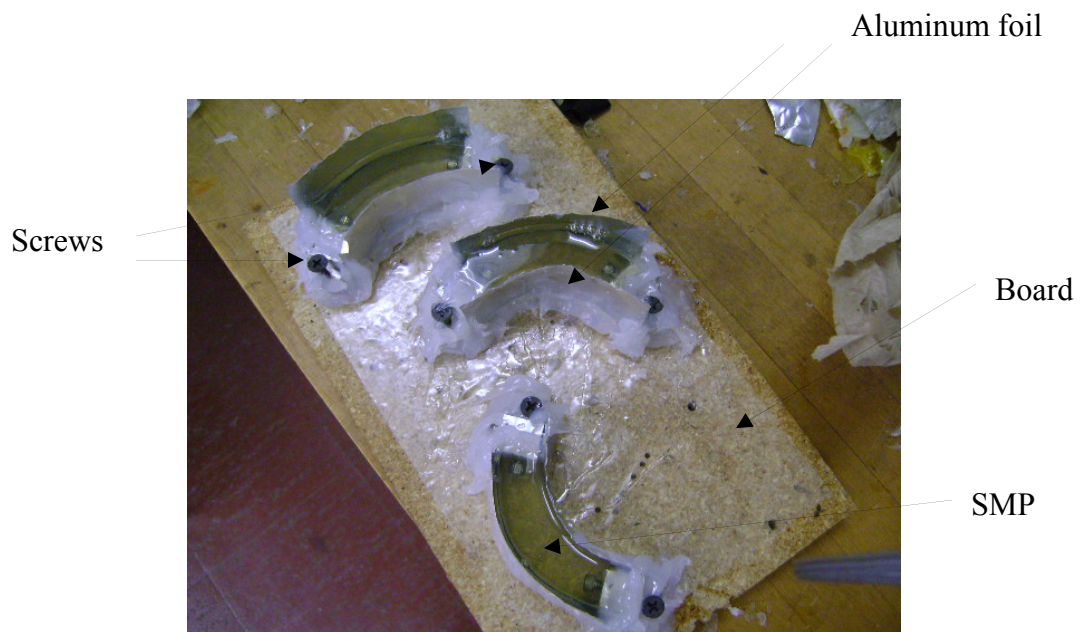
Figure 6.2. Smart Links at 95 degree initial interior angle after curing process is complete
