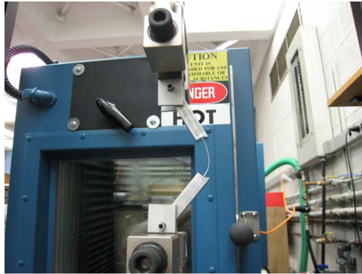
Figure 3.11. Continuous aluminum link without SMP in load frame
