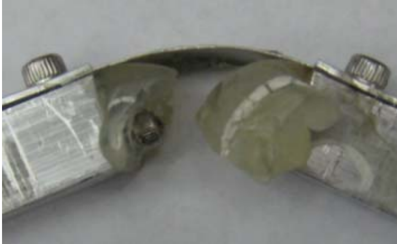
Figure 3.15. Ruptured SMP after thermal cycling and compression
