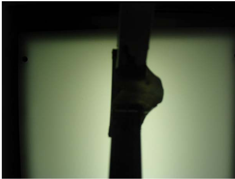
Figure 3.16. Buckling of SMP during compression test as link bends away from camera view
