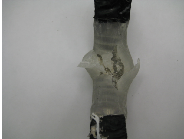
Figure 3.18. Failure of SMP during nichrome activation
