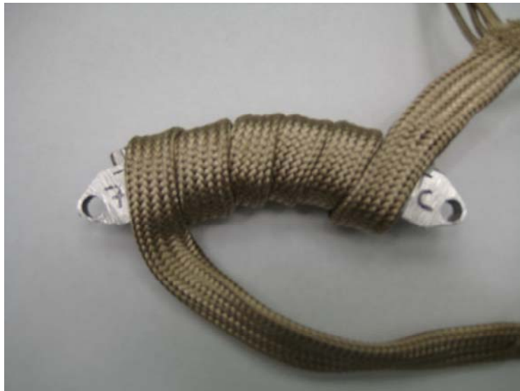
Figure 4.1. Smart Link wrapped with heating tape
