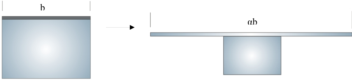
Figure 7.5. Conversion of cross section to entirely SMP based on moduli ratio \alpha
