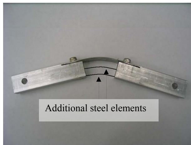
Figure 3.13. Smart Link with additional spring steel elements
