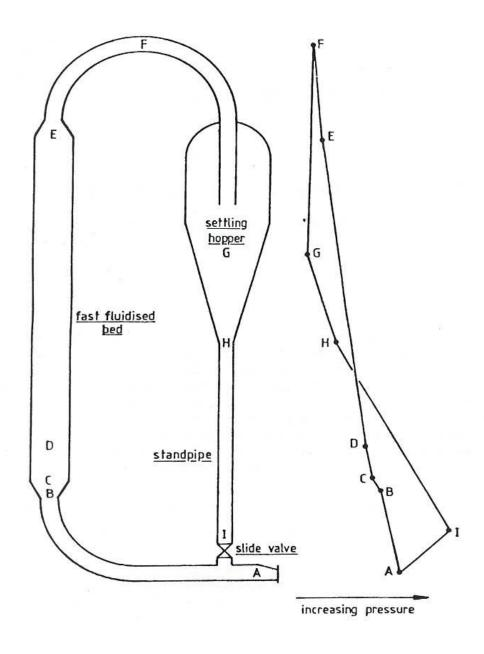
Figure 2.3 Circulating Fluidized Bed Reactor [28].
