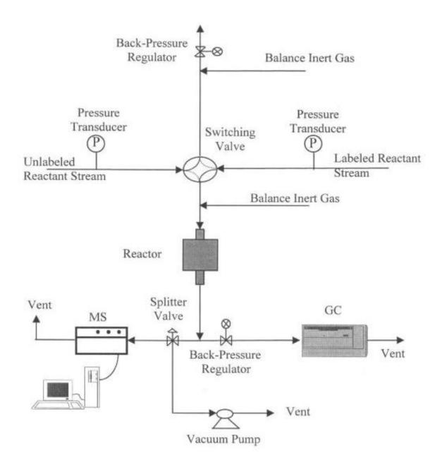
Figure 2.6 Schematic Diagram of Typical SSITKA System [82].
