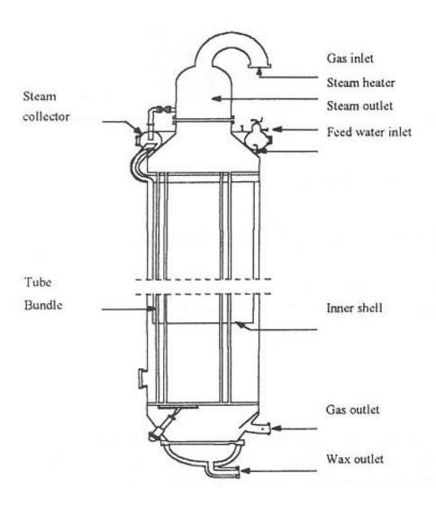
Figure 2.1 Tubular Fixed Be d (ARGE) Reactor [23].
