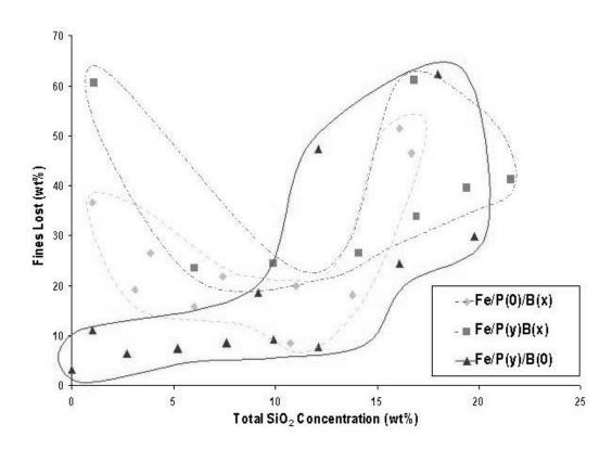
Figure 7.1 Attrition of all Spray-Dried Fe Catalysts in the Calcined State Previously Studied.
