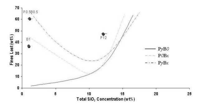
Figure 7.2 Attrition in the Calcined State of the Catalysts Selected for this Study.
