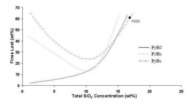
**Figure 6.1** Attrition of P8B8 in the Initial Calcined State Referenced to Other Spray-Dried Fe Catalyst Formulations.
