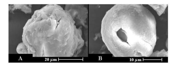
**Figure 5.6** SEM Micrographs of Typical SiO<sub>2</sub> Structures after Acid Leaching [Fe/P(12)]: [A] Typical Structure, [B] Particle with Interior Hole.
