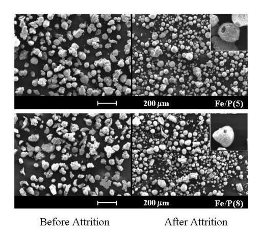
Figure 5.3 SEM Micrographs of Fe/P(5) and Fe/P(8) before and after Attrition.
