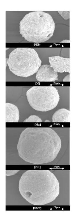
Figure 6.7 SEM Micrographs of Calcined and Pretreated Samples of P8B8.
