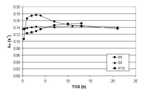
Figure 8.6 Effect of Pretreatments on the Development of Intrinsic Site Activity with TOS.
