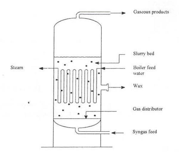
Figure 2.2 Slurry Bubble Column Reactor [23].
