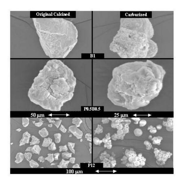
**Figure 7.7** SEM Micrographs of the Original Calcined and CO-Pretreated Catalysts after Acid Leaching.
