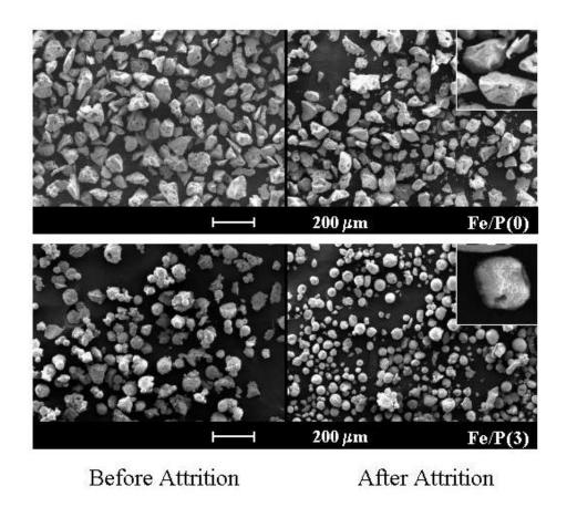
**Figure 5.2** SEM Micrographs of Fe/P(0) and Fe/P(3) before and after Attrition.
