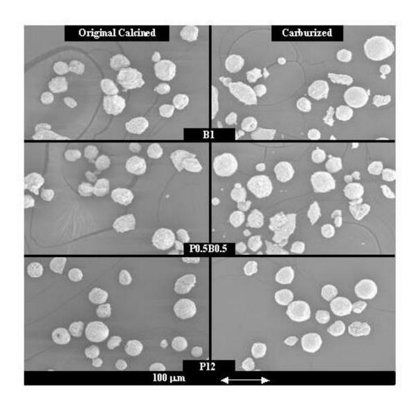
**Figure 7.5** SEM Micrographs of all Catalysts Studied, Comparing their Original Calcined and CO-Pretreated Forms (Low Magnification).
