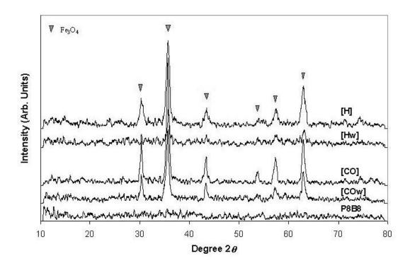
**Figure 6.4** XRD Patterns of Calcined and Differently Pretreated P8B8 Catalysts after Recalcination.
