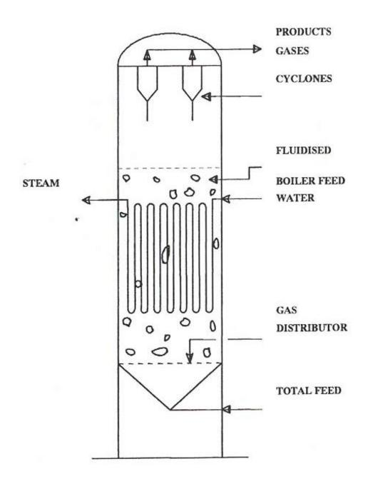
Figure 2.4 Fixed Fluidized Bed Reactor [28].
