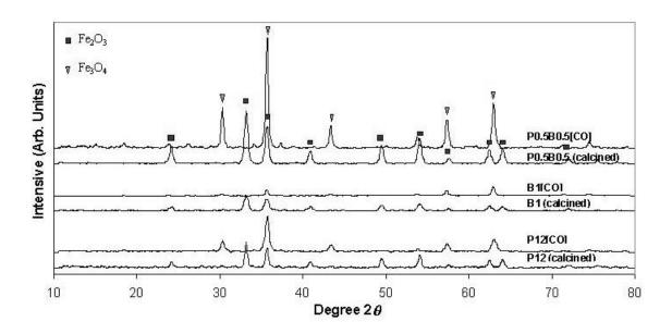
**Figure 7.4** XRD Patterns of B1, P0.5B0.5, and P12 Catalysts in both the Original Calcined and CO-Pretreated Forms after Recalcination.
