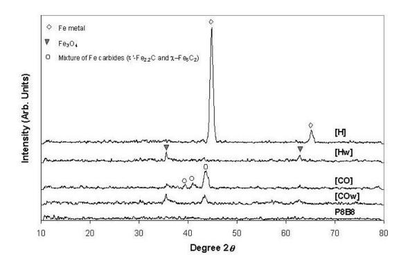
**Figure 6.3** XRD Patterns of Calcined and Differently Pretreated P8B8 Catalysts After Passivation.
