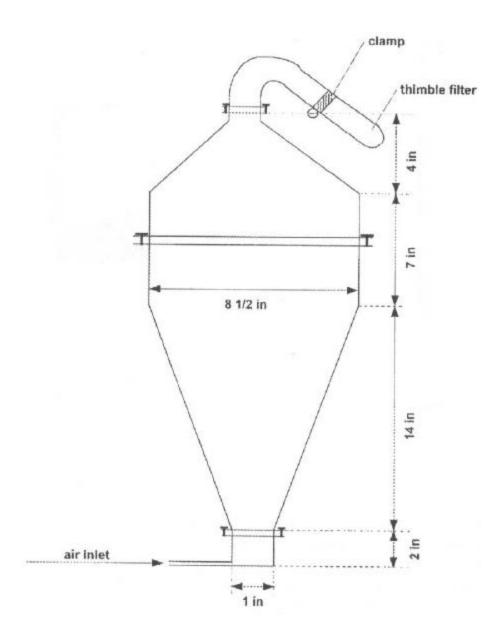
Figure 4.2 Jet Cup Attrition Testing System [11].
