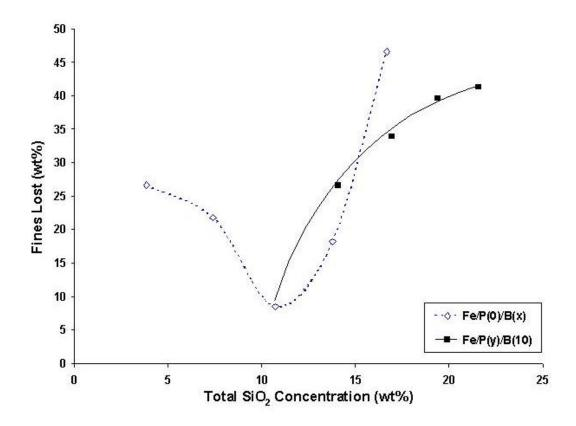
**Figure 2.5** Attrition Test of Fe FT Catalysts [60].
