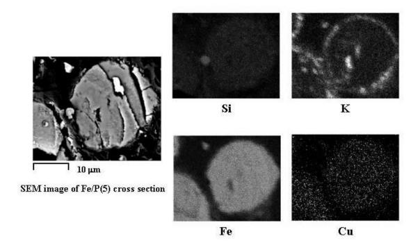
**Figure 5.5** EDXS Results for the Cross Section of a Typical Fe/P(5) Particle.
