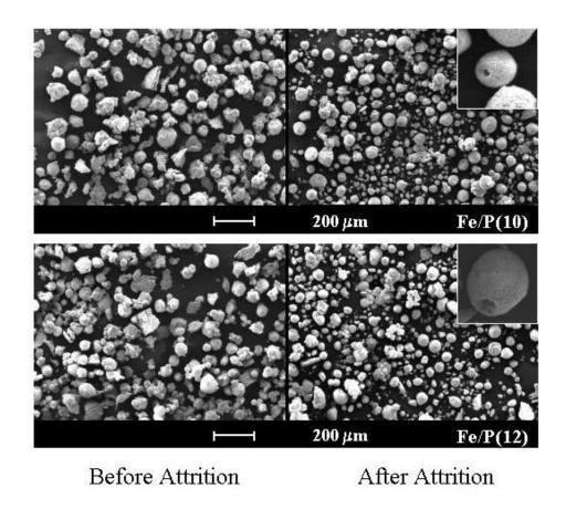
Figure 5.4 SEM Micrographs of Fe/P(10) and Fe/P(12) before and after Attrition.
