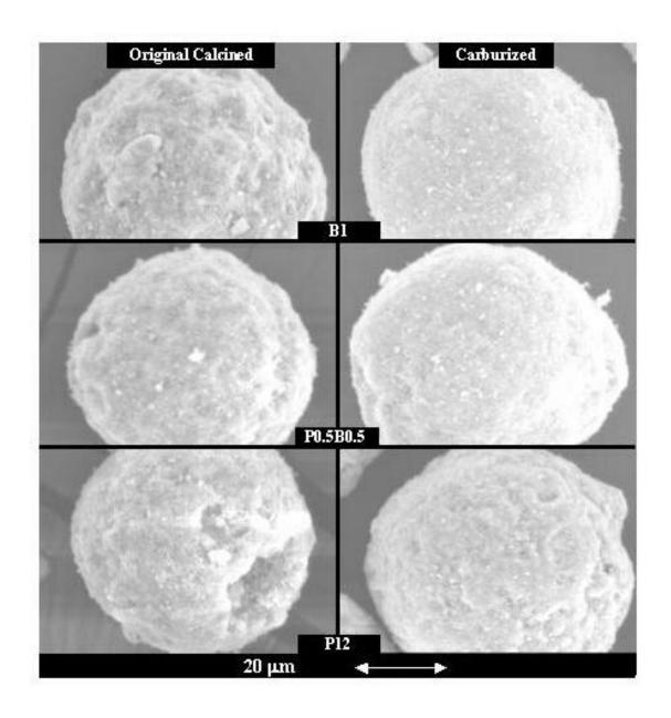
**Figure 7.6** SEM Micrographs of all Catalysts Studied, Comparing their Original Calcined and CO-Pretreated Forms (High Magnification).
