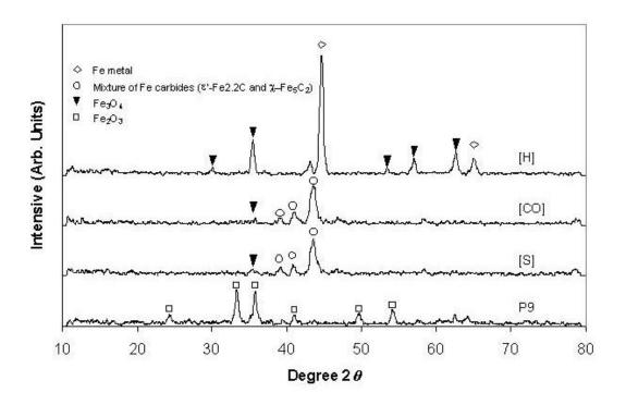
Figure 8.1 XRD Patterns of the Original Calcined and Differently Pretreated Catalyst Samples.
