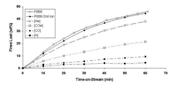
Figure 6.2 Attrition of Calcined and Differently Pretreated P8B8 Catalysts.
