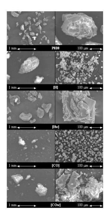
Figure 6.8 SEM Micrographs of Calcined and Pretreated Samples of P8B8.
