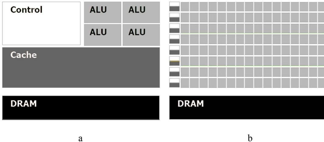
Figure 5.5: Structural organization of a CPU and a GPU, (a) CPU, (b) GPU
