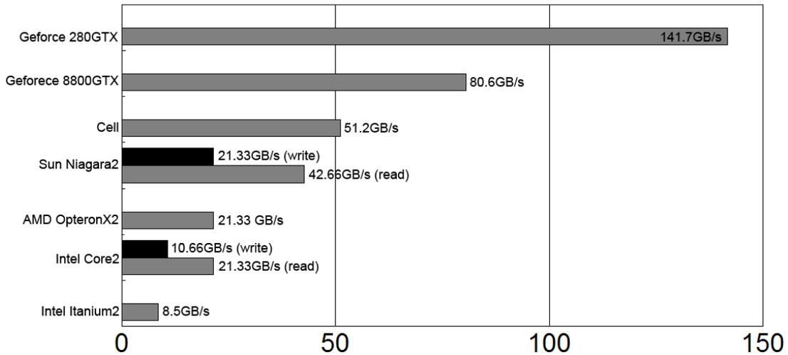
Figure 5.7: Comparison of memory bandwidth for different system
