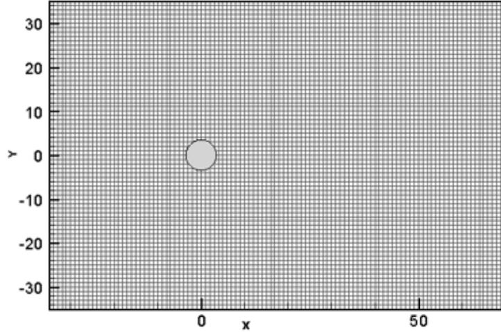
Figure 3.4: Schematic of the computational area for steady flow over a circular cylinder.
