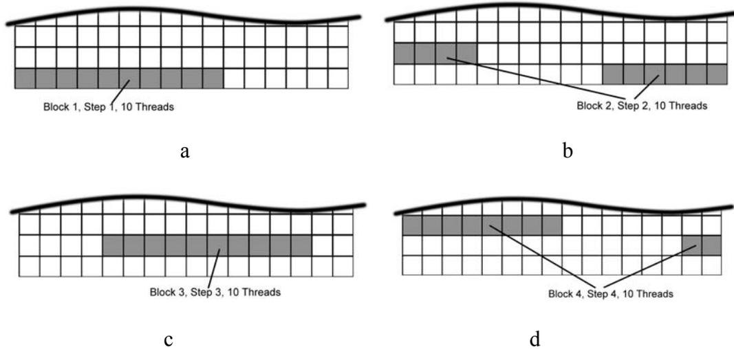
Figure 5.10: Demonstration of block division for CUDA
