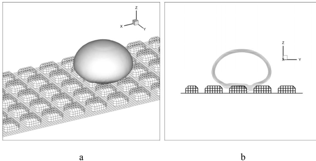
Figure 5.26: (a) liquid droplet on hydrophobic surface, (b) a cross section of droplet
