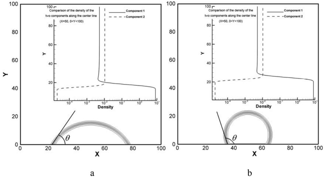
Figure 4.8: Position of the interface of the two components on a hydrophilic and hydrophobic surface, and comparison of the density of the two components along the center line ( $x = 50, 0 \leq y \leq 100$ )
