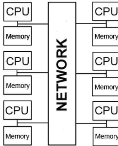
Figure 5.3: Modern supercomputer architecture
