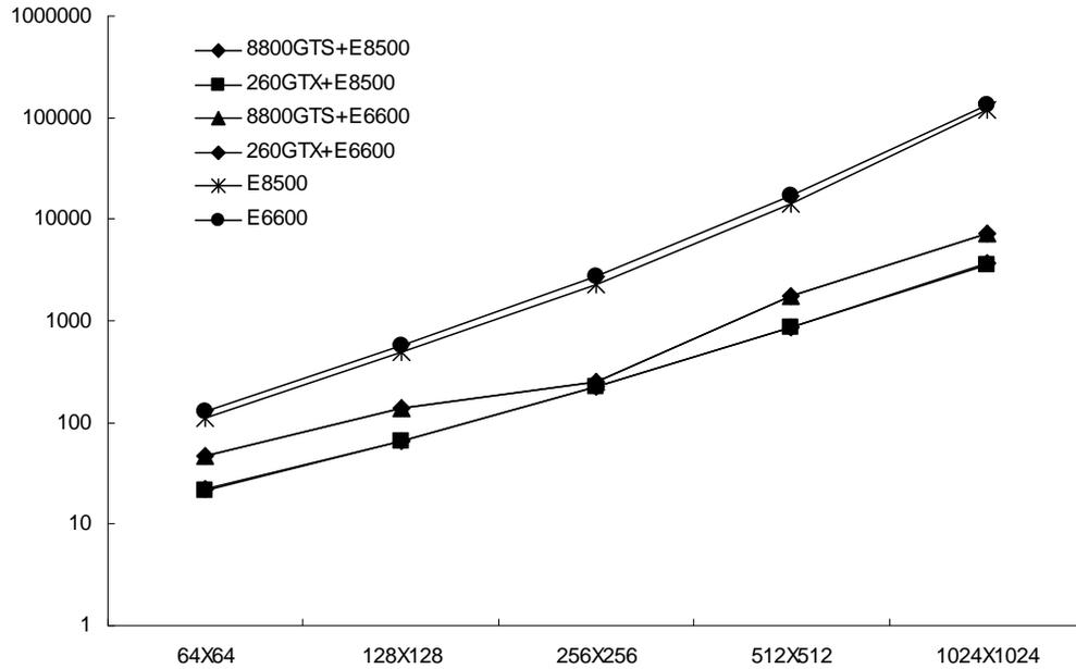
Figure 5.17: Calculation time comparison between GPUs and CPUs
