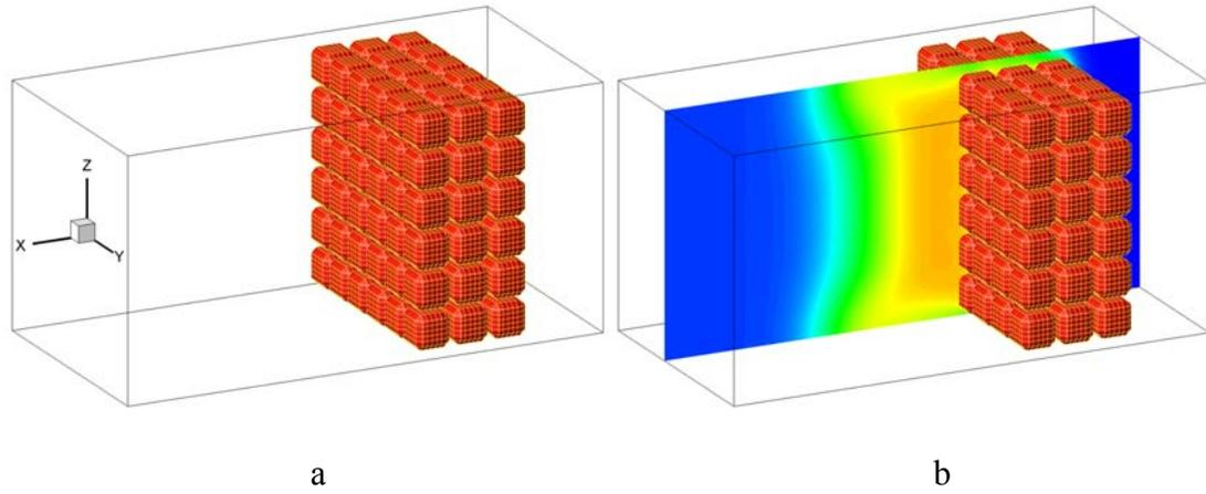
Figure 5.22: (a) Demonstration of simulation domain, (b) Temperature contour on a slice at  $y=25$
