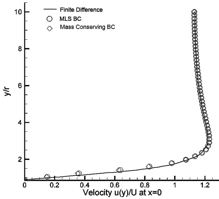
Figure 3.6: Comparison of the velocity profiles at  $x=0$  for the MLS BC, mass conserving BC and finite difference result for  $Re=10$
