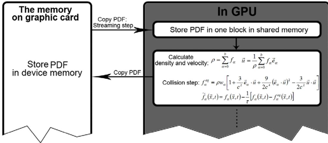
Figure 5.12: Demonstration of the streaming step and collision step based on the CUDA
