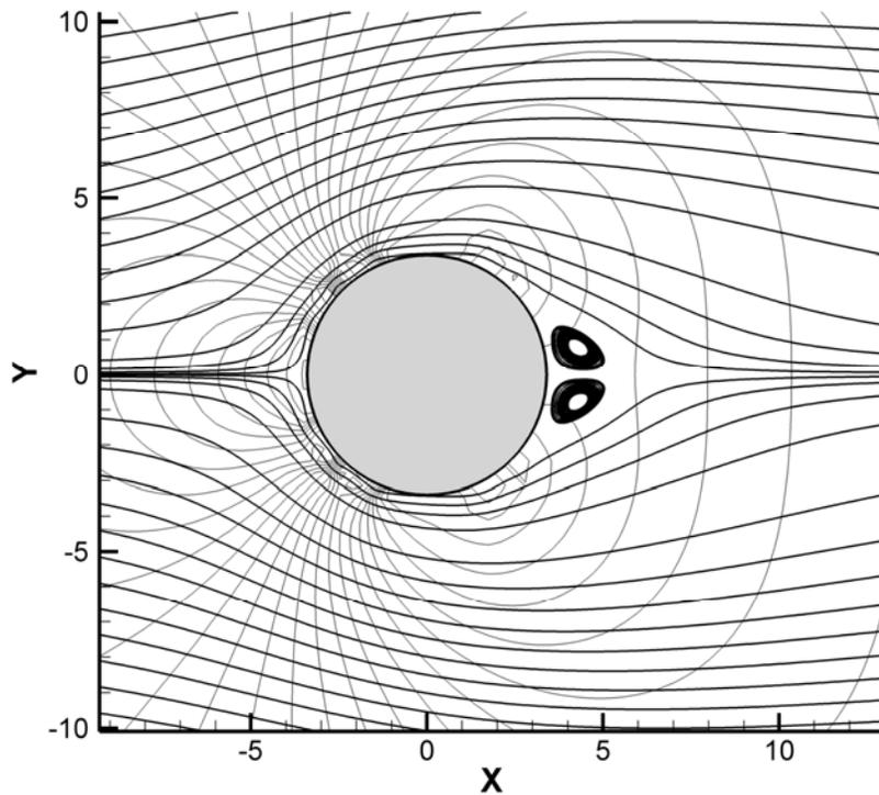
Figure 3.5: Steady flow around a cylinder at  $Re=10$ , with streamlines and pressure contours
