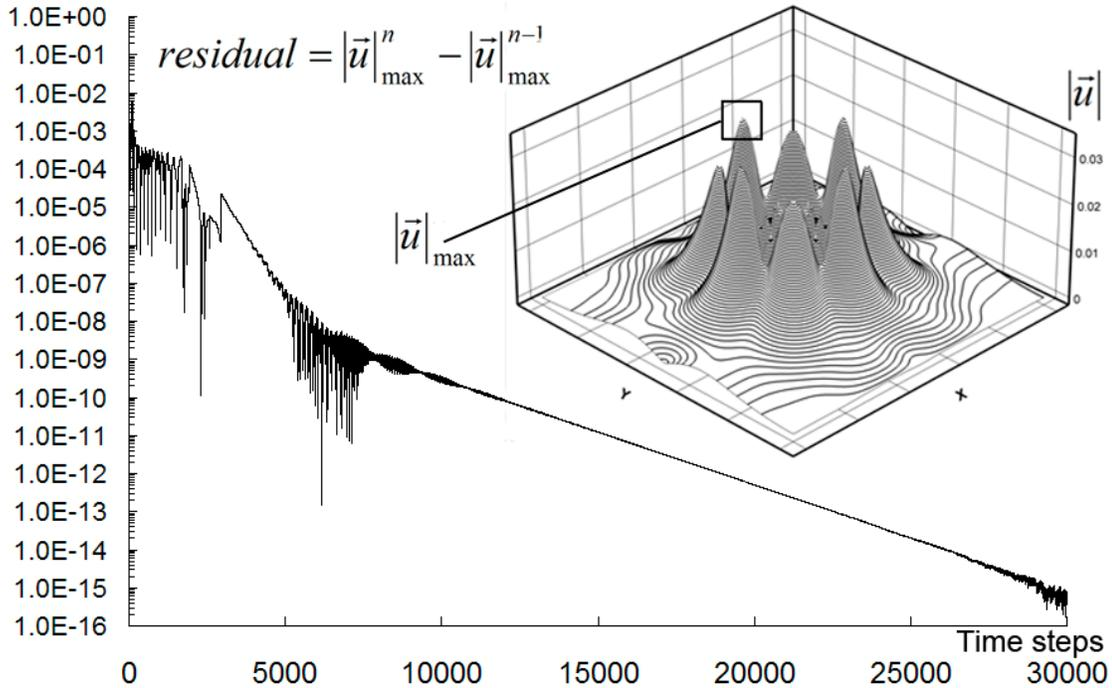
Figure 4.7: The residual changes with time steps
