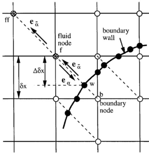
Figure 2.3: Layout of the lattice and curved wall boundary
