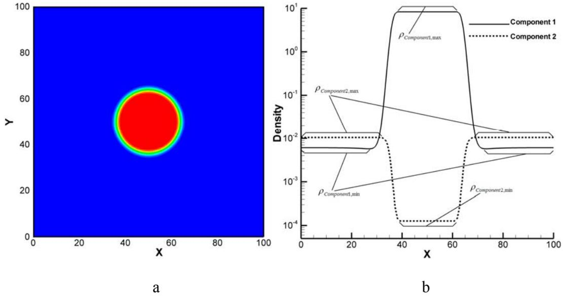
Figure 4.1: (a) Density contour for a circular droplet, (b) Comparison of the densities of the two components along the center line ( $y = 50, 0 \leq x \leq 100$ )
