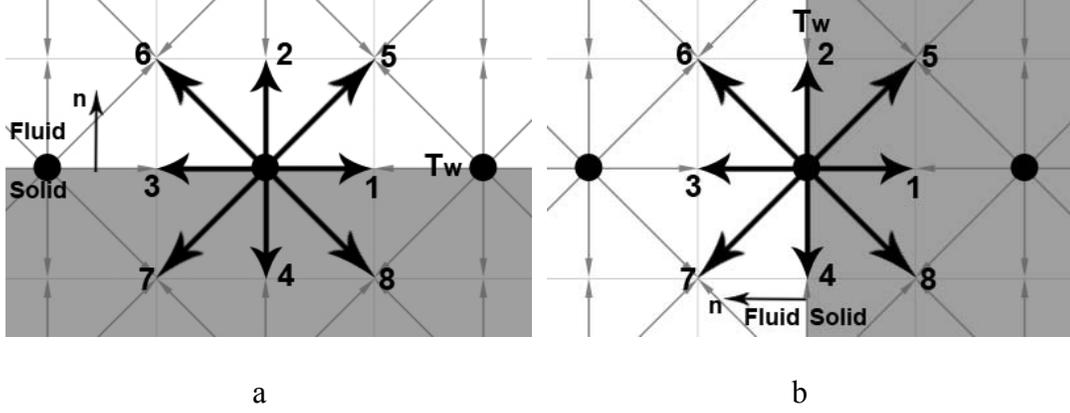
Figure 2.7: Sketch of thermal boundary condition for D2Q9
