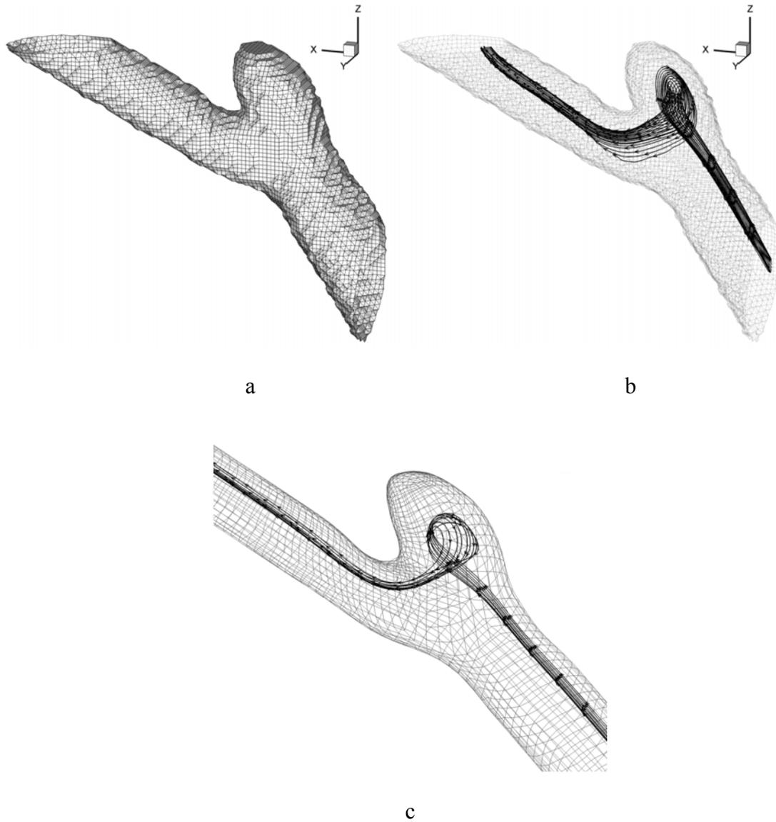
Figure 5.21: (a) Simulation domain for flow in vessel networks, (b) streamline in blood vessel from the LBE model, (c) streamline in blood vessel from a finite element analysis method
