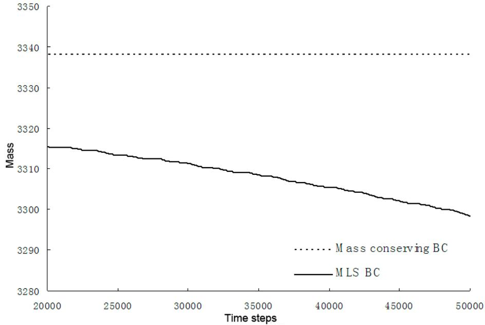
Figure 3.3: System mass change with time using the mass conserving BC and MLS BC
