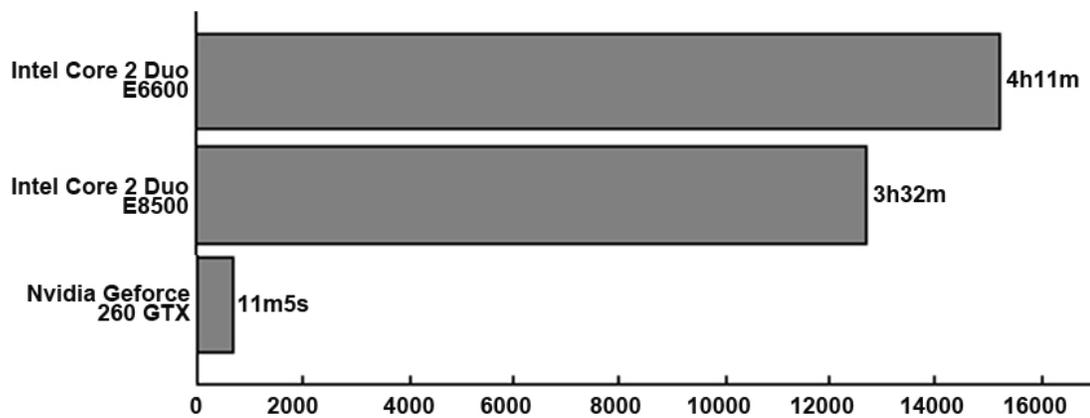
Figure 5.20: Calculation time comparison for 3-D porous media flow
