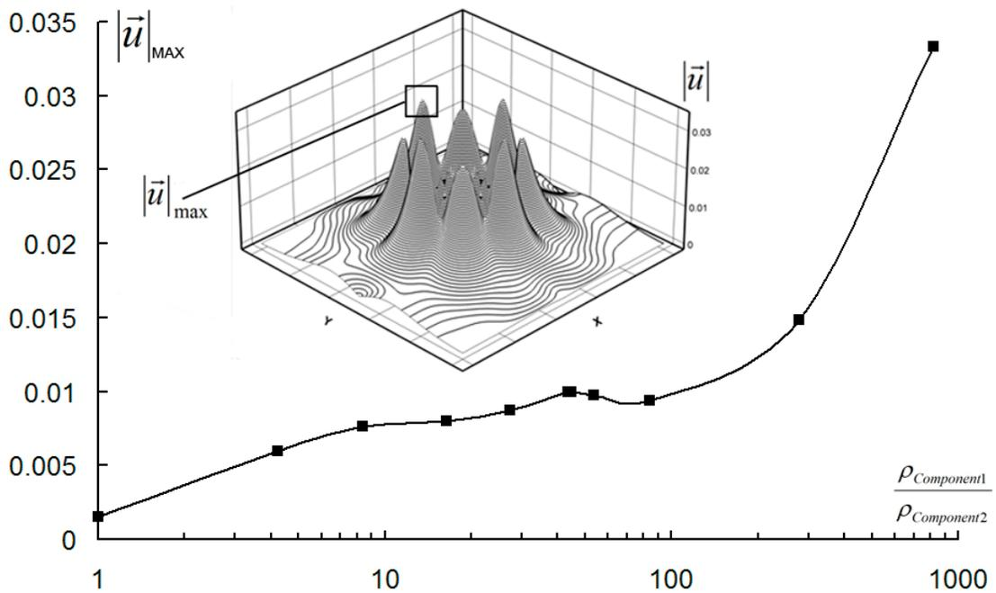
Figure 4.6: The maximum magnitude of the spurious currents varying with the density ratio
