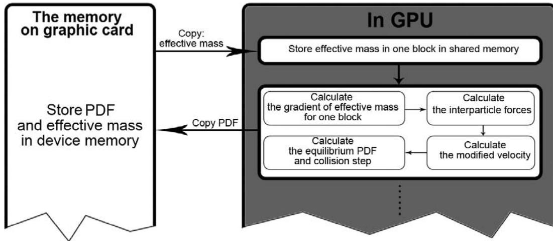
Figure 5.14: Demonstration of MCMP LBE model based on CUDA programming
