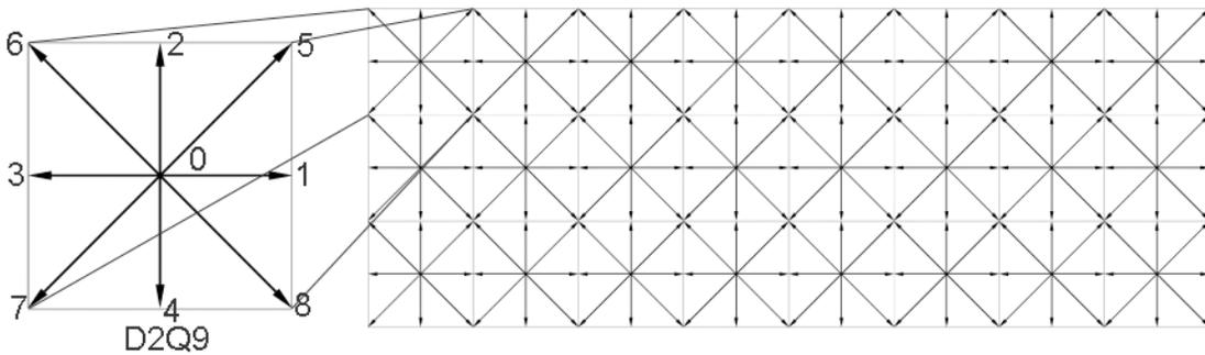
Figure 1.1: The 2D grids for LBM
