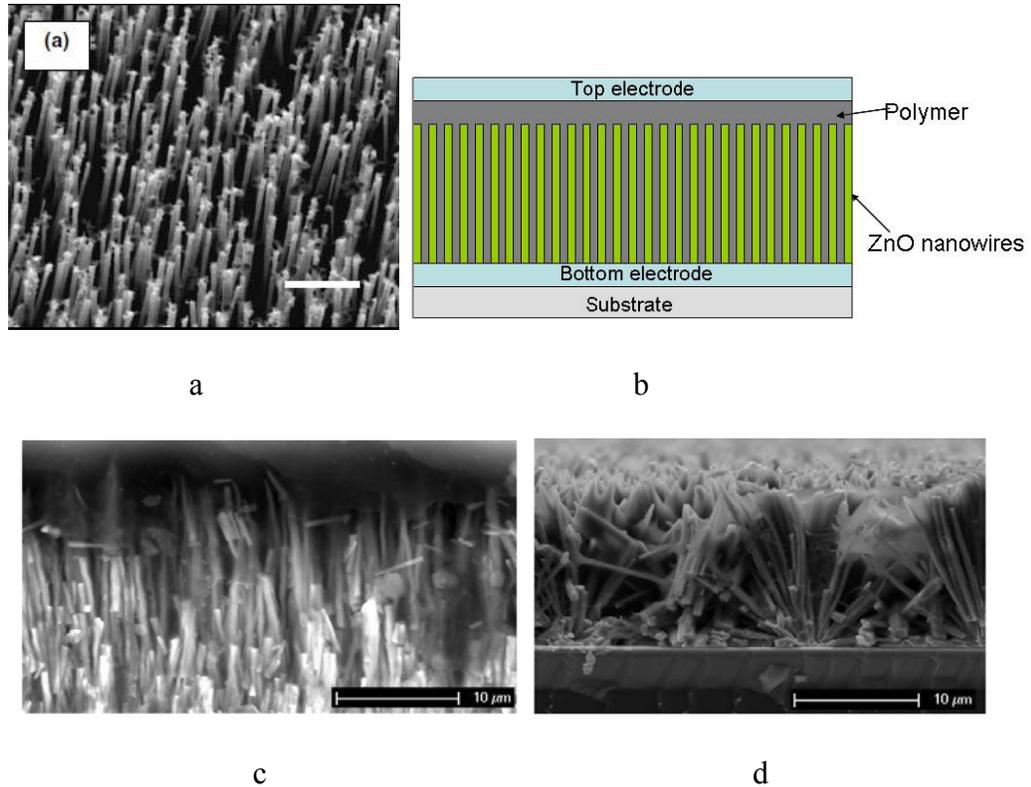
Figure 5.31: (a) SEM image of nanowire array, (b) schematic diagram of ideal ZnO nanocomposite, (c)(d) SEM image of ZnO nanocomposites
