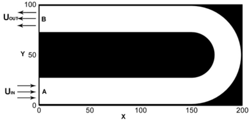
Figure 3.1: Schematic computational area for flow in a curved pipe
