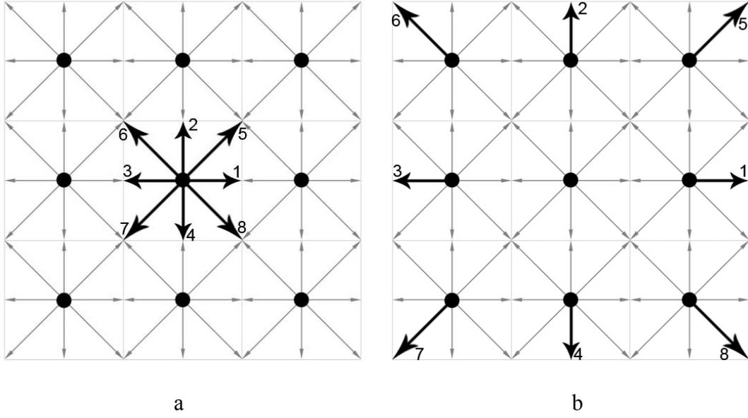
Figure 5.11: Streaming step: (a) time step 0; (b) time step 1
