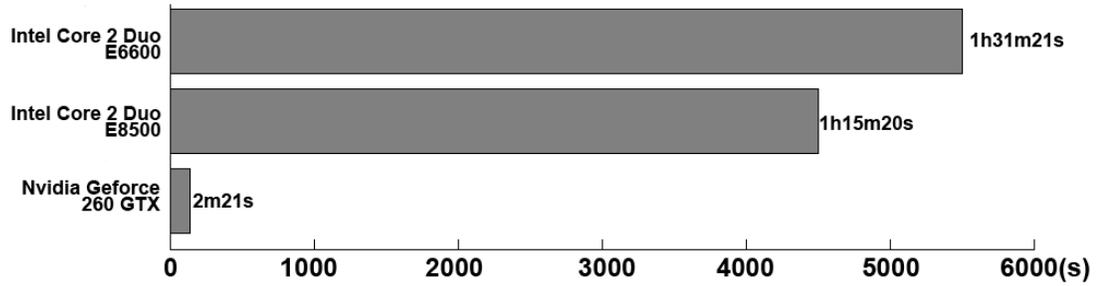
Figure 5.24: Calculation time comparison for 3-D thermal porous media flow
