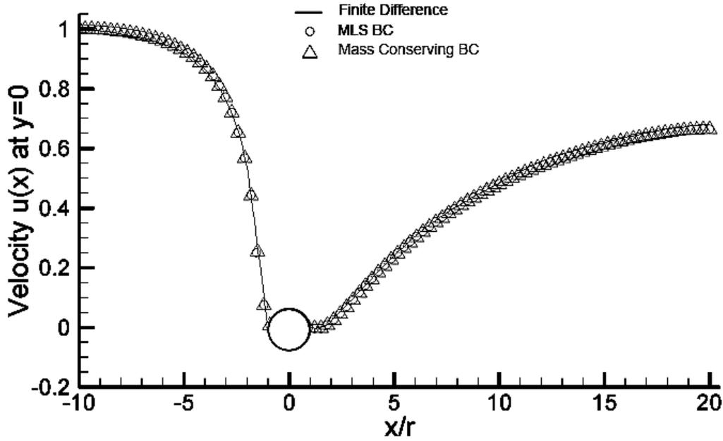
Figure 3.7: Comparison of the velocity variation at the centerline ( $y=0$ ) for the MLS BC, mass conserving BC and finite difference result for  $Re=10$
