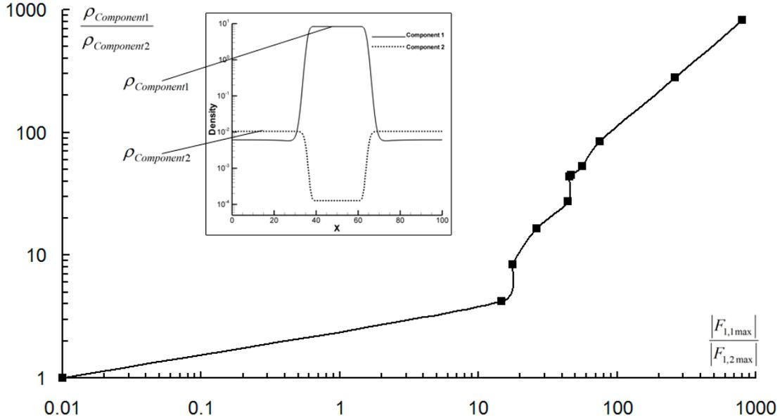
Figure 4.4: Density ratio  $\frac{\rho_{Component1}}{\rho_{Component2}}$  variation with the ratio of the maximum force  $\frac{|F_{1,1max}|}{|F_{1,2max}|}$
