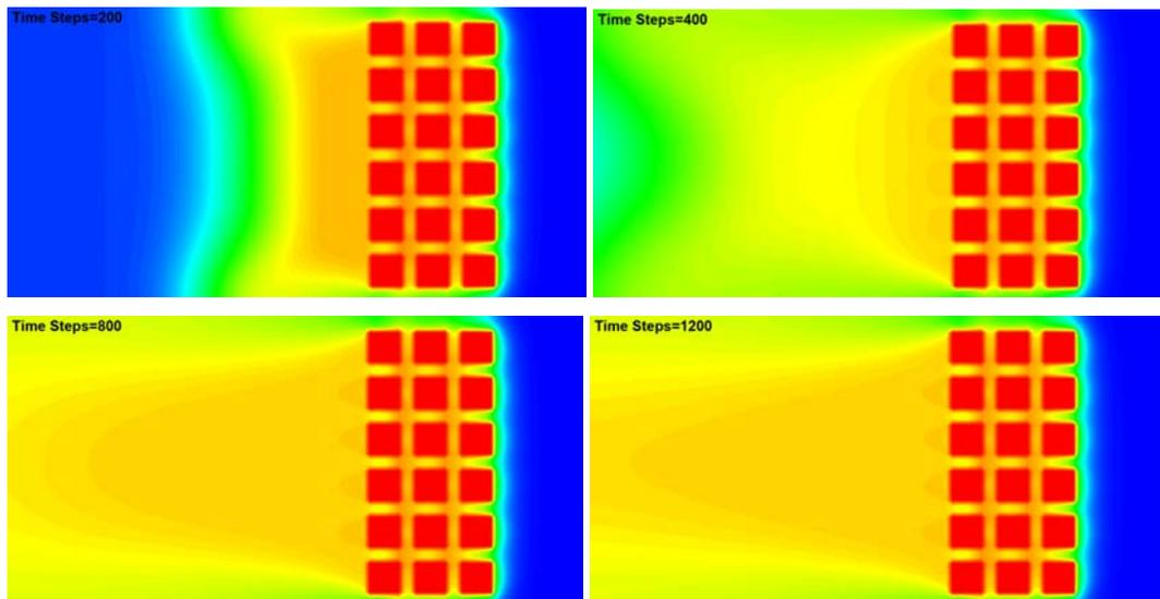
Figure 5.23: Temperature contour at the slice of  $y=20$  for time steps 200, 400, 800 and 1200
