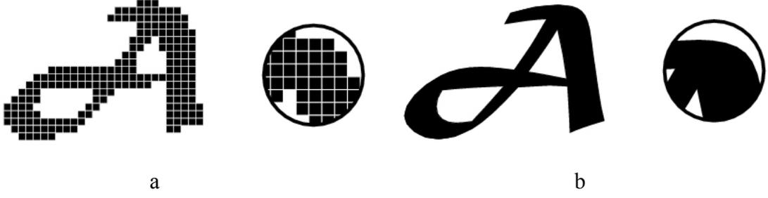
Figure 2.2: Demonstration of 2-D LBE grids, (a) low resolution, (b) high resolution
