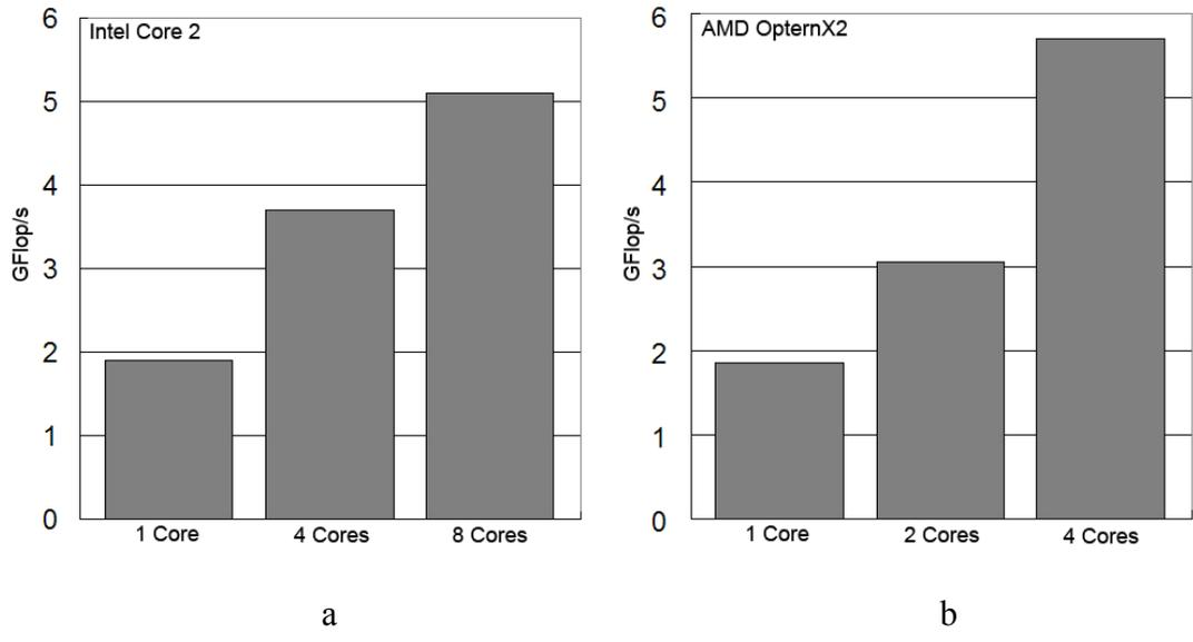
Figure 5.1: Comparison of runtime performance for a different number of cores on a 64X64X64 LBE problem<sup>38</sup> for the (a) Intel Core 2 and (b) AMD OpteronX2
