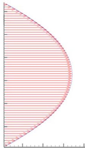
Figure 5.16: Comparison of velocity profile from CUDA LBE model (red vectors) and analytical solution (blue line)
