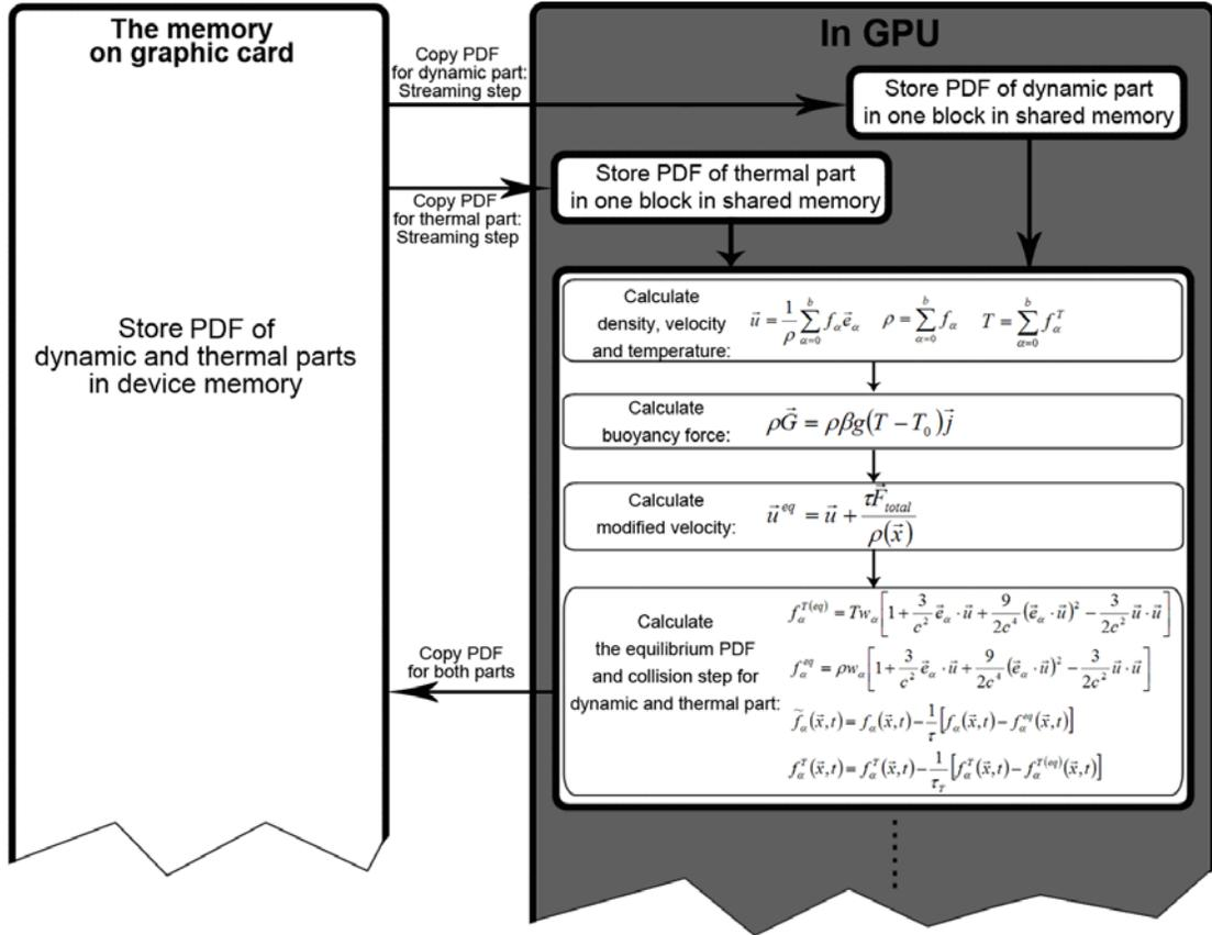
Figure 5.15: Demonstration of the Thermal LBE model based on CUDA programming
