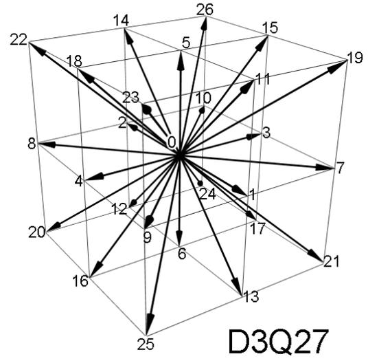
Figure 1.2: 2D square lattice and 3D cubic lattice for LBM
