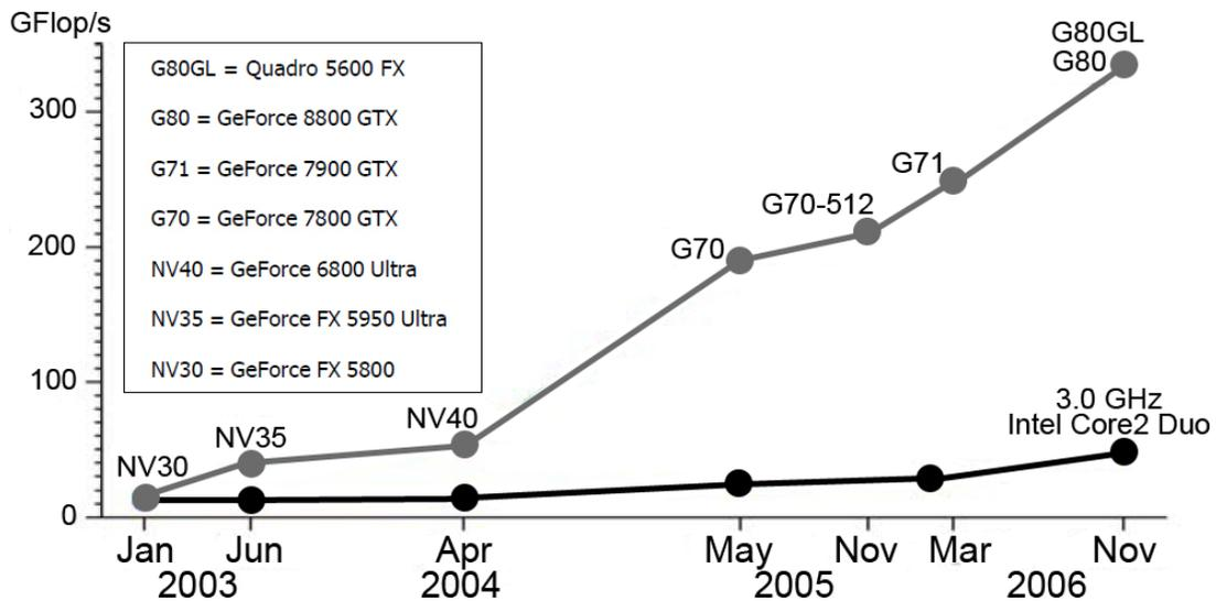
Figure 5.4: Comparison of floating-point operation capacity between GPUs and CPUs
