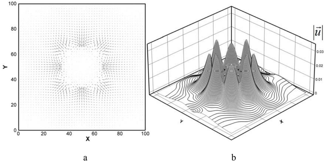
Figure 4.5: (a) Vector of spurious current around the droplet, (b) magnitude of the spurious current
