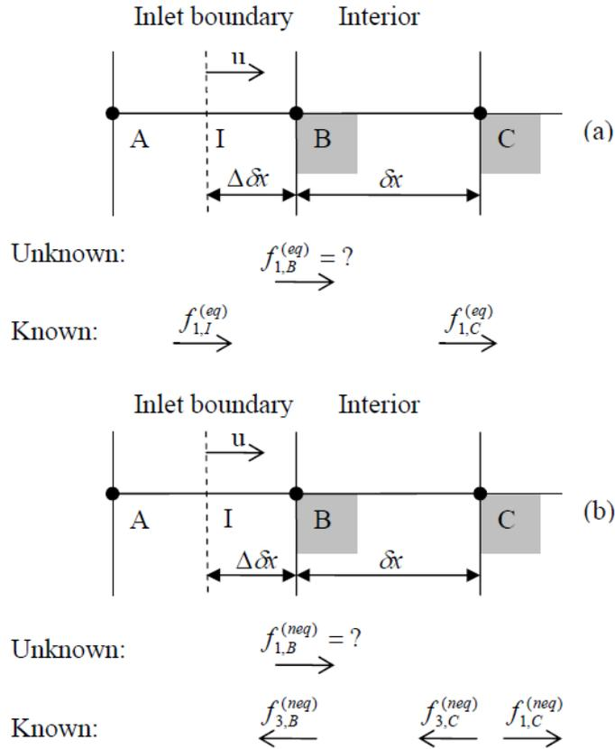
Figure 2.6: Configuration of PDFs used to construct the inlet boundary condition: (a) Configuration of equilibrium PDFs at the inlet, (b) Configuration of non-equilibrium PDFs at the inlet (the gray color denotes a fluid node)
