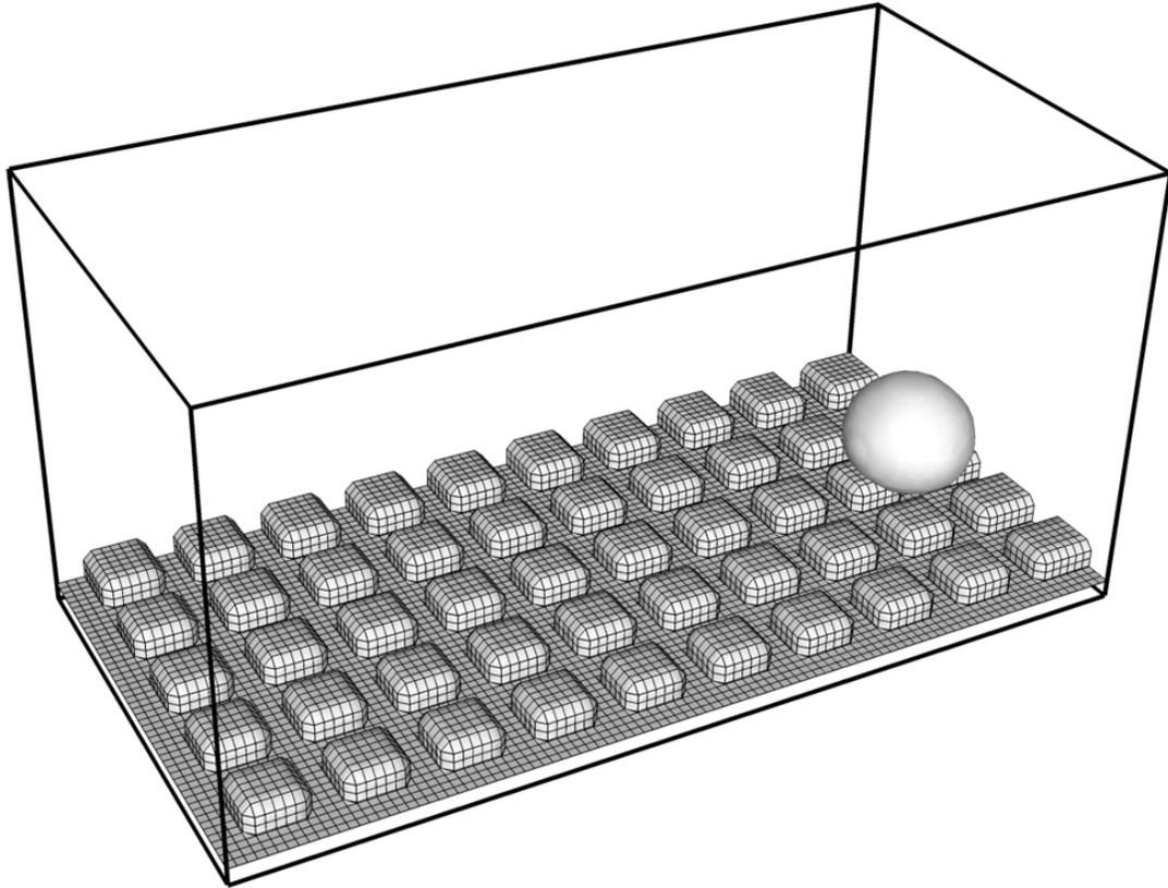
Figure 5.25: A droplet on a micro-structured solid surface
