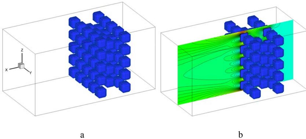
Figure 5.19: (a) Demonstration of simulation domain, (b) Velocity profile on a slice at  $y=25$
