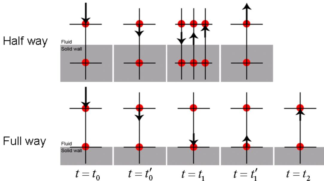
Figure 2.1: Demonstration of half way and full way bounce back boundary condition
