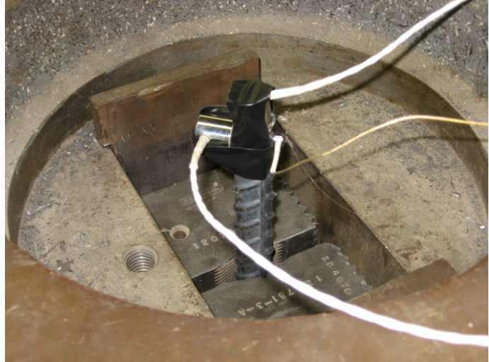
(b) AE sensor arrangement on top of rebar
