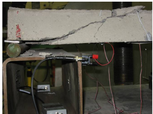
(b) shear failure of Specimen 4x2.
