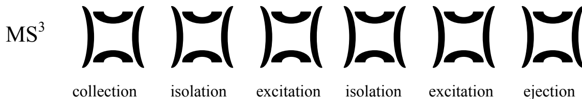
Figure 1.8 The scheme of a MS 3 experiment in ion trap. The experiment is initiated by the collection of the ion current, followed by the isolation of the parent ion, excitation of the parent ion, isolation of the fragment ion, excitation of the fragment ion and the ejection of the secondary fragment ions generated by the secondary excitation.
