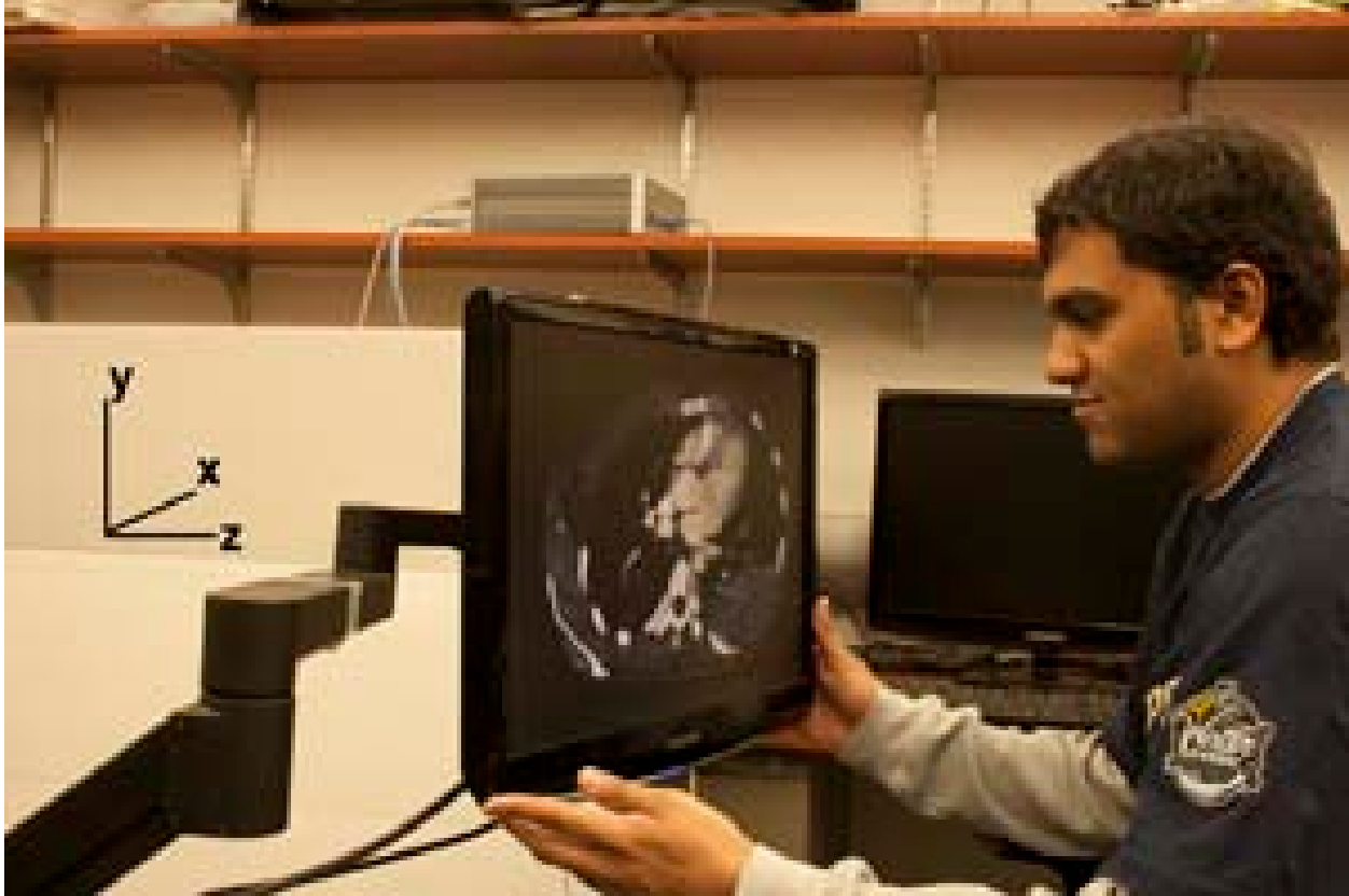
Figure 3.3: User operating the grab-a-slice display, which can be manipulated freely in six degrees of freedom.
