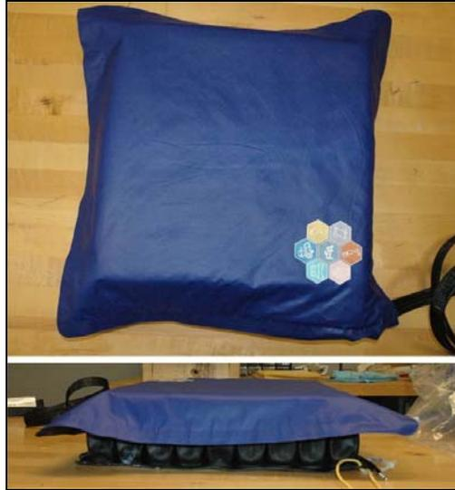
**Figure 23: FSA pressure mat system.**
