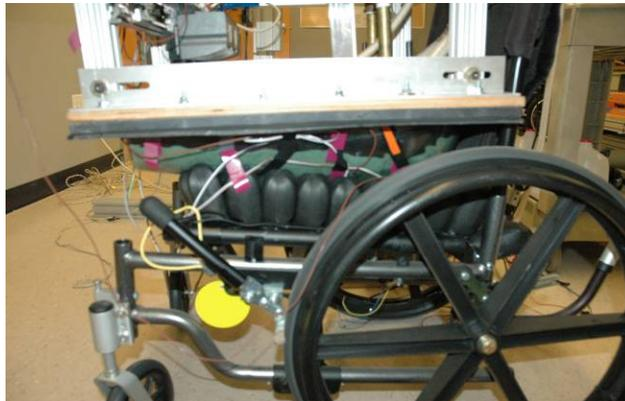
**Figure 27: TRCLI resting on calibrated ROHO cushion**
