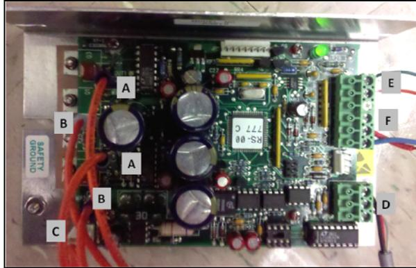
Figure 11: TEC controller board with two power supplies (A)(B) and dual input thermistors (E)(F).
