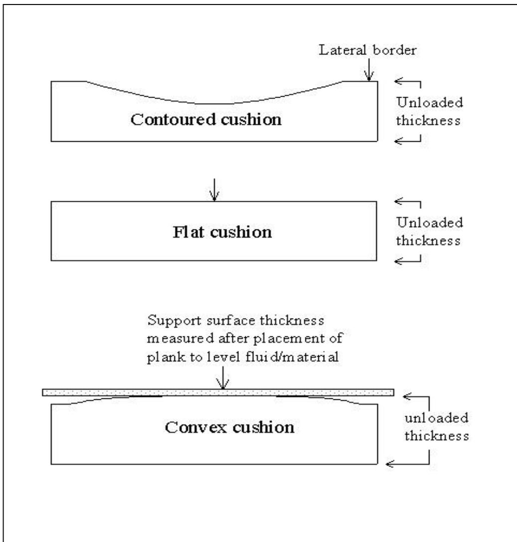
FIGURE 13: Measurement method for concave and convex seat cushion[40]
