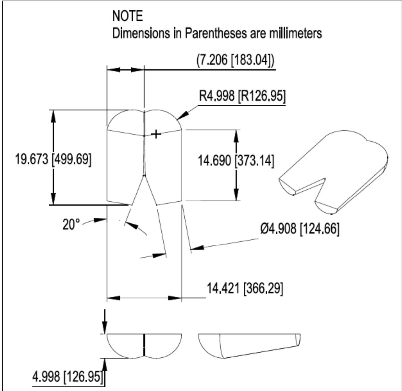
FIGURE 1: 2-D drawing of the modified Staarink indenter (RCLI) [40]
