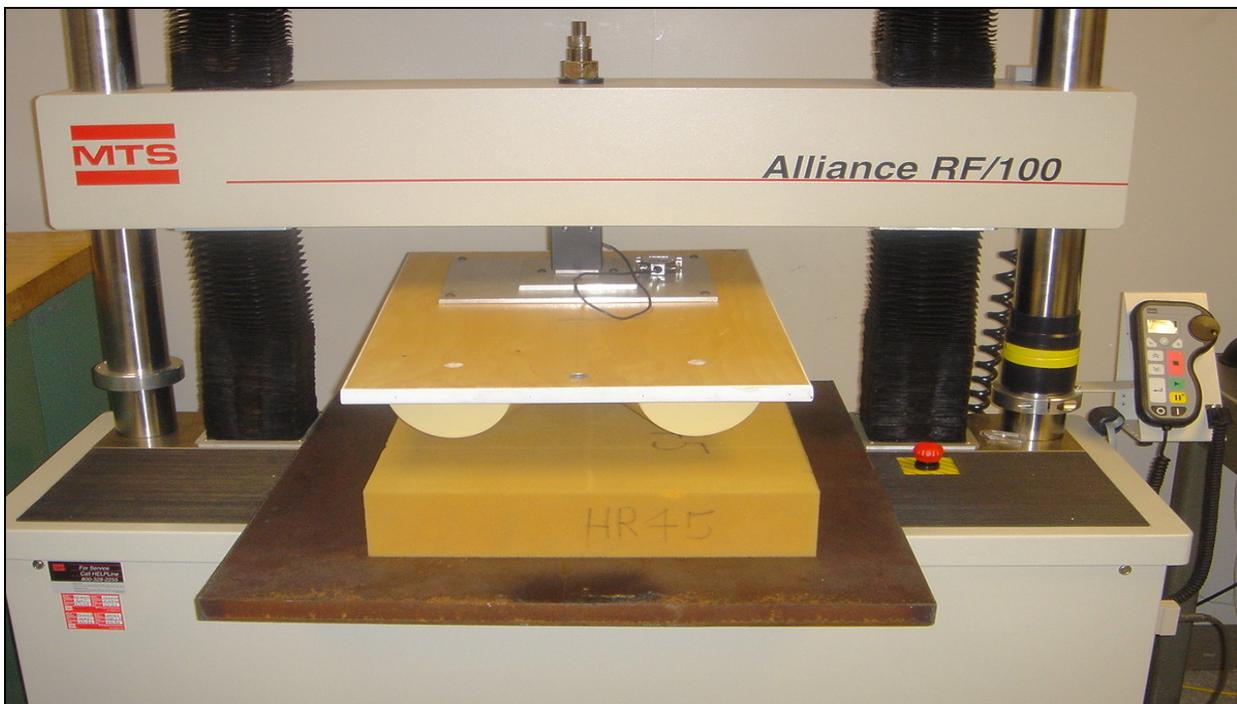
FIGURE C1: Set Up for Load-Deflection
