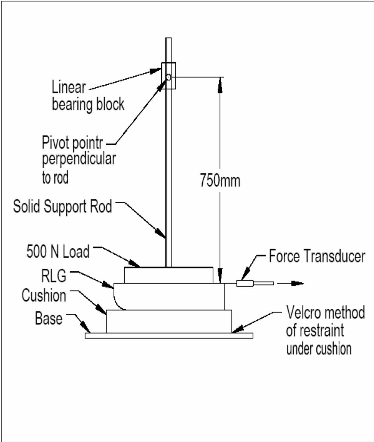
FIGURE 10: Apparatus to measure Lateral and Forward Stiffness[40]
