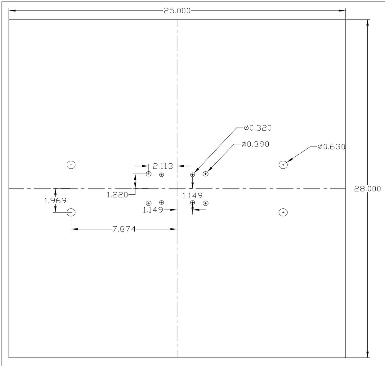
FIGURE B1: MTS Base Plate (in inches)
