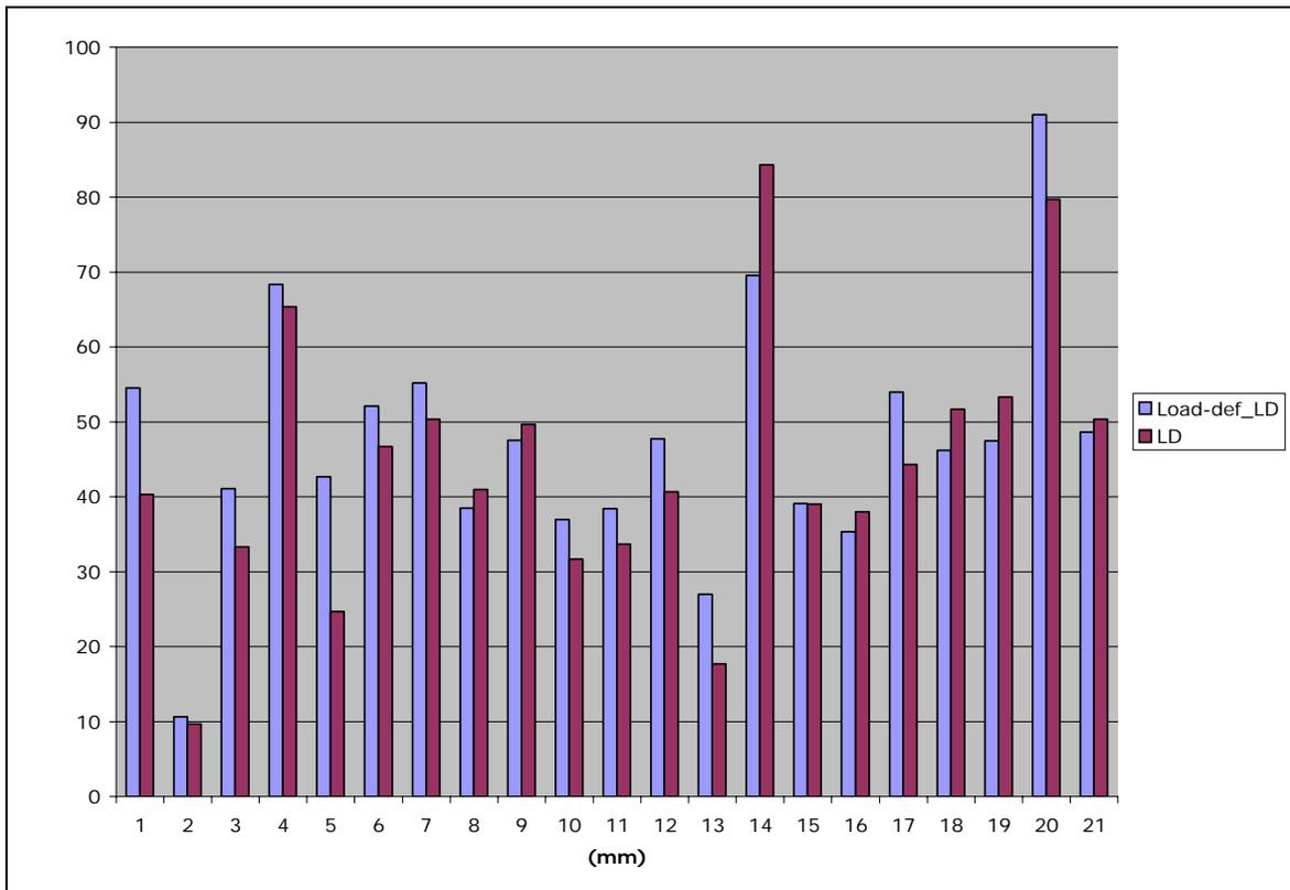
FIGURE 15: Comparison between Load-def loaded depth at 500N and LD
