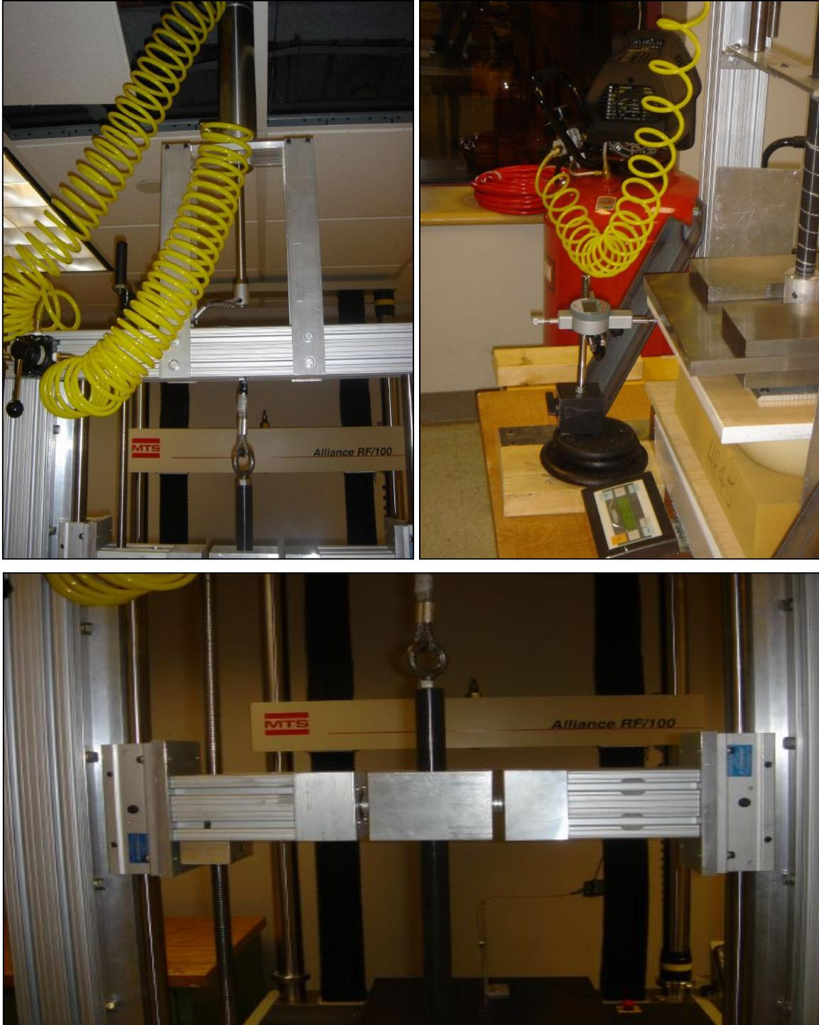
FIGURE D2: (i) Cylinder assembly (ii) Displacement & Force Gauge assembly (iii) Linear Bearing assembly
