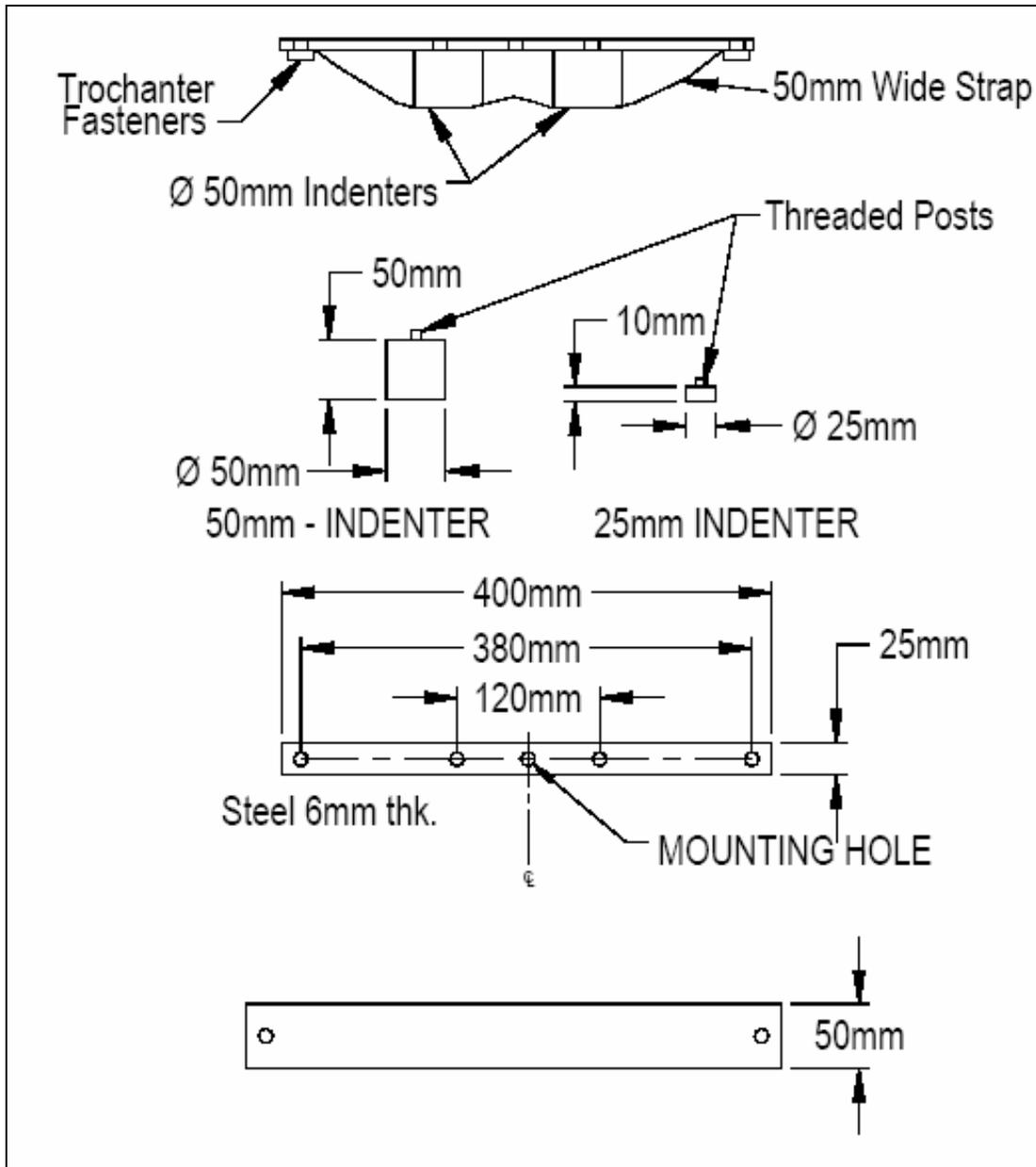
FIGURE 12: Details of the Contour Loading Jig[40]
