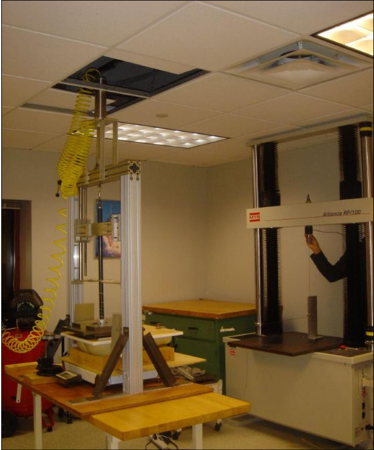
FIGURE D1: Set Up for Lateral and Forward Stiffness
