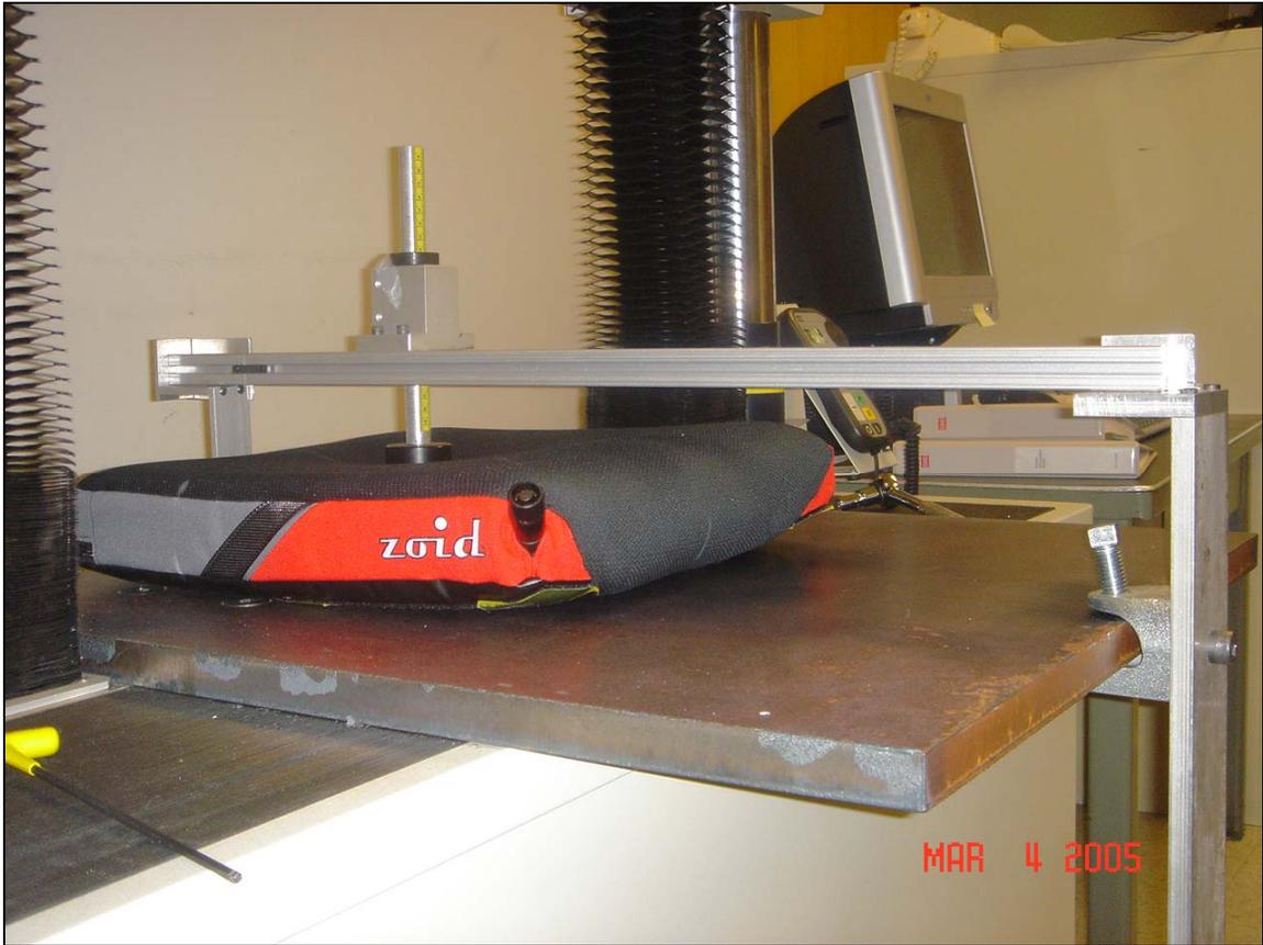
FIGURE B4: Circular Loading Rig (Automated Set-up)
