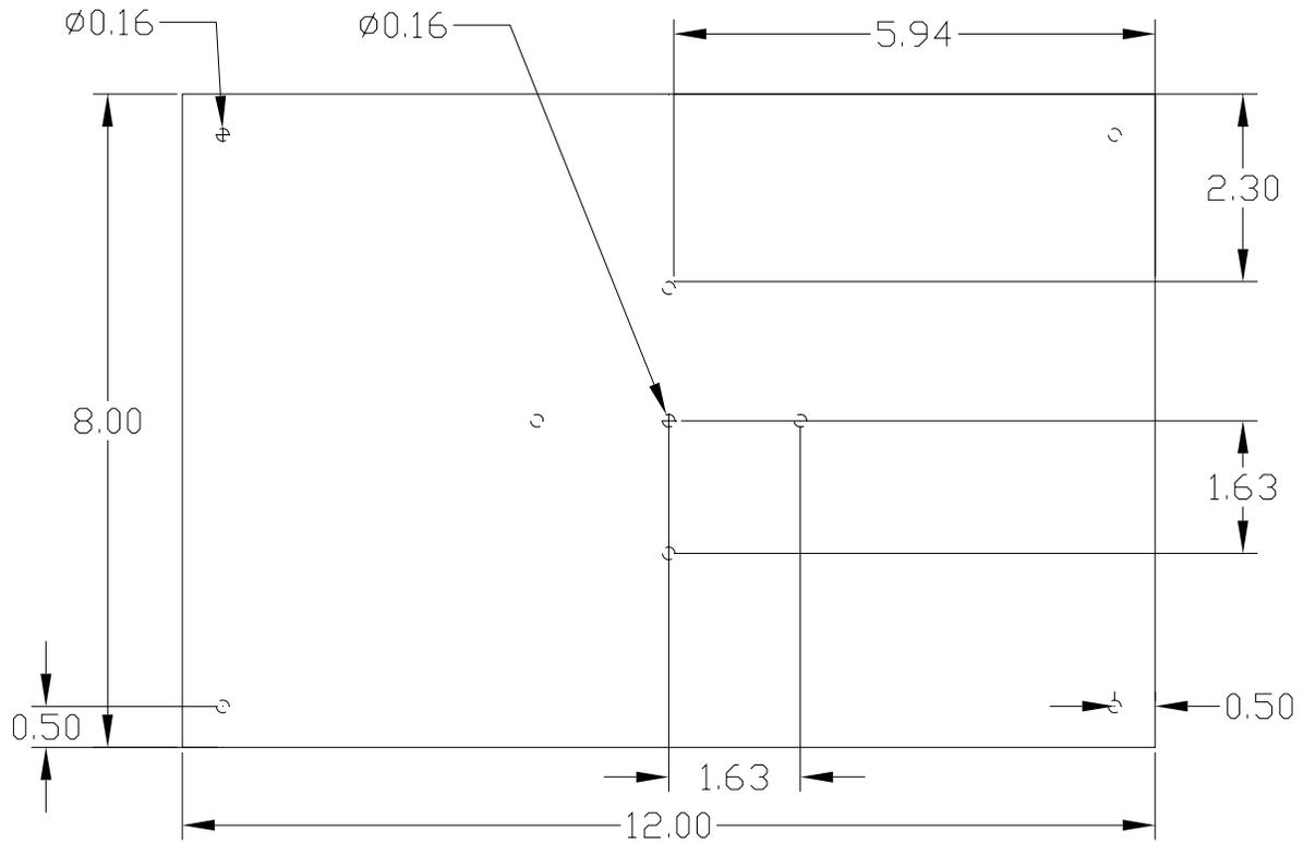
FIGURE B2: MTS-RCLI Adapter (in inches)
