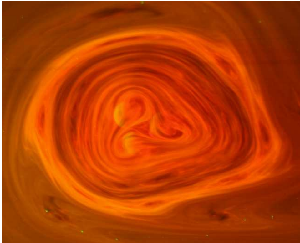
Figure 21: Complex inner structure of toroidal flow just after injection of Rhodamin B fluorescent dye dissolved in glycerin.
