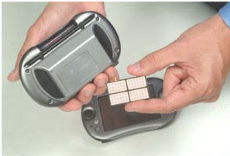
Figure 4 Intermac's newest RFID handheld reader using Mobion™ fuel cell technology
