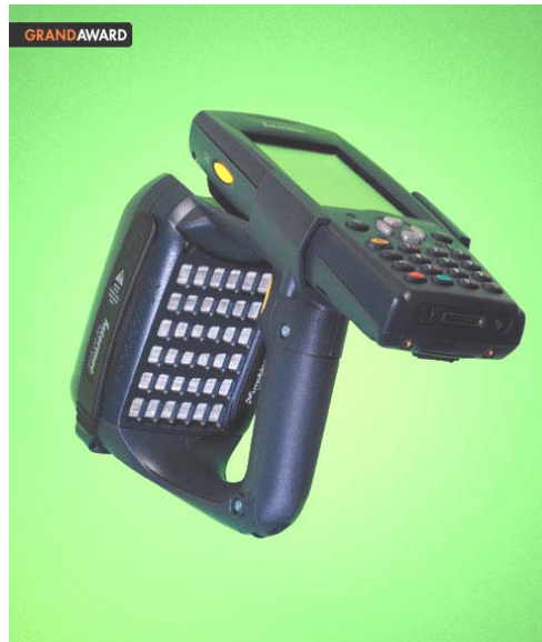
Figure 4 Intermac's newest RFID handheld reader using Mobion™ fuel cell technology
