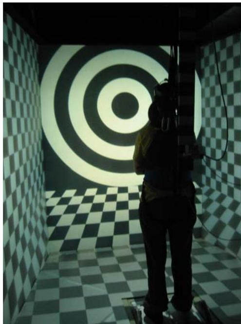
**Figure 2 Subject viewing a bullseye-and-checkerboard pattern in the BNAVE virtual environment. Sway responses were recorded via a single force plate beneath the feet, and an electromagnetic tracking device located at the head. Subject is secured to the support structure by a safety harness.**
