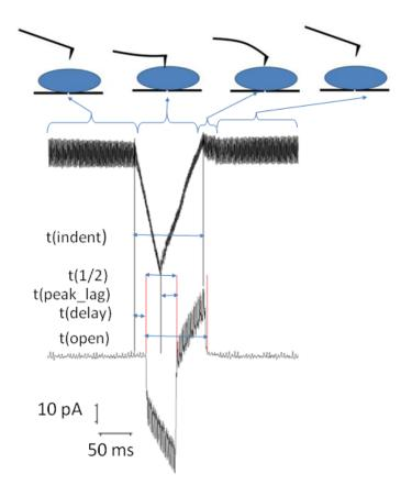
Figure 5.2. Cantilever indenting a voltage clamped cell. Cartoon depiction (top) of various stages of the indentation process as manifested in voltage output from the photodiode (upper trace) and the corresponding whole-cell current in response to an indentation (lower trace). Kinetic parameters pertaining to the process are indicated.
