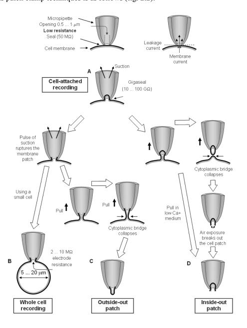
Figure 2.2. Patch clamp configurations. (a) intact-cell configurations include the "cell-attached", the "whole-cell", and the "perforated patch" (b) excised patch configurations include the "inside-out" and the "outside-out" (http://www.bem.fi/book/04/04x/0427x.htm)
