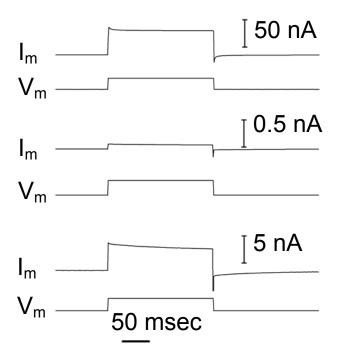
Figure 4.4. Current  $(I_m)$  responses to a 100 mV voltage step  $(V_m)$  for: (top) an open pore, (middle) cell plasma membrane forming giga-ohm seal, and (bottom) a whole-cell patch clamp of a CHO cell.
