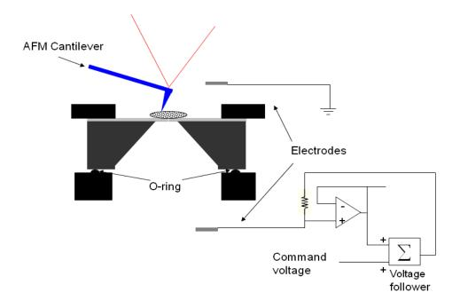
Figure 5.1. Schematic of the planar patch clamp assembly integrated with an AFM.
