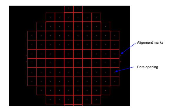
Figure 3.2. AutoCAD snapshot of a sample mask to be used for the back-side photo-lithography step. This defines the 1cm X 1cm array of individual devices (red squares). The small red dots represent the 700  $\mu$ m square windows for the back-side etching. A 4-inch wafer yields about 92 patch-clamp chips.
