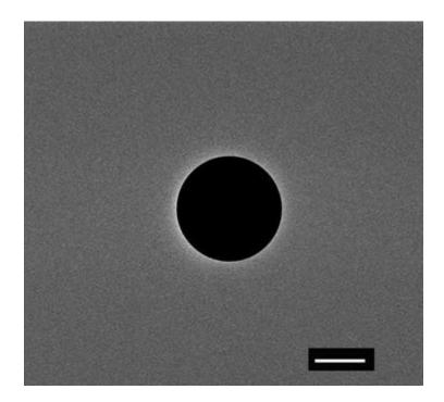
Figure 4.1. Scanning electron micrograph of the pore in a sample, representative chip. The scale bar at the bottom is 0.5  $\mu m$ .
