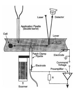
Figure 2.5. Schematic of the apparatus used for obtaining AFM images of excised membrane patches spanning the opening of a glass pipette (Horber, Mosbacher et al. 1995).
