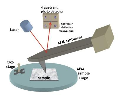
Figure 2.4. Atomic force microscope setup: The deflection of the cantilever is measured by reflecting a laser beam from the top side of the cantilever while it is scanning over the surface of the sample mounted on a piezo-activated XYZ stage. (Source: Opensource Handbook of Nanoscience and Nanotechnology)
