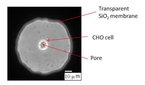
Figure 4.2. A phase contrast optical microscopy image of a CHO cell sitting over the central pore on the circular  $SiO_2$  membrane window. The dark, opaque portion surrounding the membrane is the silicon as seen from the bottom of the chip.
