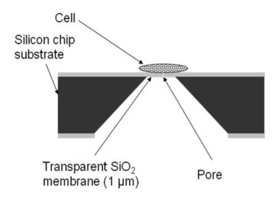
Figure 3.1. Cross-section of the planar patch clamp chip design
