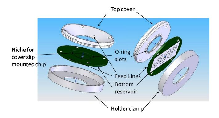
Figure 3.4. Design of the liquid cell.
