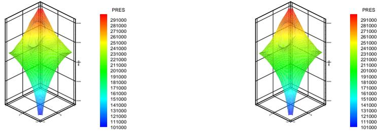
Figure 61: 3D view of pressure contours at 350 days for heterogeneous benchmark problem:  $(r_{p_1}, r_{s_1}) = (4, 2), (r_{p_2}, r_{s_2}) = (3, 1)$  (left) and  $(r_{p_1}, r_{s_1}) = (5, 3), (r_{p_2}, r_{s_2}) = (3, 1)$  (right).
