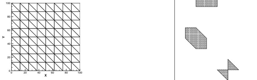
Figure 47: Uniform triangular mesh (left) and permeability field (right):  $k = 5 \times 10^{-13}m^2$  in dark regions and  $k = 5 \times 10^{-9}m^2$  in rest of domain.
