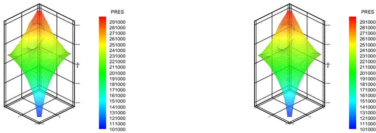
Figure 64: 3D view of pressure contours at 350 days for heterogeneous benchmark problem:  $(r_p, r_s) = (4, 2)$  (left) and  $(r_p, r_s) = (5, 3)$  (right).
