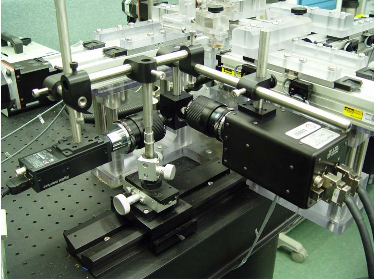
**Figure 29. The dual biaxial testing device dual camera system.**
