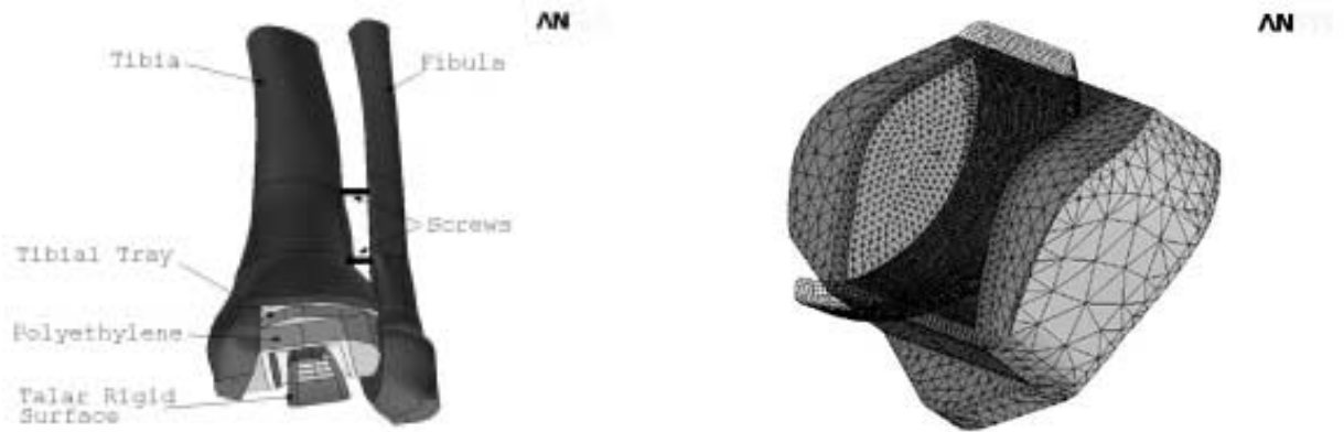
Figure 6.1 Full solid model (right) and FEM submodel (left) for calculating stresses in the UHMWPE insert
