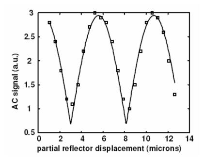
**Figure 2-2** The dependence of the near-field signal on displacement of the partial reflector. Squares represent the data points; solid line represents the fit, whose functional form is the absolute value of cosine of the displacement.
