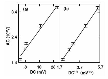
**Figure 2-3** The amplitude of scattered near-field signal at  $2\Omega$  vs. (a) the amplitude of dc component, (b) the square root of the amplitude of dc component. Solid lines represent a linear fit to the data points.
