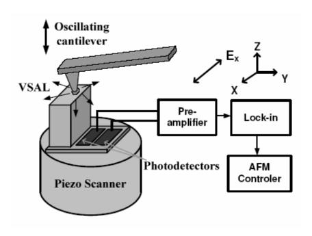
Figure 4-1 Geometric relations of the apertureless NSOM components for the imaging of VSAL.
