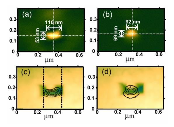
**Figure 5-4** Observation of optical field confinement in the ridge waveguide: (a) Near-field image at *If* detection; (b) near-field image at *2f* detection, (c) and (d) are the height images with optical intensity contours for *If* and *2f*. Spot size confinement effect is clearly indicated.
