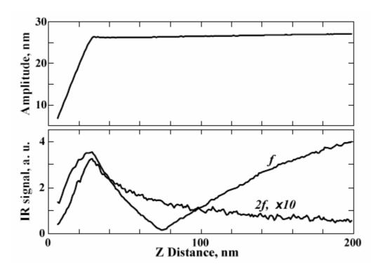
**Figure 3-2** The top panel shows how the amplitude of the vertical probe oscillation depends on the separation from the surface. The bottom panel shows IR signals demodulated at the frequency of the probe oscillation (f) and twice the oscillation frequency (2f). The interferometric feature present in the f-signal is missing from the 2f-signal.
