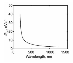
Figure 4-2 Dispersion diagram of surface plasmons generated at Al/Si<sub>3</sub>N<sub>4</sub> surface.
