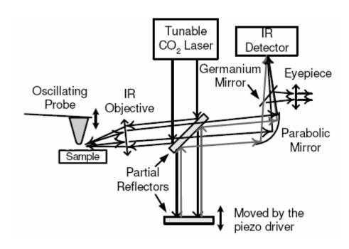
**Figure 2-1** Schematic representation of the apertureless near-field infrared microscope. The back-scattered light,  $E_{sc}$ , is modulated by the oscillating tip. The piezo driver adjusts the relative phase of the homodyning reference field,  $E_r$ , that interferes at the detector with the light back-scattered by the probe. The dominant AC contribution to the homodyned intensity at  $2\langle E_{sc}E_r\rangle$  is detected using a lock-in amplifier.
