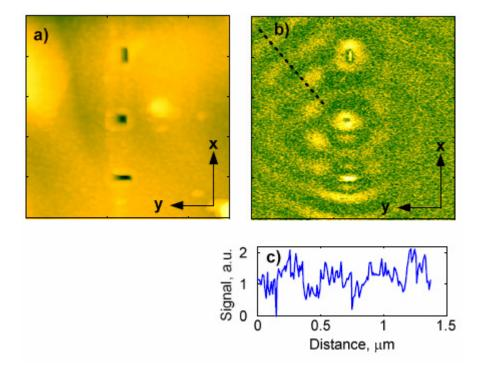
**Figure 4-5** (a) Topographic image of three apertures made on Al coated laser diode. (b) Near-field signal collected in the vicinity of the apertures using integrated photodetectors. Image scan area is 2500 nm x 2500 nm. (c) Section line indicated in (b) by dashed line.
