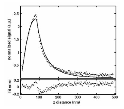
**Figure 2-5** Top panel shows the fit of the one scattering sphere model for the near-field signal. In the model, the sphere oscillates above the surface. The bottom panel shows the fit error.
