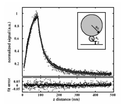
**Figure 2-6** The top panel shows the normalized near-field signal-distance dependence (dots) and curves calculated according to the model described in the text (solid lines). The bottom panel shows the fit error.
