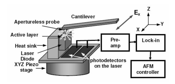
**Figure 5-3** Detailed geometric relations of the apertureless NSOM components for ridge waveguide structure imaging. The structure is fabricated along the active layer.
