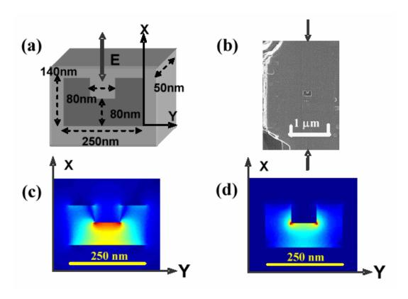
**Figure 5-2** (a) Detailed geometry of a designed ridge waveguide structure, (b) FIB image of such a ridge waveguide fabricated on VSAL (arrow indicating active layer position); (c) and (d) are FDTD simulations of this ridge waveguide showing the  $E_x$  field structure (the dominant component) and total field E distribution at the exit plane of the aperture.
