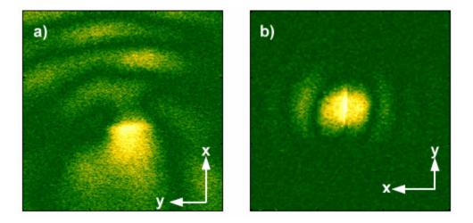
**Figure 4-4** Near-field signals collected in and near the aperture shown in Figure 4-3 using external detector. The aperture was rotated 90 degrees prior to collecting image (b). The external detector was not rotated with the aperture.
