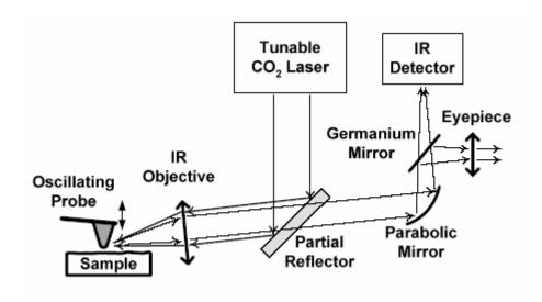
**Figure 3-1** Schematic of the apertureless near-field infrared microscope.
