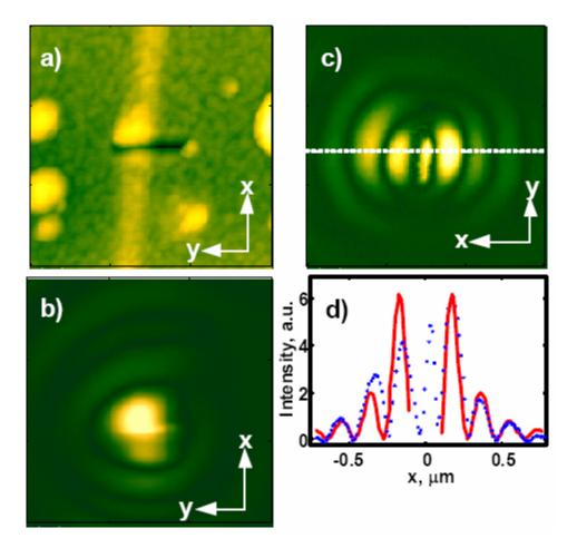
**Figure 4-3** (a) Topographic image of the aperture and its surrounding. The dimensions of the aperture were 400 nm x 100 nm. (b), (c) Near-field signals in and near the aperture. The aperture was rotated 90 degrees prior to collecting image (c). The scan area of the images was 1500 nm x 1500 nm. Plot (d) presents a cross section (dotted line) made in image (c) and a fit (solid line) made according to the surface plasmon point-source model.
