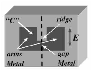
Figure 5-1 A ridge waveguide structure (C aperture) that can have high power throughput.
