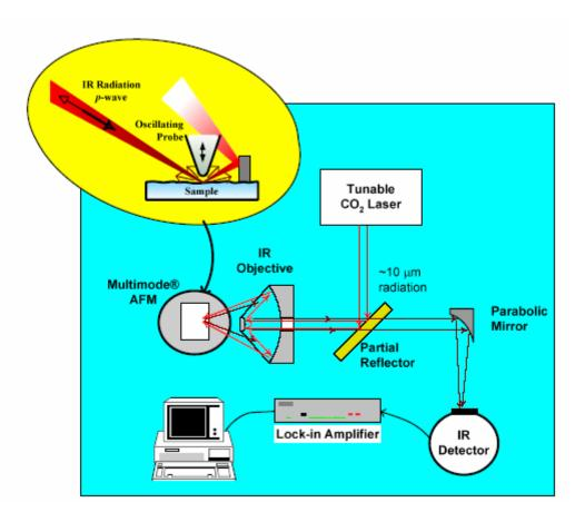
**Figure 1-1** Schematic representation of an apertureless near-field microscope. The laser light is focused onto the end of the probe oscillating near the sample's surface, and the back-scattered radiation from the tip-sample system is focused by means of far-field optics onto the detector's window. Lock-in detection is used to collect the near-field signal at the harmonics of cantilever's oscillation frequency.
