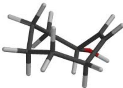
**Figure 1: A Chair-Boat Conformation of 2-Cycloocten-1-ol Using Conformer Distribution, MMFF, Macspartan Pro**
