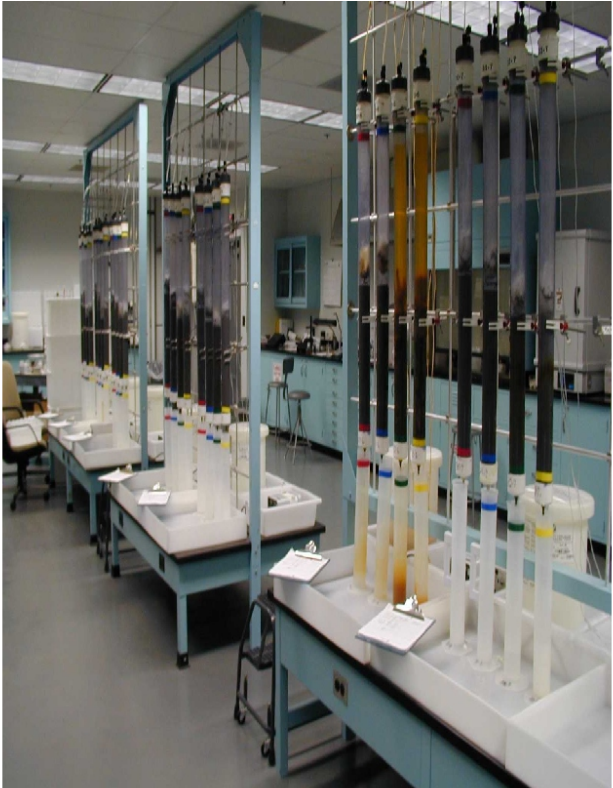
Figure 10. Seven groups of four columns constitute one leaching test.
