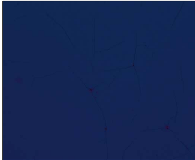
Figure 26. Close Up: Microscopic View of Sputtered PZT Prior to Annealing
