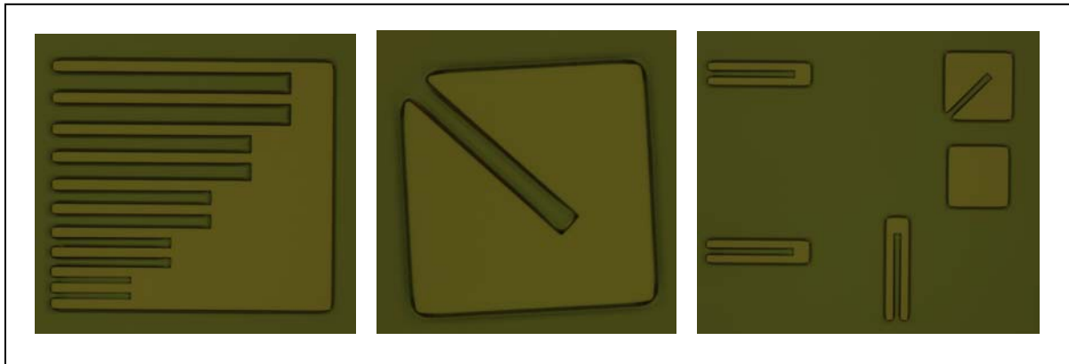
Figure 55. Microscope Images of SiO 2 /SiN x /SiO 2 beams after RIE Etch
