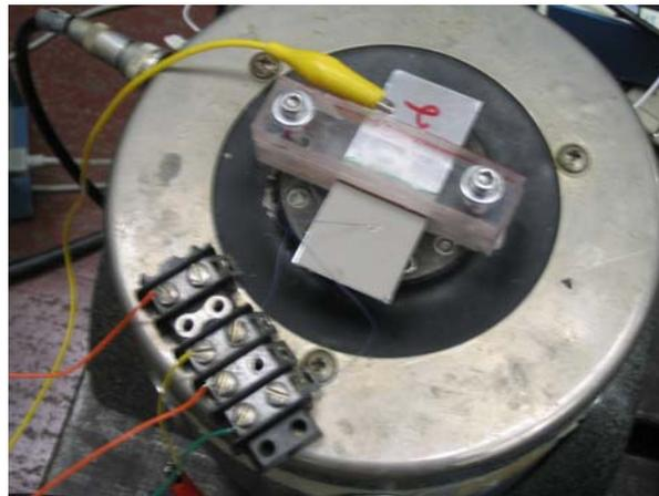
**Figure 6.9.** Bimorph clamped on top of shaker.
