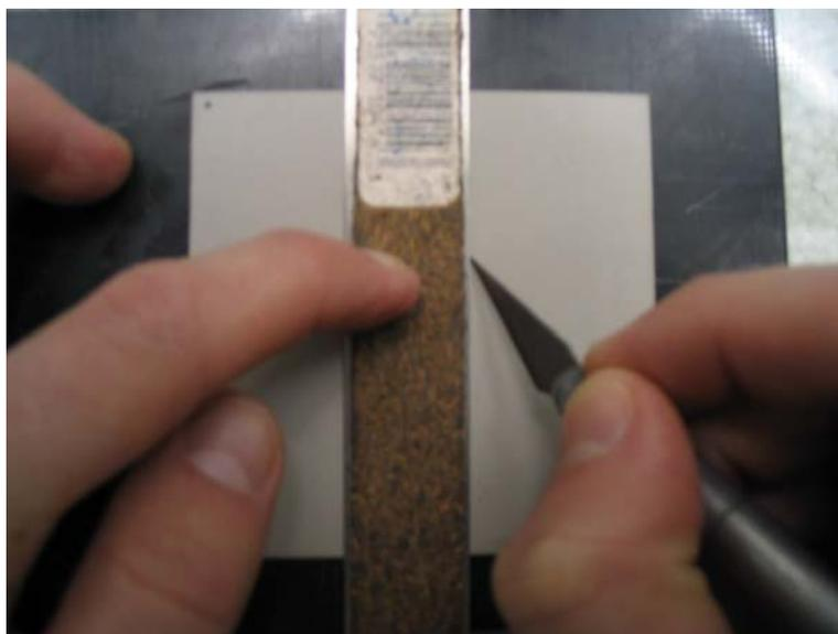
**Figure 6.1.** Scoring a sheet of PZT
