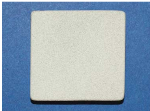
Figure 34. Test sample (ReneN5, MCrAlY, APS YSZ by NETL).
