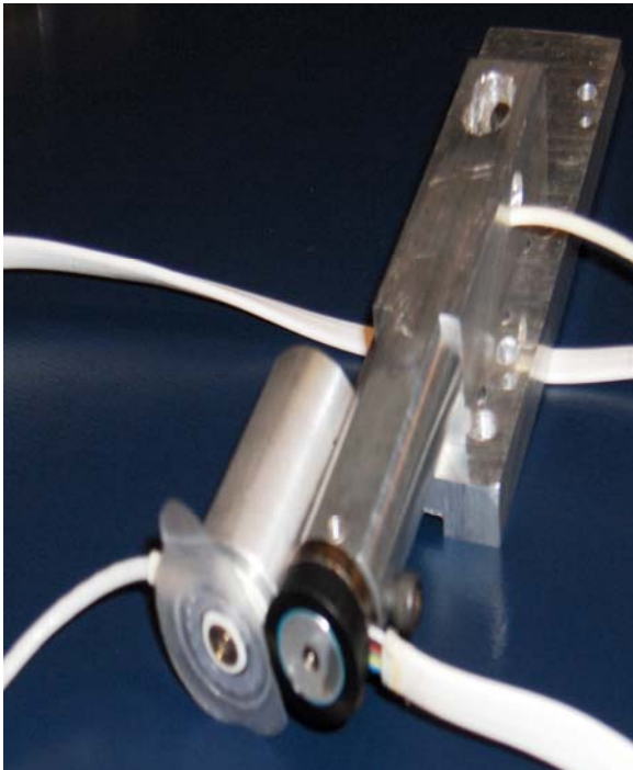
Figure 2. Combined indenter head (left) on computer controlled indenter (right)
