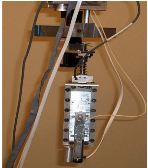
Figure 2. Combined indenter head (left) on computer controlled indenter (right)
