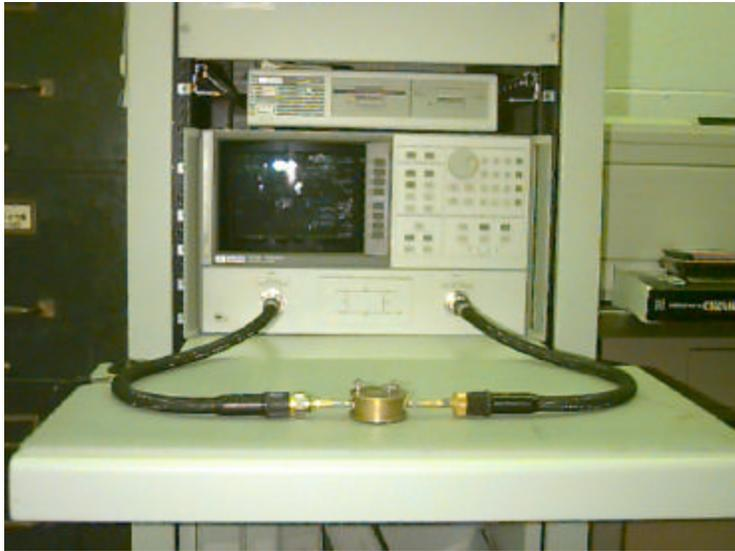
**Figure 13** Courtney method set-up for the measurement of the dielectric constant.
