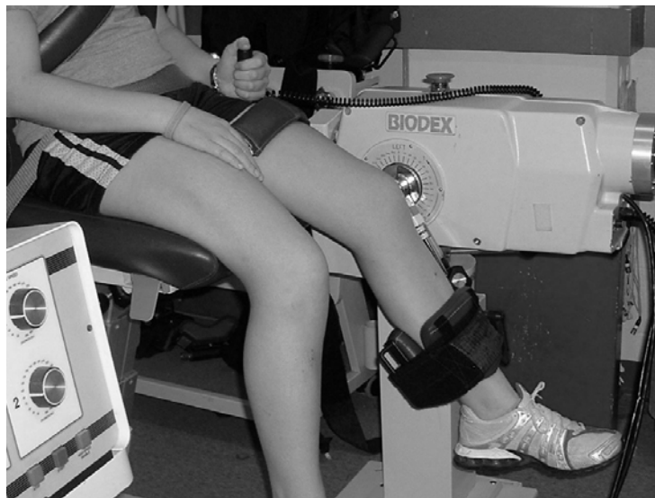
Figure 4. Strength Testing Setup. Subjects were seated with the knee angle set at 45° flexion. Isometric knee flexion and extension strength were collected at 1000 Hz using a Biodex AP System 2 (Biodex Medical Systems, Inc., Shirley, NY).
