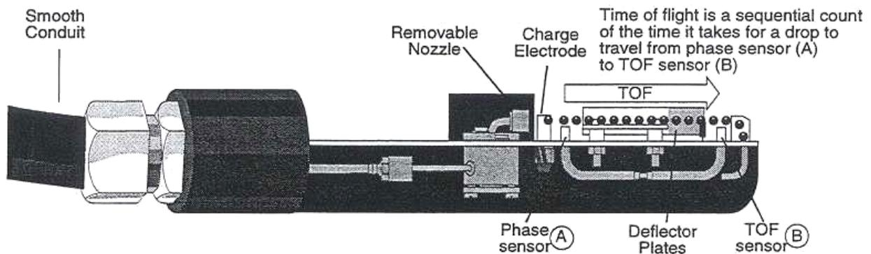
**Figure 8: Side view of CIJ print head with drop formations**
