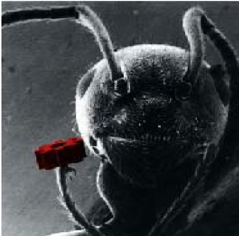
**Figure 1: Eye catching example of an ant holding a LIGA fabricated gear in its claw**
