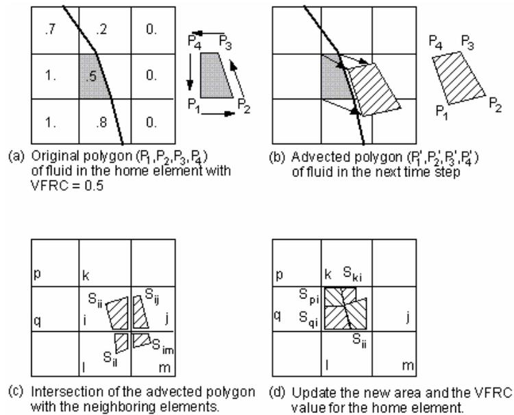
**Figure 39: Typical Advection Step in CLEAR-VOF Algorithm**
