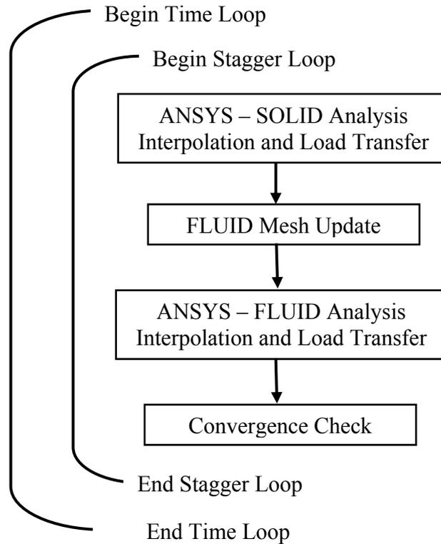
**Figure 28: Fluid-Solid Interaction Solution Algorithm**
