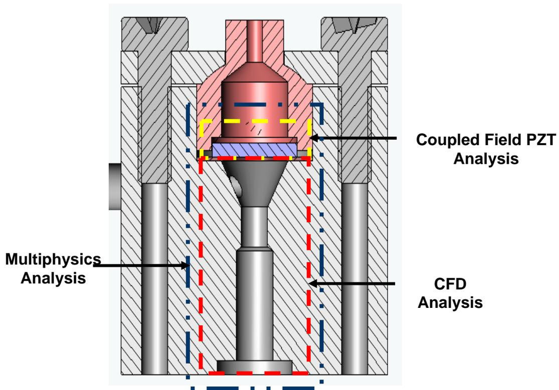
Figure 11: CIJ components and respective analysis types
