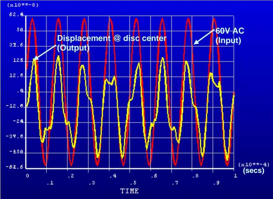
**Figure 23: Superposition of input voltage and output displacement waveforms for 100µs**
