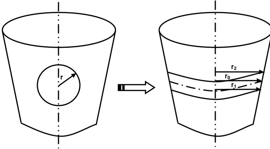
**Figure 43: Equivalent inlet area for axisymmetric CFD model**
