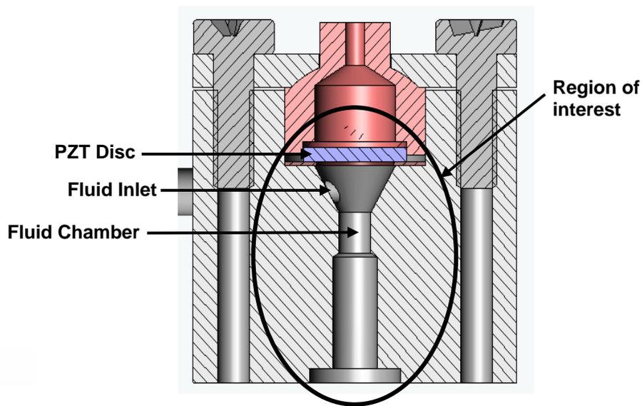
**Figure 26: Cross-sectional view of PZT modulator assemble components**
