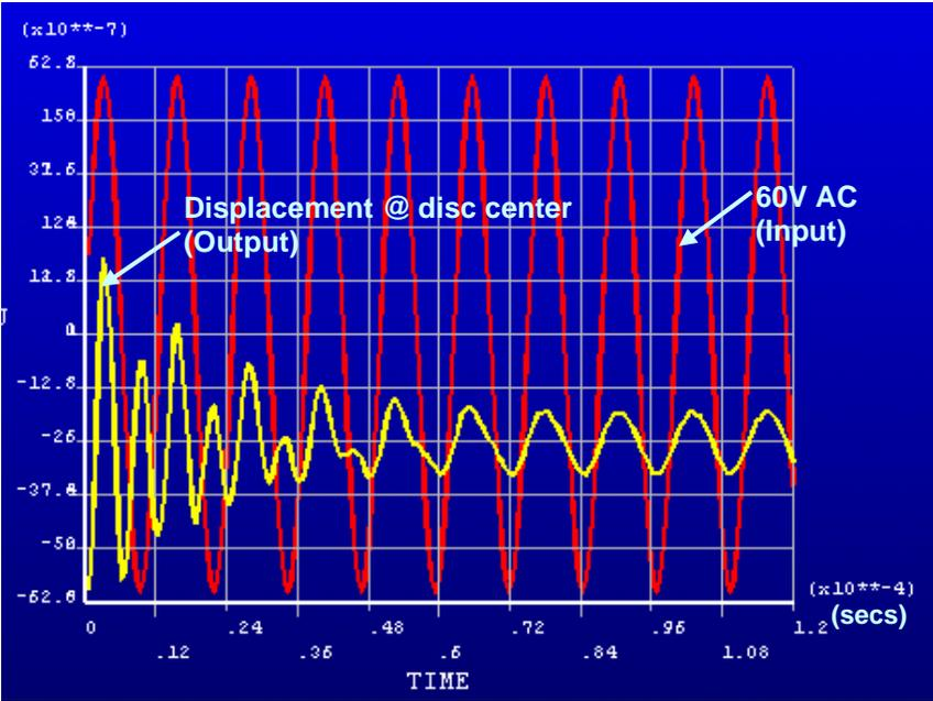
**Figure 24: Superposition of input voltage and output displacement waveforms for  $120\mu\text{s}$  (FSI)**
