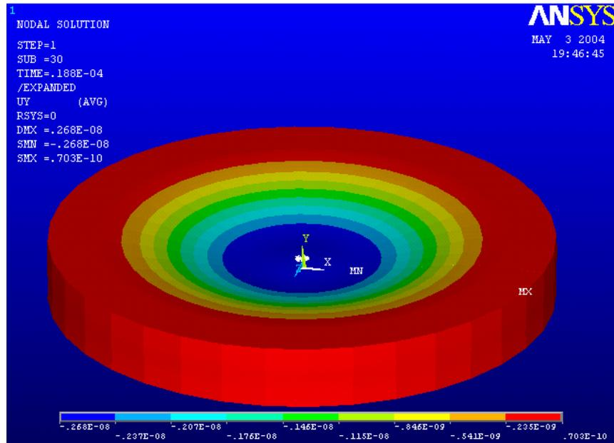
**Figure 22: Displacement values of the 3D PZT disc at 18.75  $\mu$ s in (m)**
