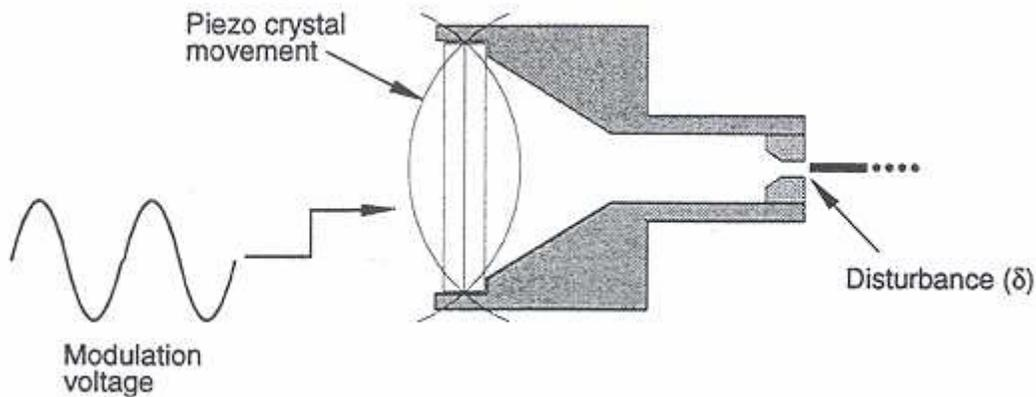
**Figure 9: Piezoelectric crystal perturbation on the ink**
