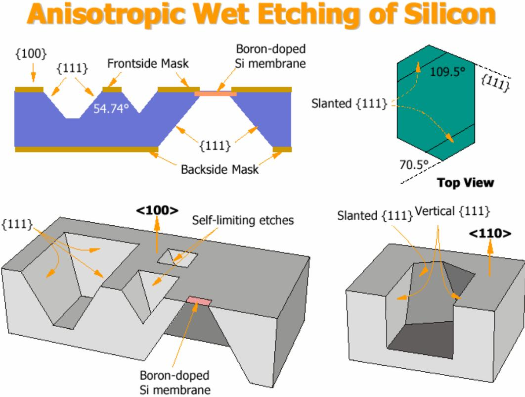
Figure 3: Anisotropic Wet Etching Process
