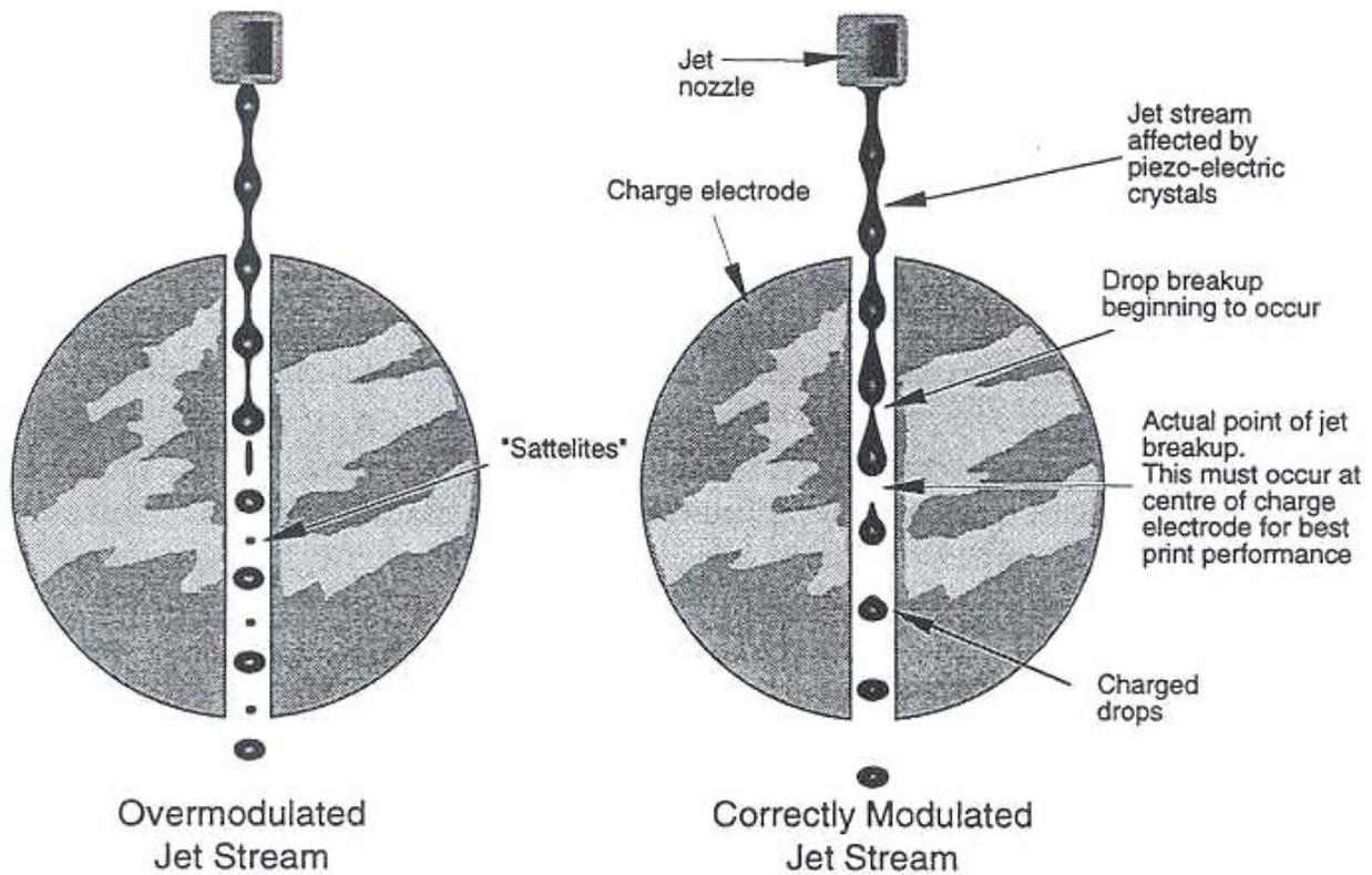
**Figure 10: Modulation modes and satellite formations**
