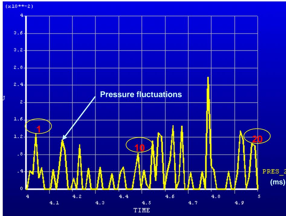
**Figure 45: Pressure fluctuations at breakup length from 4 to 5 milliseconds**
