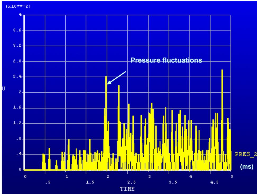
**Figure 44: Pressure fluctuations at breakup length (1.5mm) over 5 milliseconds**
