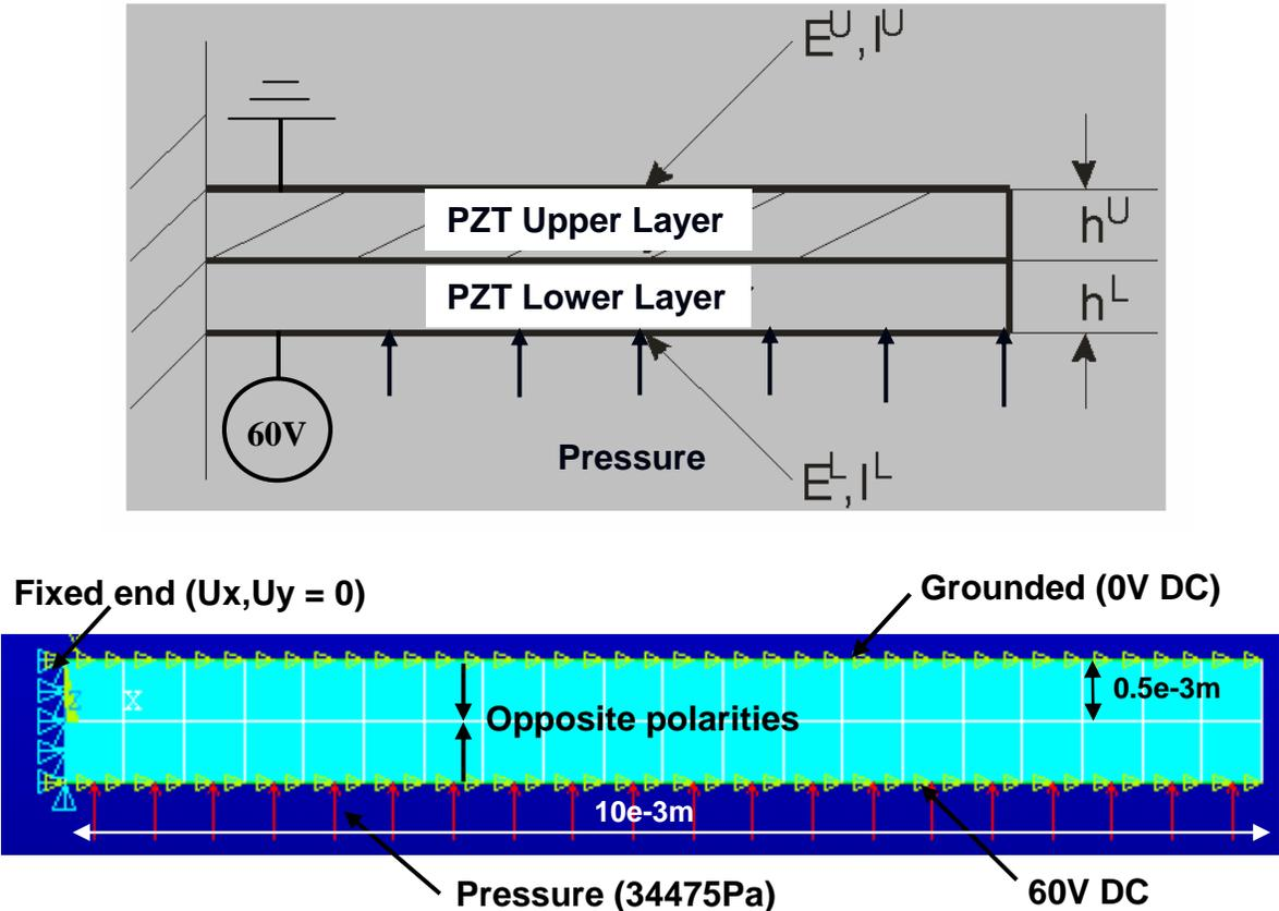
**Figure 16: Schematics and boundary conditions of PZT bimorph cantilever beam**
