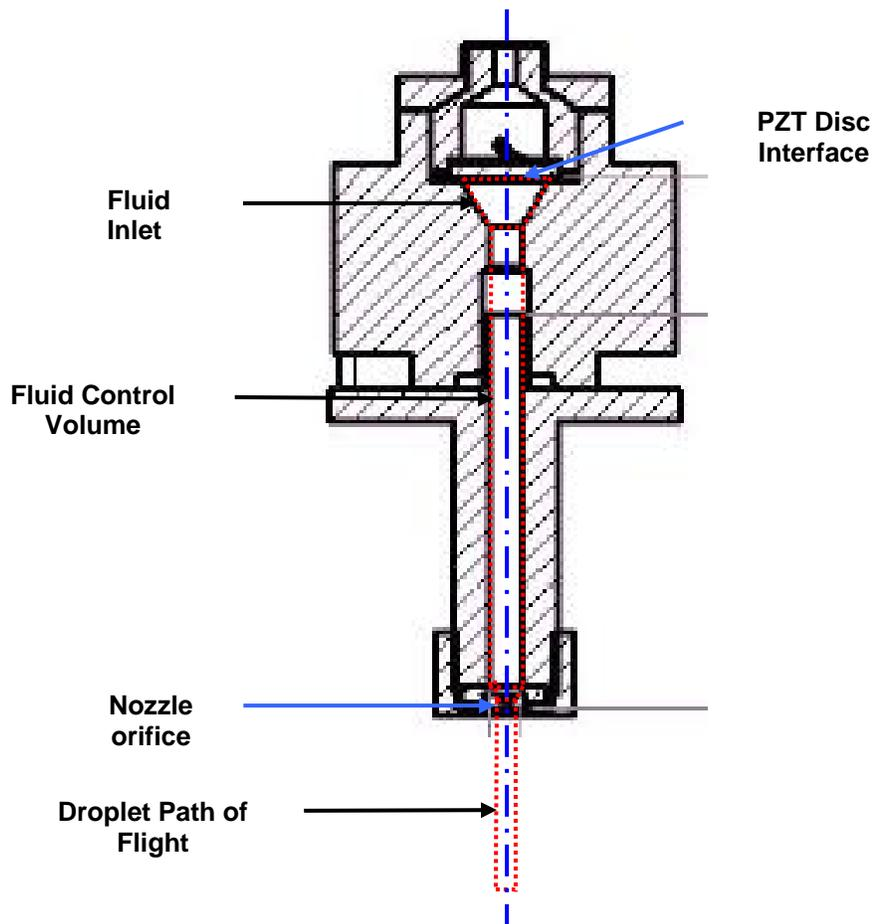
**Figure 40: Control Volume for CFD Analysis**
