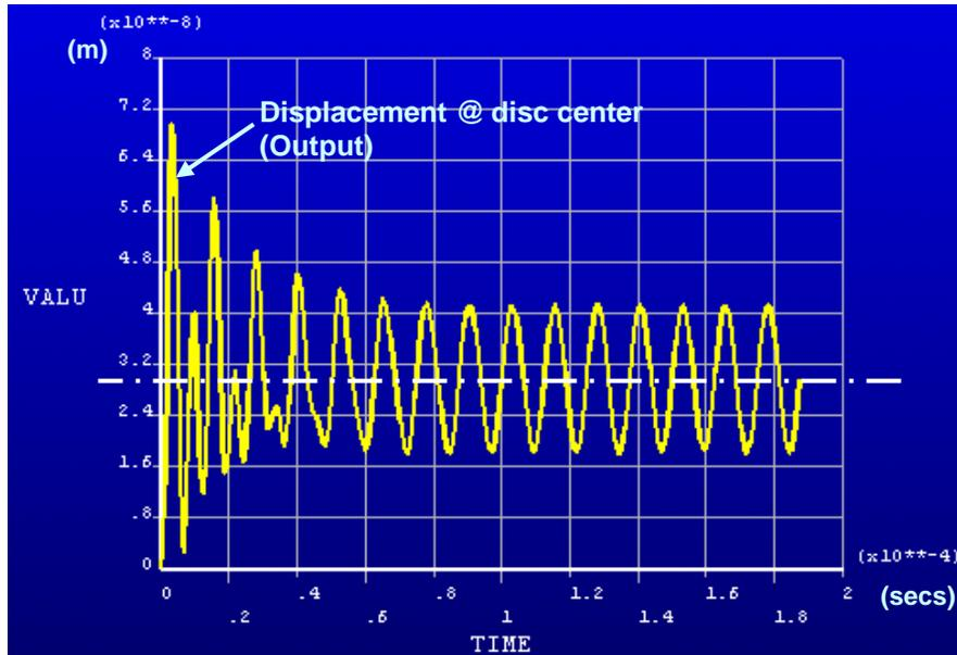
Figure 35: PZT disc displacement at 20psi, 80 kHz, 60V, with DISP = 0.012 $\mu$ m
