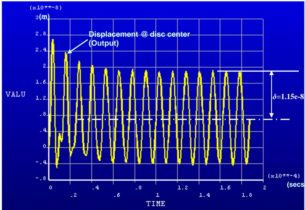
**Figure 33: PZT disc displacement at 5psi, 80kHz, 60V, with DISP = 0.0115 $\mu$ m**
