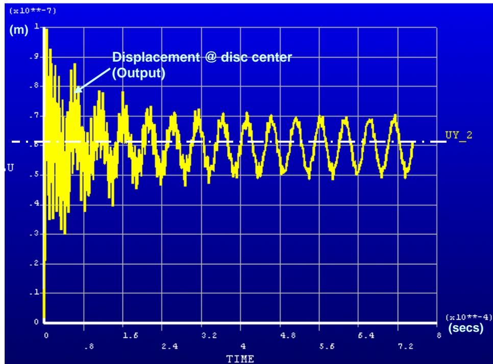
**Figure 37: PZT disc displacement at 40psi, 20 kHz, 60V, with DISP = 0.0105 $\mu$ m**
