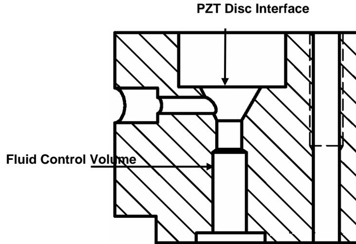
**Figure 27: Cross-sectional view modeled of PZT modulator assembly components**
