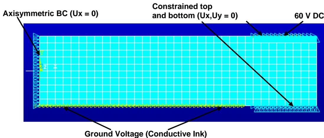
**Figure 18: PZT bimorph disc and finite element boundary conditions**
