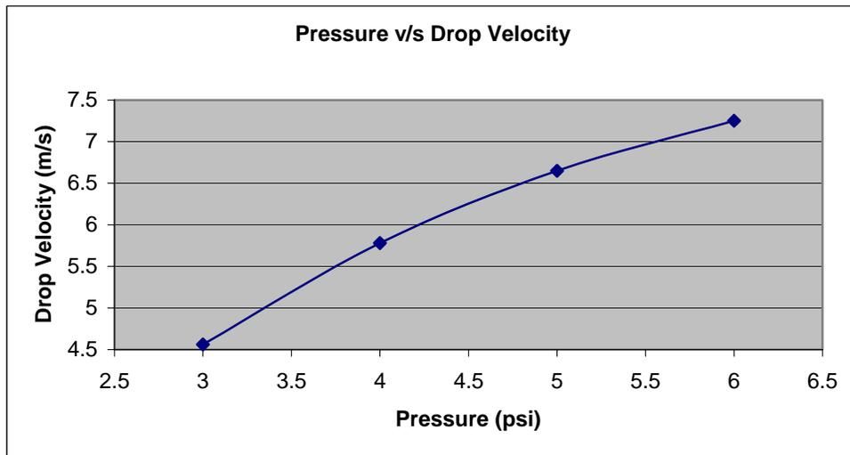
**Figure 50: Pressure v/s Drop Velocity**
