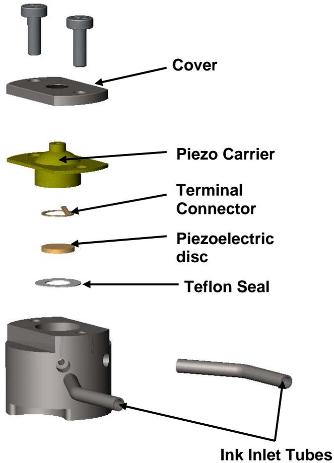
**Figure 13: Exploded view of piezoelectric modulation assembly**
