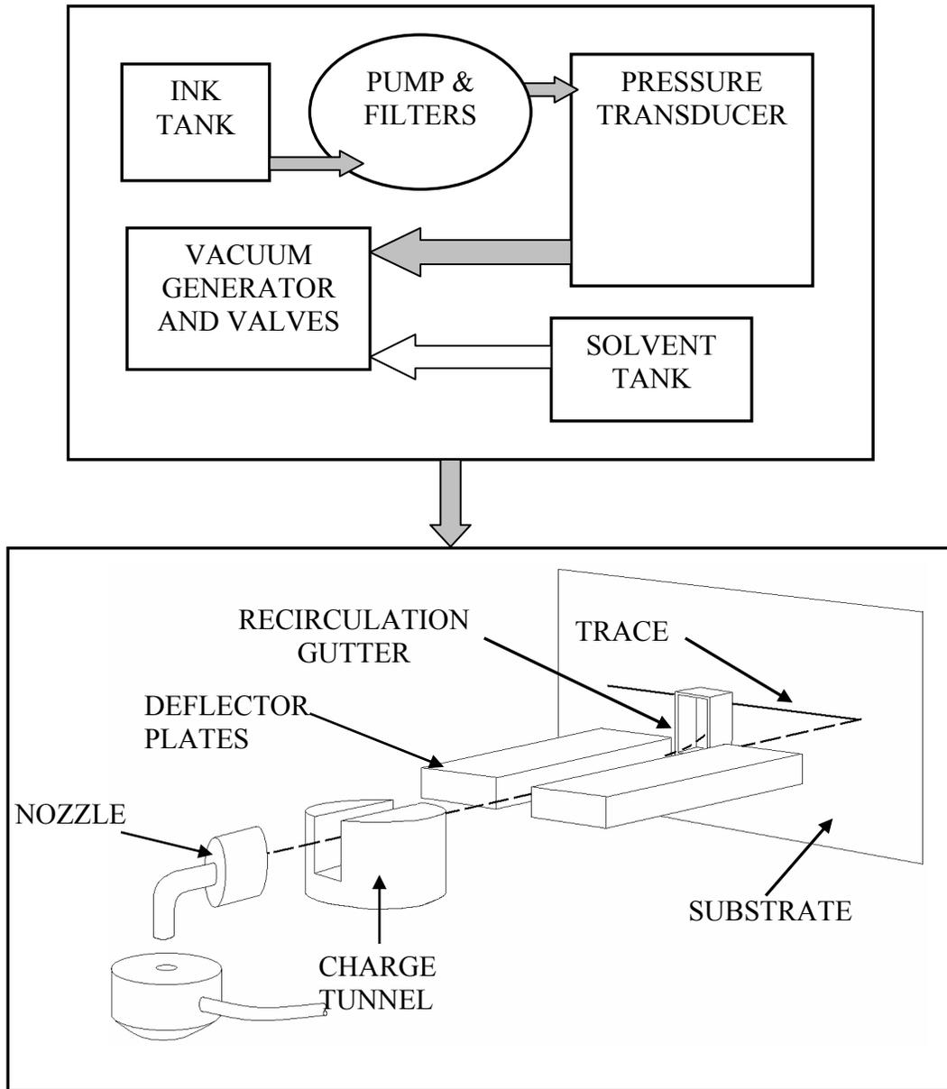
**Figure 7: Control System and Print Head Schematics**
