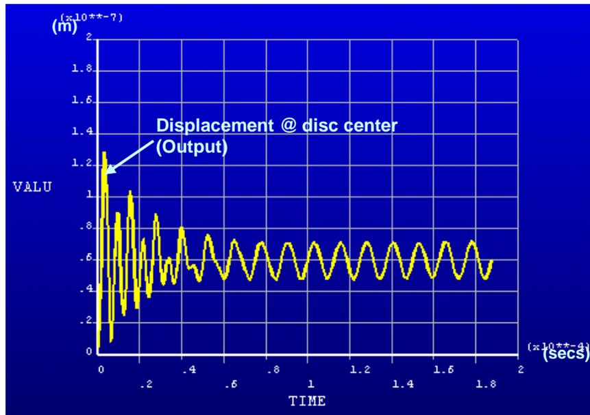
**Figure 25: Displacement waveform of PZT disc for 187.5 $\mu$ s (FSI)**
