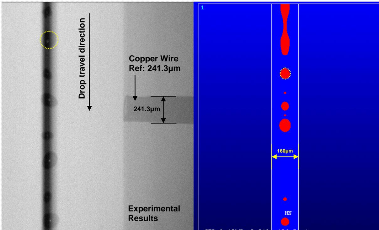
**Figure 59: Droplet Profile and Volume Comparison**
