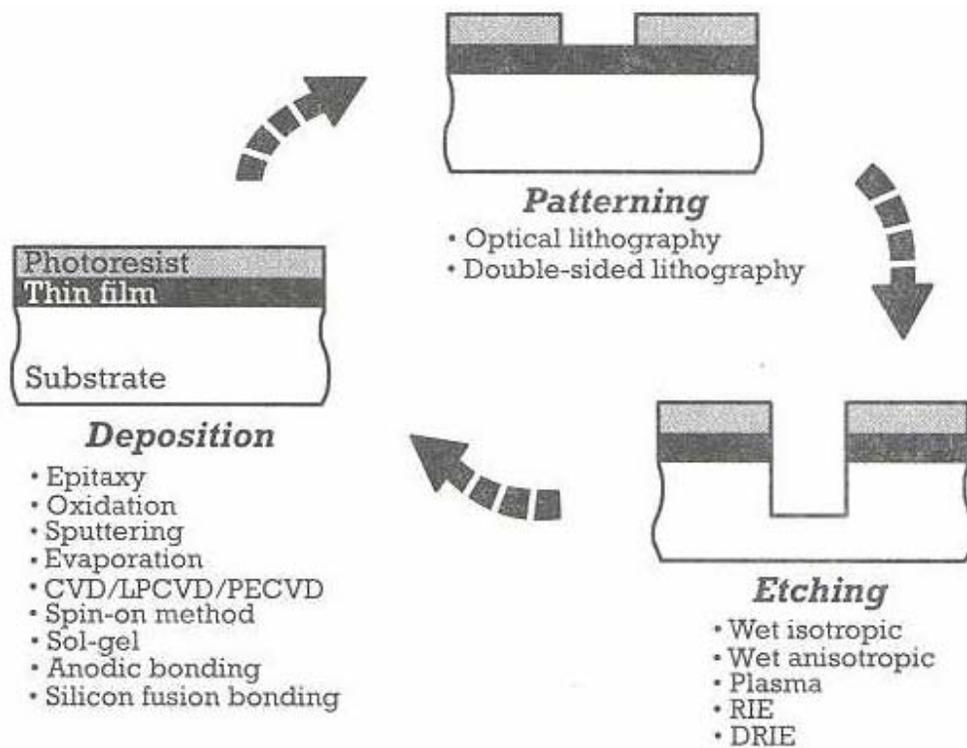
**Figure 2: Illustration of basic process flow in micromachining**
