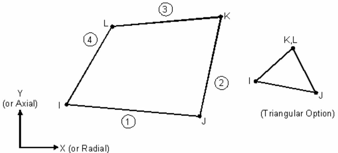
**Figure 41: FLUID141 element geometry**
