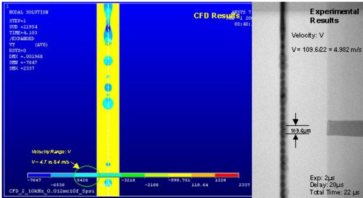
**Figure 60: Droplet Velocity Comparison**
