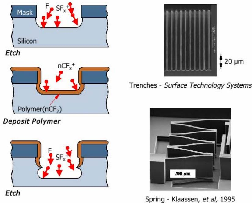
**Figure 4: Deep Reactive Ion Etching (DRIE) process**
