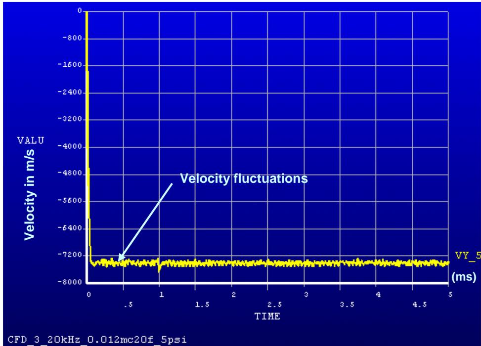
**Figure 46: Fluctuations of velocity at the orifice exit over time**
