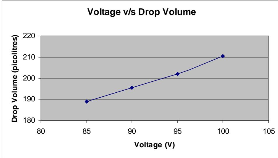
**Figure 53: Voltage v/s Drop Volume**
