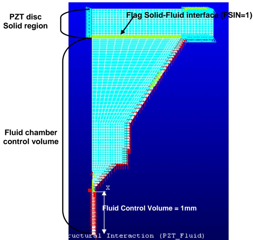
**Figure 32: Boundary conditions on axisymmetric Multiphysics model**
