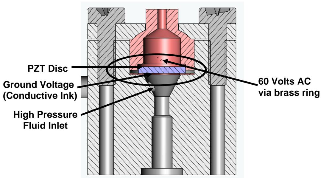
**Figure 14: Cross-sectional view of piezoelectric disc within PZT**
