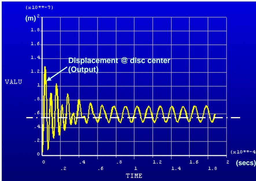
Figure 36: PZT disc displacement at 40psi, 80kHz, 60V, with DISP = 0.0115 $\mu$ m
