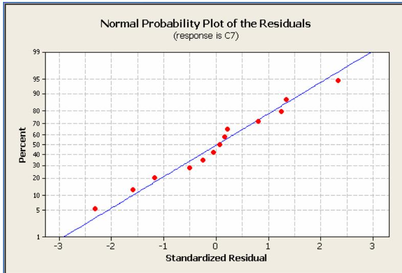
**Figure 70: Normality Plot for Response (Droplet Volume)**
