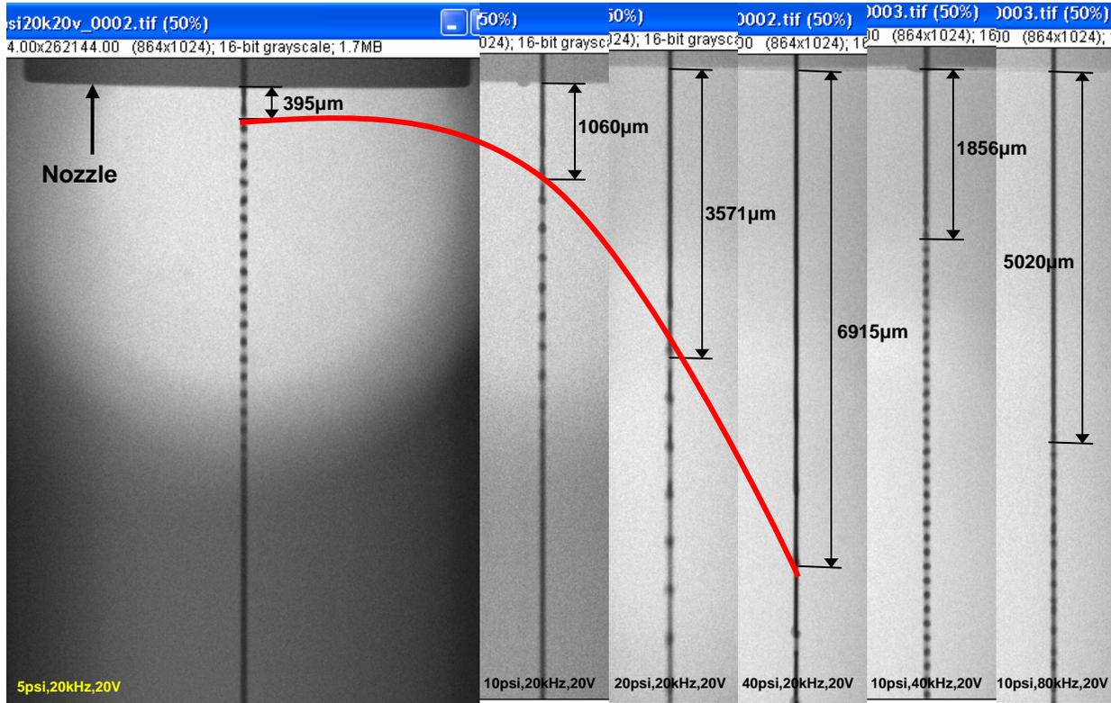
**Figure 58: Variations in droplet breakup lengths**
