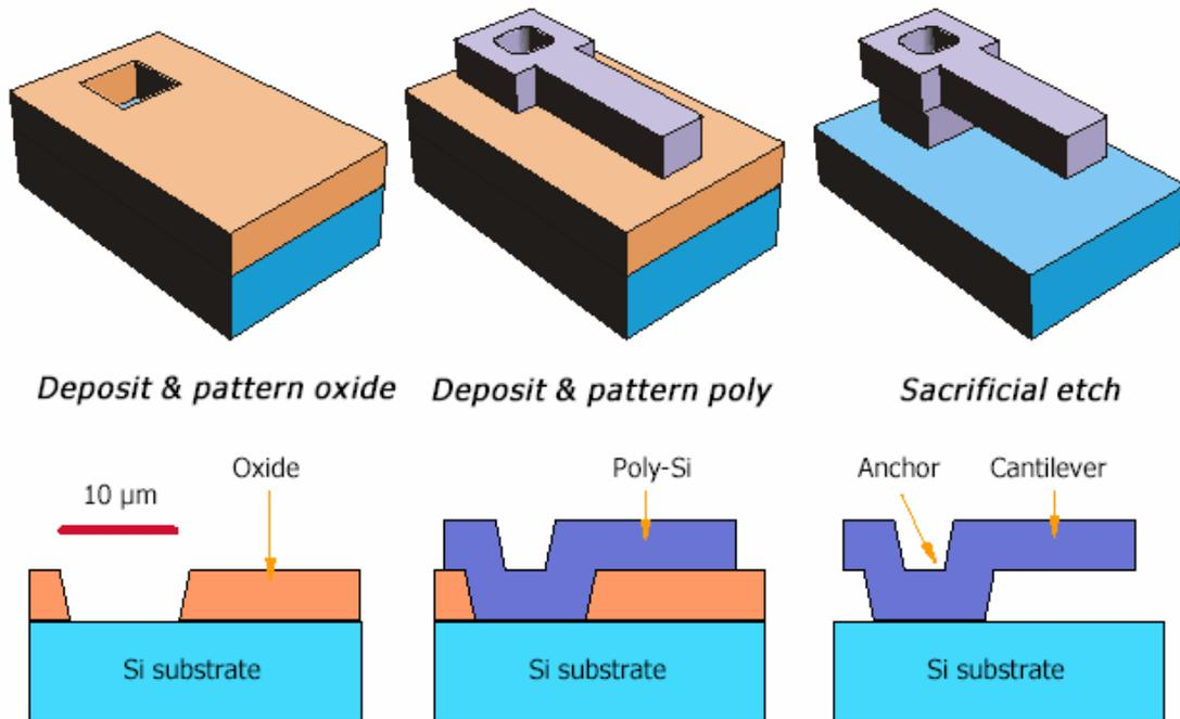
**Figure 5: Surface Micromachining Process**
