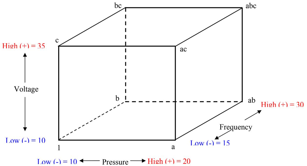
**Figure 61: Geometric view of  $2^3$  factorial design**
