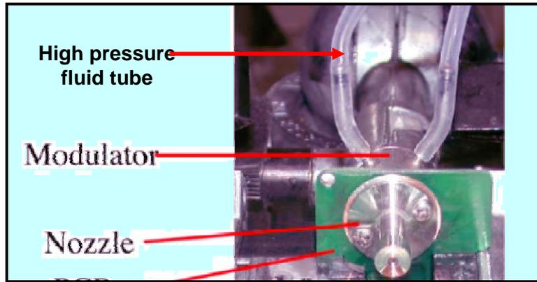
**Figure 57: PZT Modulator Assembly**
