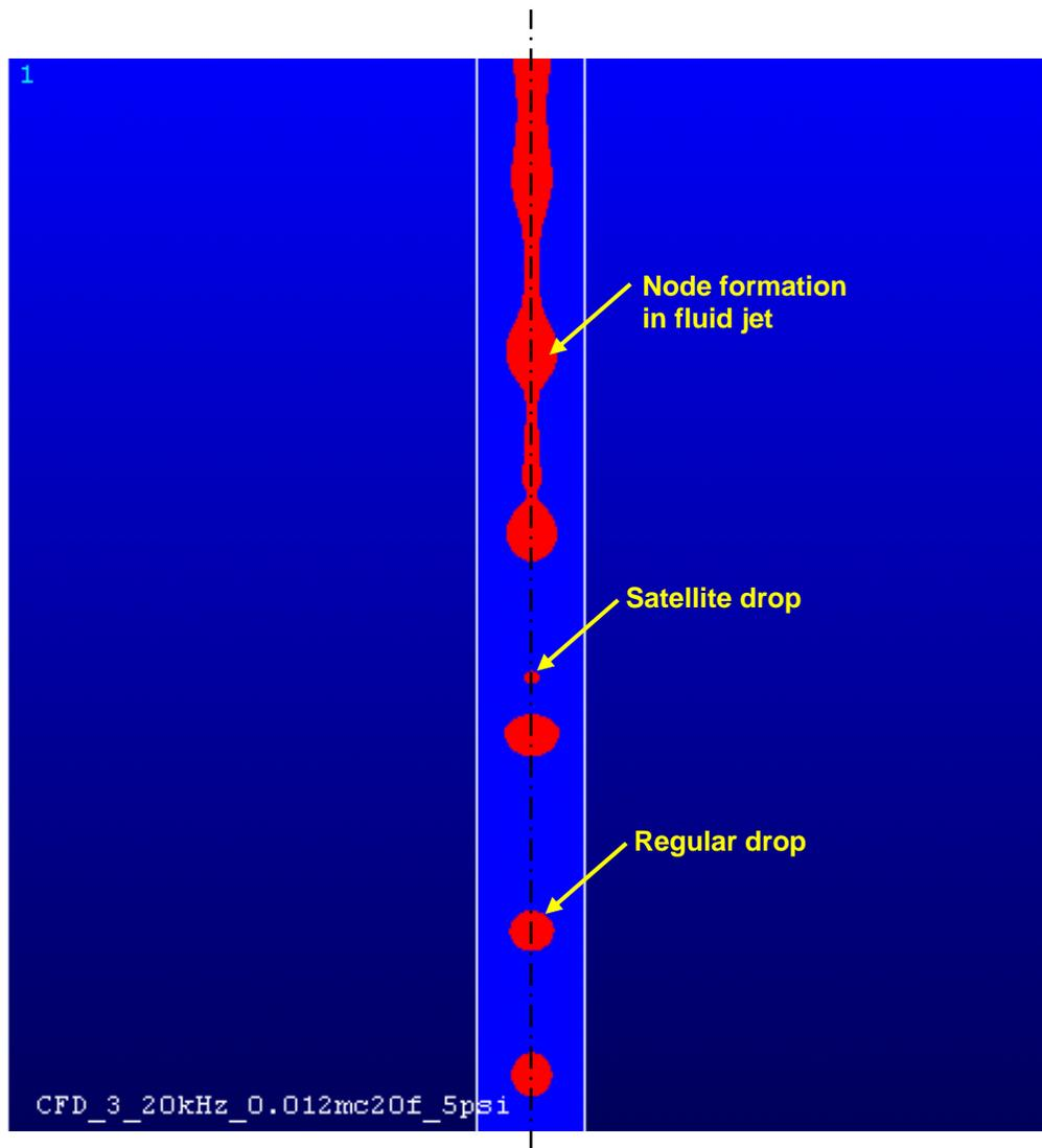
**Figure 47: Droplet generation at 4ms**
