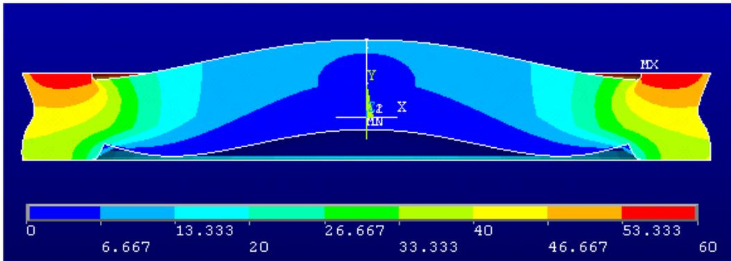
**Figure 20: Voltage drop across the PZT disc in volts (cross sectional view)**
