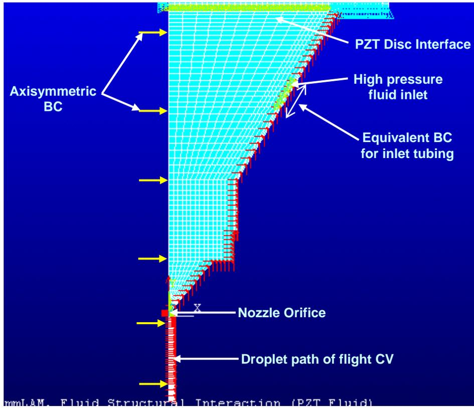
**Figure 29: Boundary conditions and loading of CFD model**
