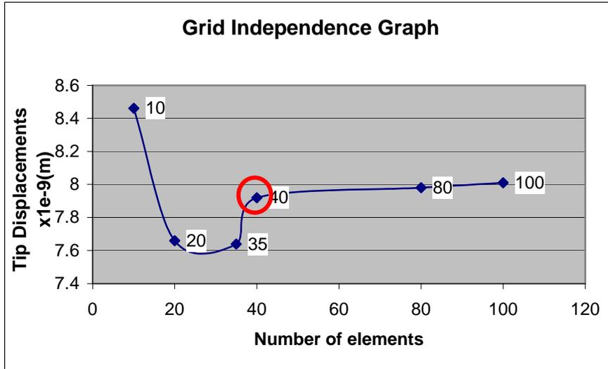
**Figure 19: Displacement at disc center v/s number of elements along the PZT disc radius**
