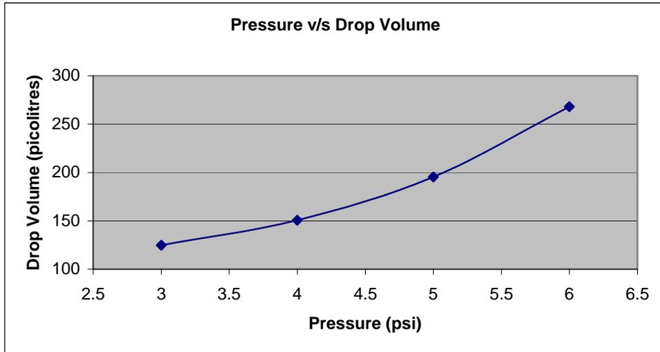
**Figure 49: Pressure v/s Drop Volume**
