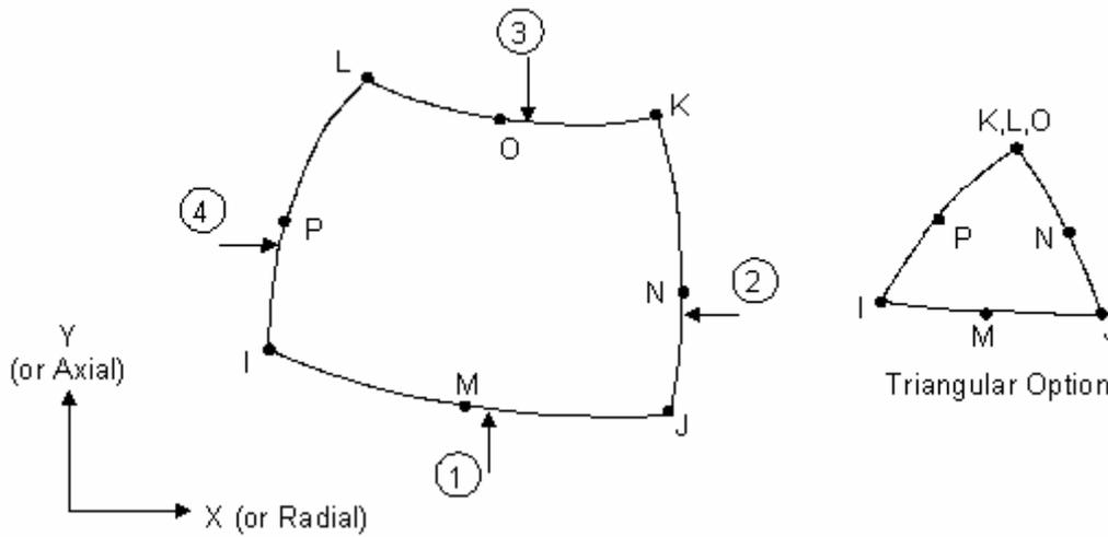
**Figure 15: Geometry of PLANE 223 element**
