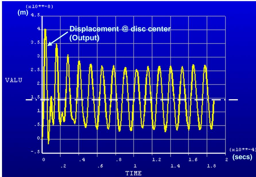
**Figure 34: PZT disc displacement at 10psi, 80 kHz, 60V, with DISP = 0.012 $\mu$ m**
