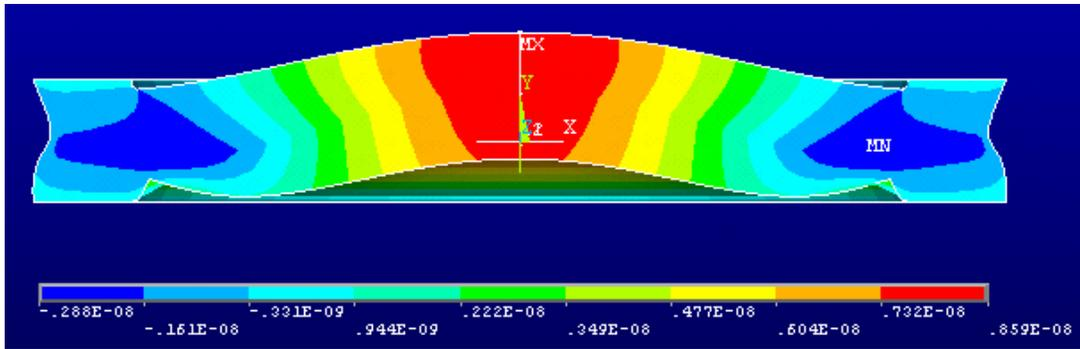
**Figure 21: Displacement values of the PZT disc in meters (cross sectional view)**
