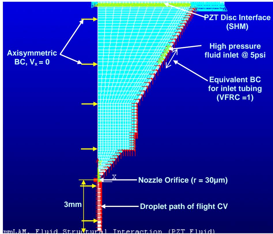
**Figure 42: Boundary conditions applied to the CFD model**
