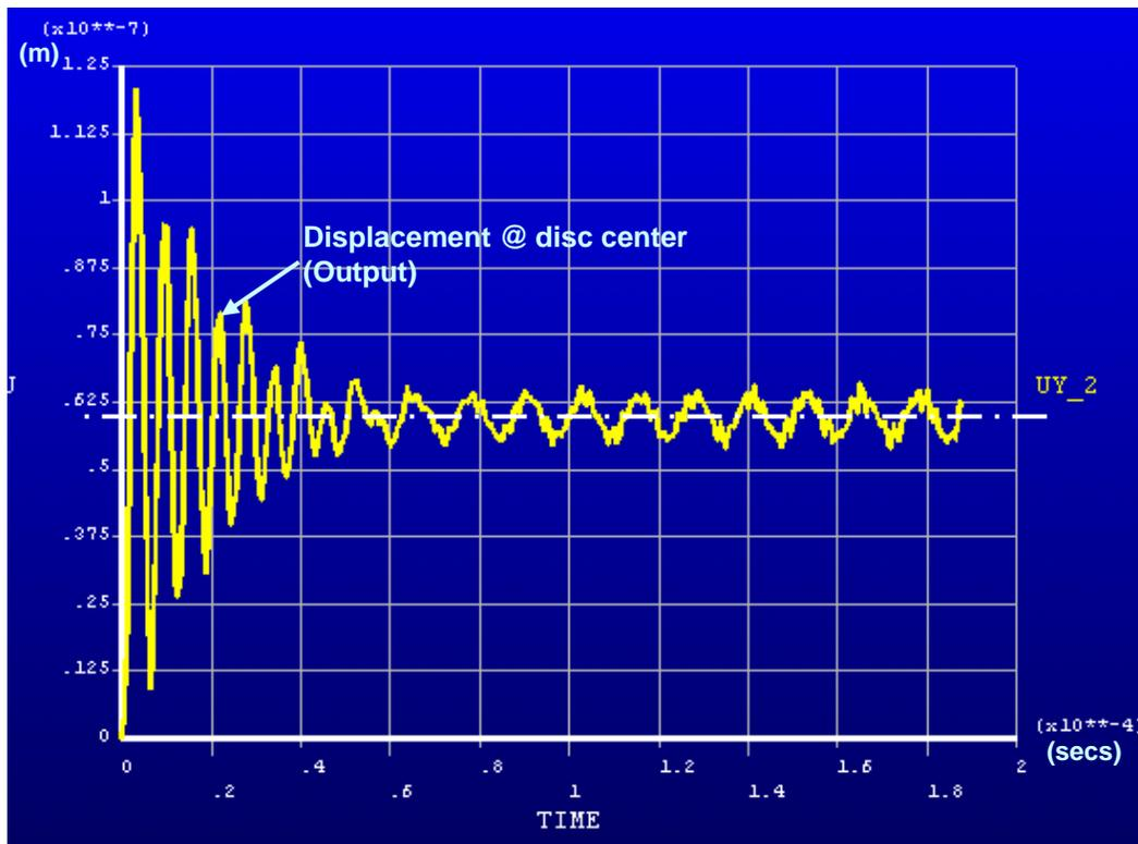
**Figure 38: PZT disc displacement at 40psi, 80 kHz, 20V, with DISP = 0.0045 $\mu\text{m}$**
