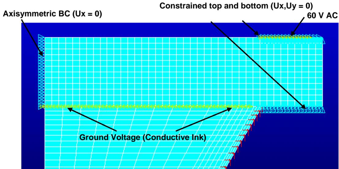
**Figure 31: Boundary conditions and voltage loading on axisymmetric PZT disc**
