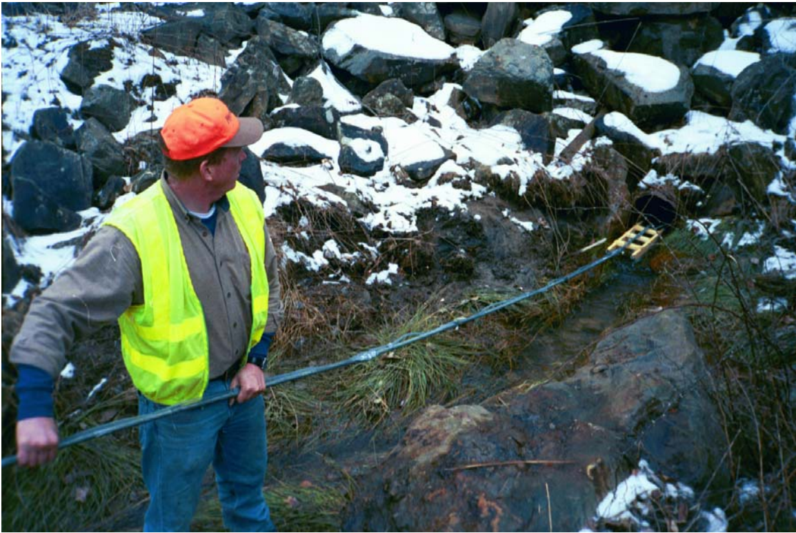
Figure 11. Sled being inserted the SLB3 drain pipe to collect water samples from original spring discharge
