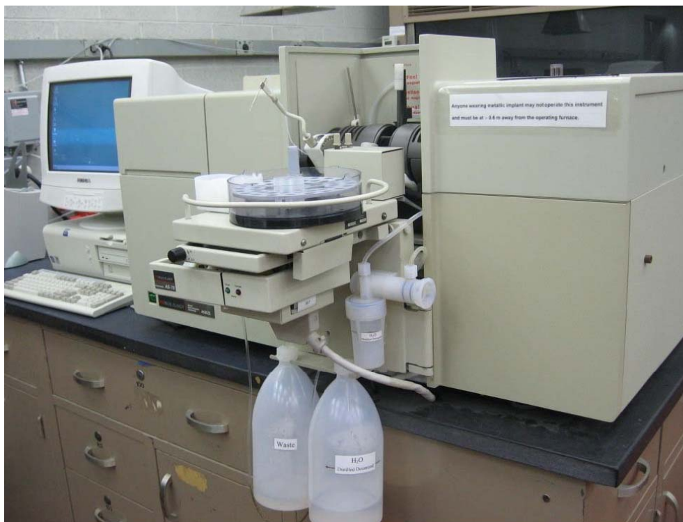
Figure 3.3 Graphite Furnace atomic absorption spectrometer (Perkin Elmer™4100ZL).
