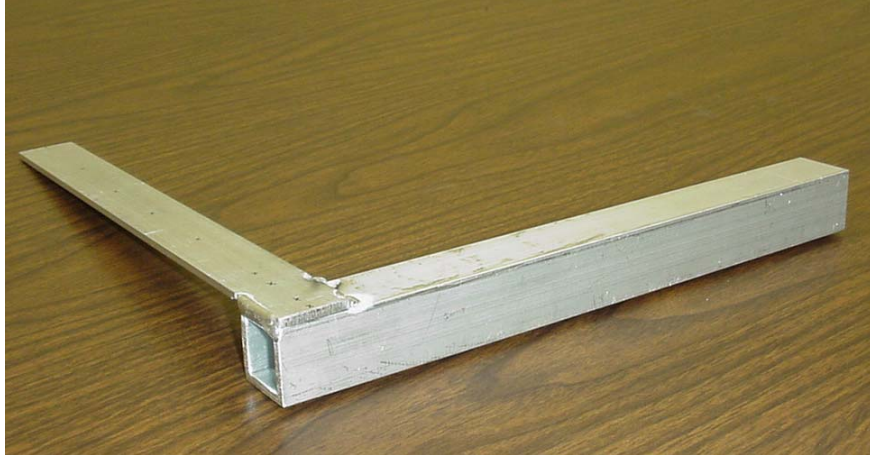
Figure 6-38 Welded joint for physical test
