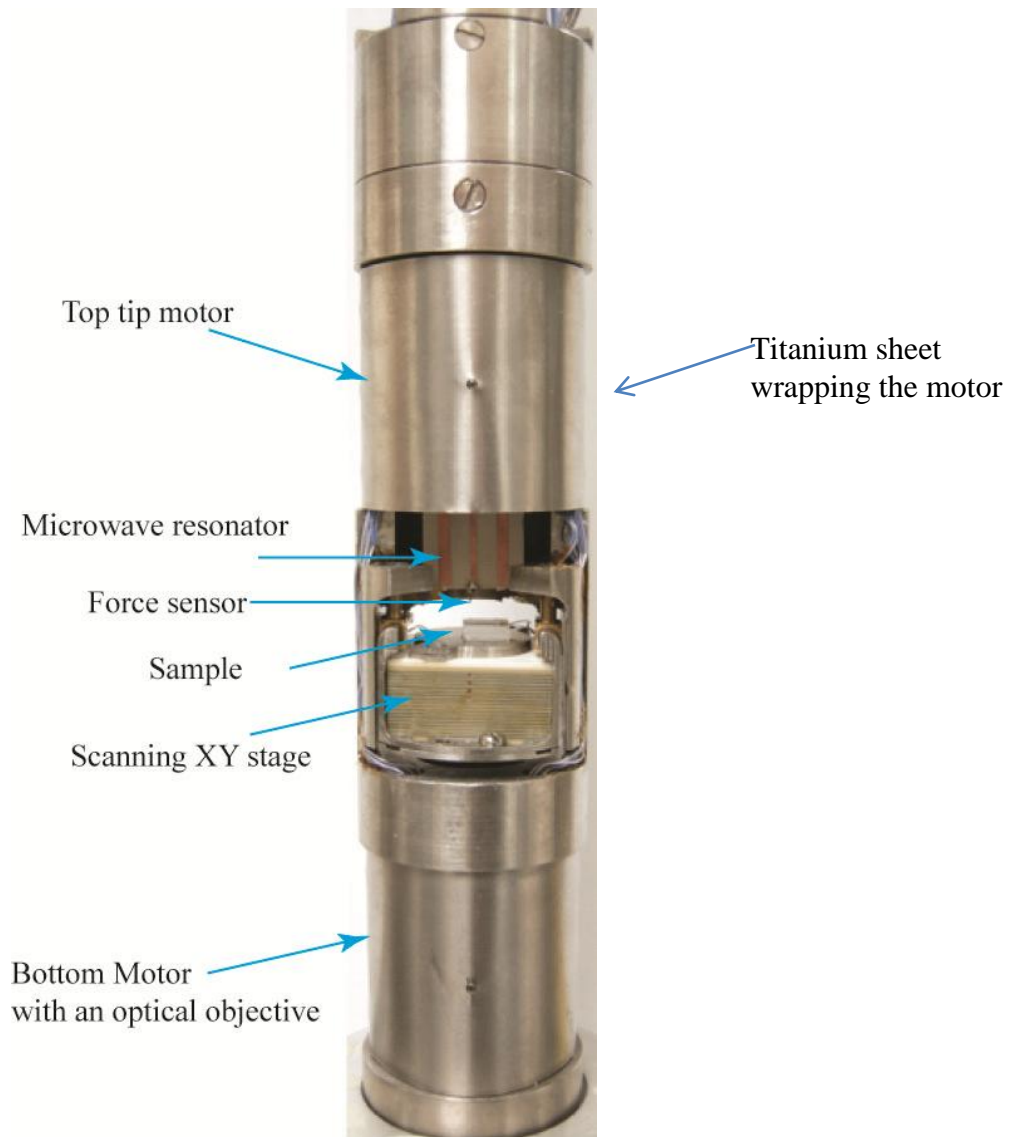
Fig. A.1 Photograph of the microscope. The microscope consists of two approach motors. The top motor holds the AFM tip and microstrip resonator, and the bottom motor holds an optical objective. Each motor is driven by 6 piezo stack assemblies. The sample stage is a peizostack scanner with a range 6\ \mu\text{m}\times 6\ \mu\text{m} in X and Y directions. At low temperature, the range is reduced to about 1.5\ \mu\text{m}\times 1.5\ \mu\text{m} .
