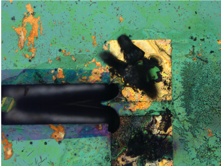
Figure 6.3. Illustration of a beam that literally exploded during poling. This was the result from an electric field that was too large
