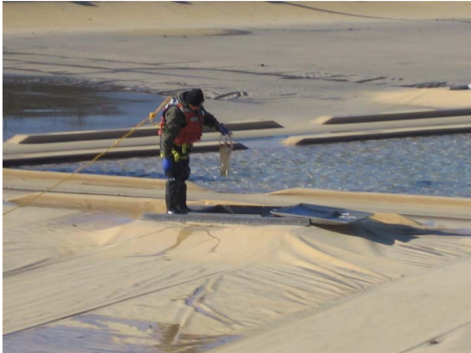
Figure 23. Lanpher Reservoir, dropping sampler down through hatch.
