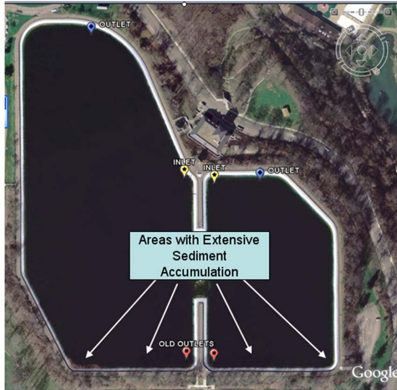
Figure 30. Locations of extensive sediment accumulation in Highland No. 1 Reservoir.
