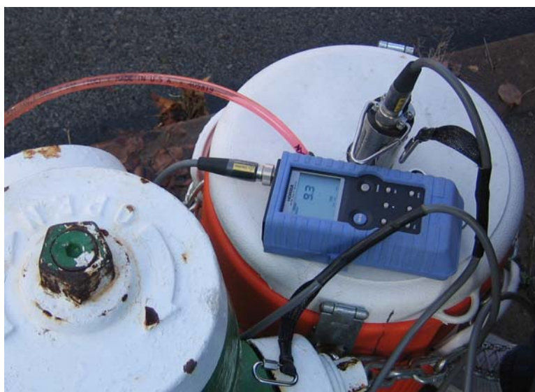
Figure 21. Collecting data from hydrant continuous fluoride analyzer.
