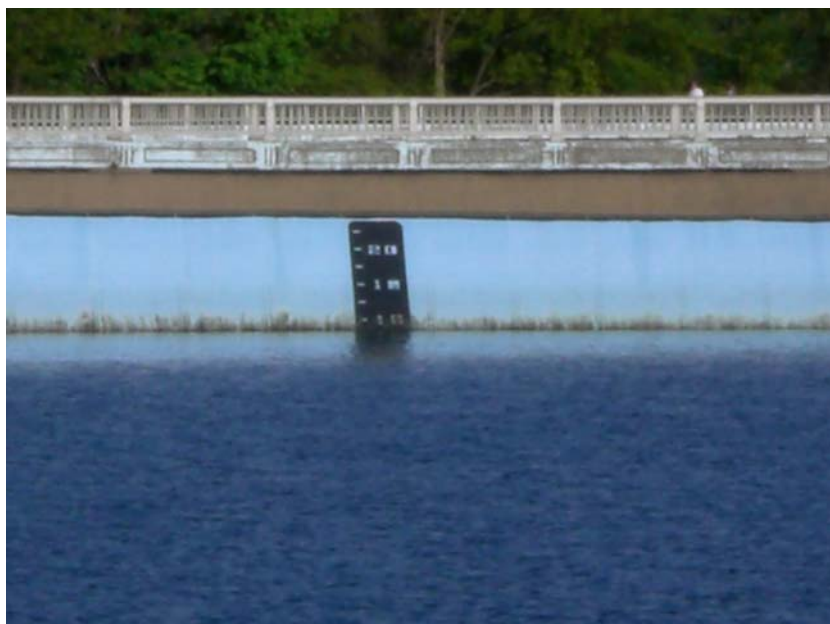
Figure 28. Highland No. 1 depth meter.
