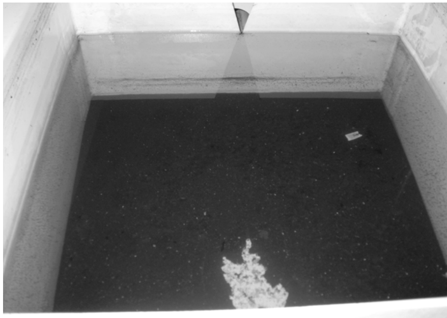
Figure 64. Runoff water from control roof stored in the weir box (Homestead)
