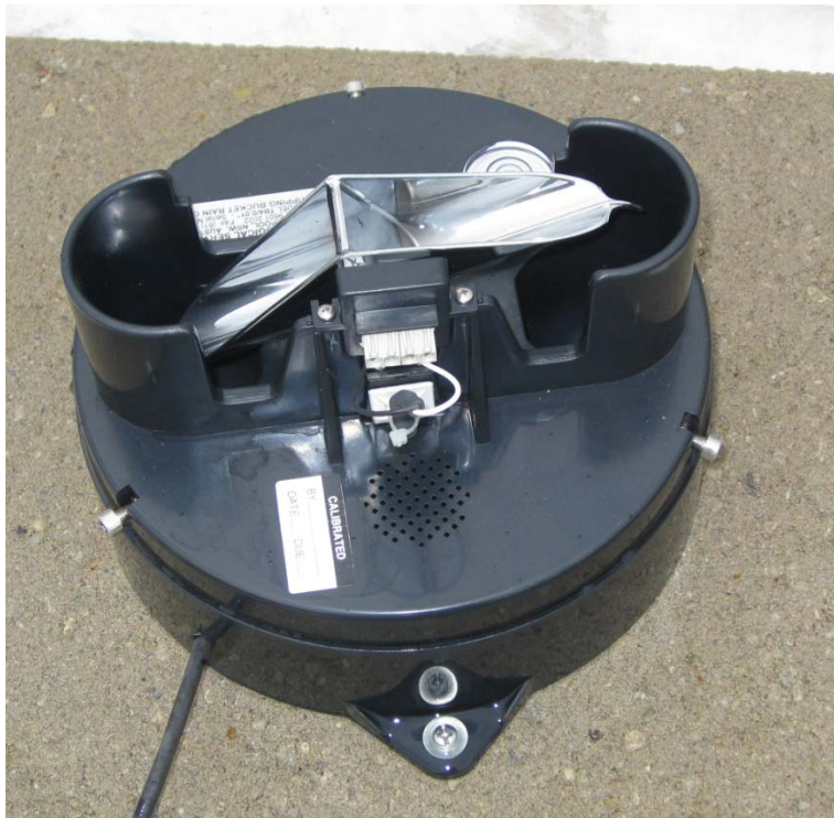
Figure 18. Tipping bucket (silver) inside the rain gauge
