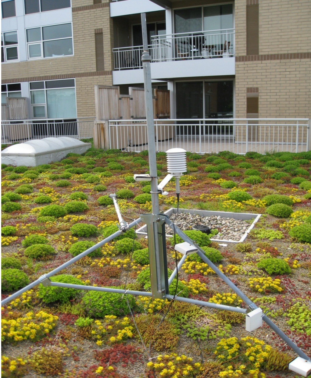
Figure 8. One of the Tripods for monitoring temperature at green roof side (Giant Eagle)
