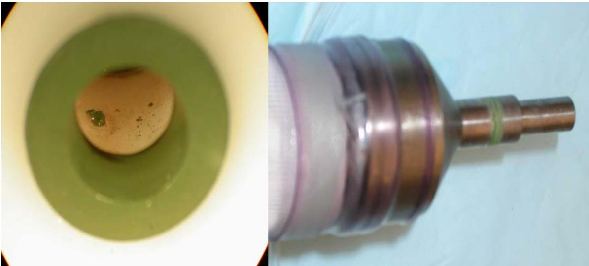
**Figure 3-4** Vyton seal exhibited debris in the original biohybrid lung prototype
