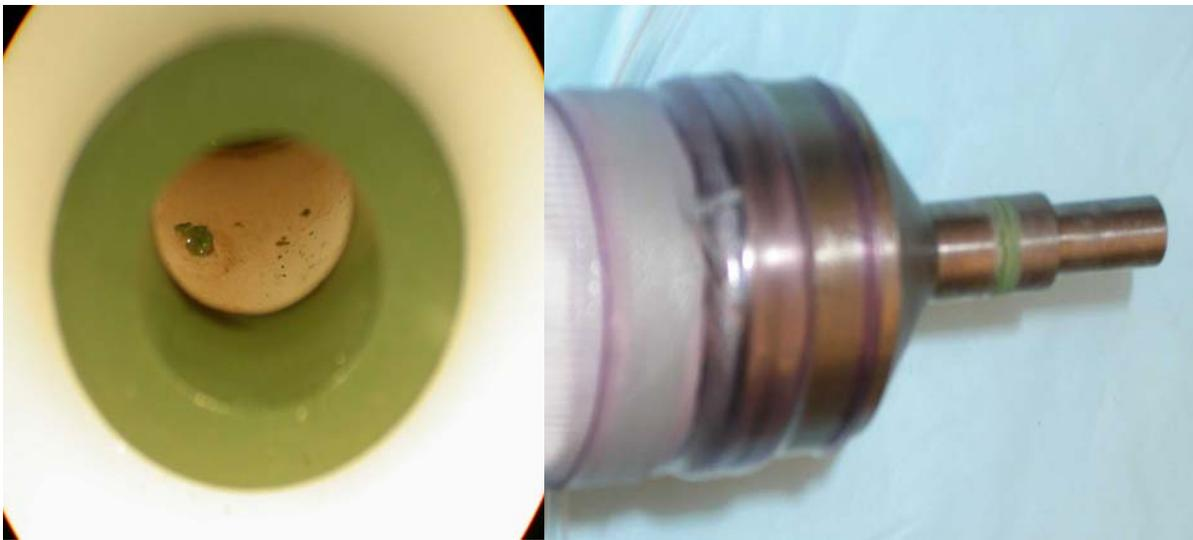
**Figure 3-4** Vytan seal exhibited debris in the original biohybrid lung prototype
