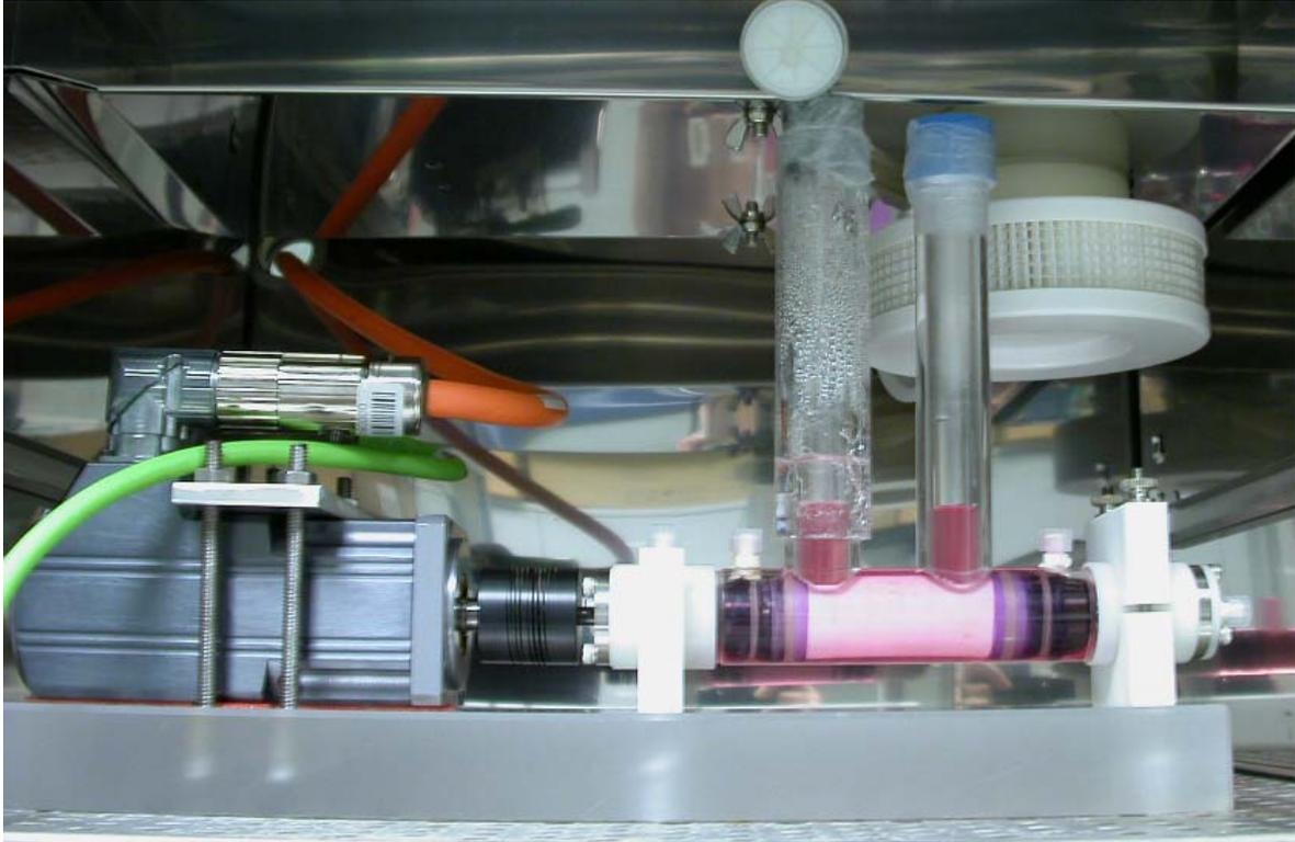
**Figure 3-5** Finalized biohybrid lung prototype
