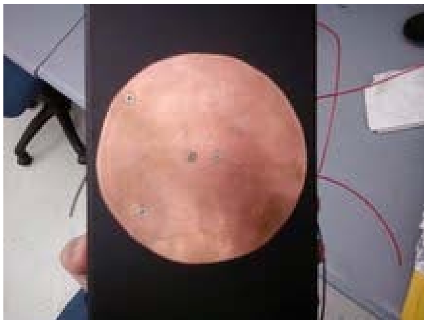
Figure 18: Copper plate attached to bottom of aluminum block
