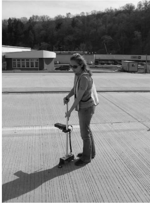
Figure 6.41. Surface profile measurements using the Dipstick™.
