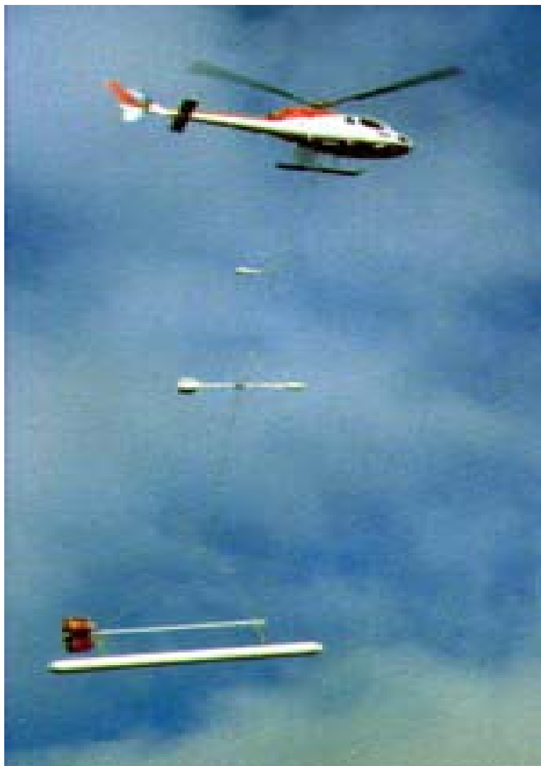
Figure 1.2: A Bell 412 helicopter was employed in the Collection of multifrequency conductivity, magnetic, and VLF data. National Energy Technology Laboratory, Department of Energy, URL; http://www.netl.doe.gov ).
