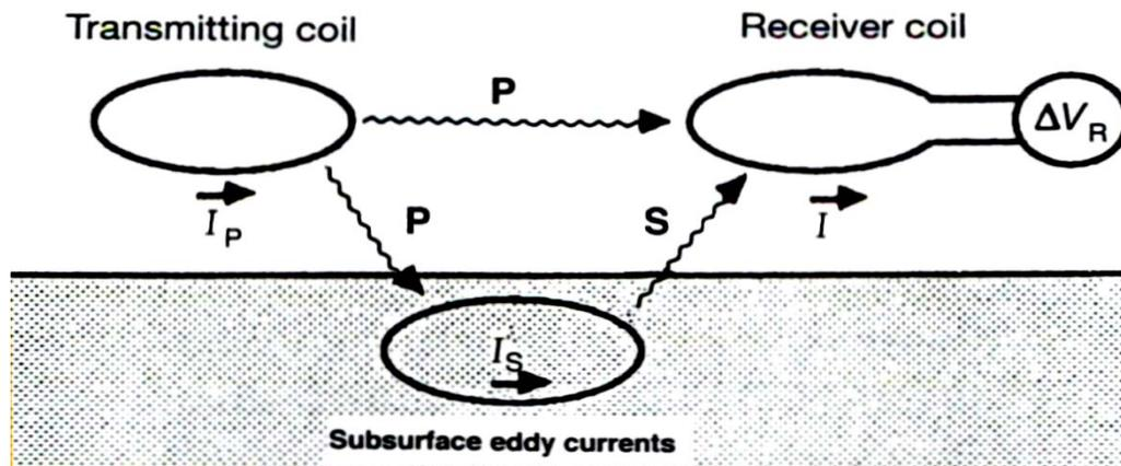
Figure 3.1: A generalized sketch of an electromagnetic induction prospecting system. The transmitting coil, energized with an alternating current ( $I_P$ ), produces a primary field, which induces eddy currents ( $I_S$ ) in the subsurface conductor. The receiver coil measures the resultant ( $R$ ) of the primary field ( $P$ ) and the secondary field ( $S$ ) induced by subsurface eddy currents (Sharma, 1997).
