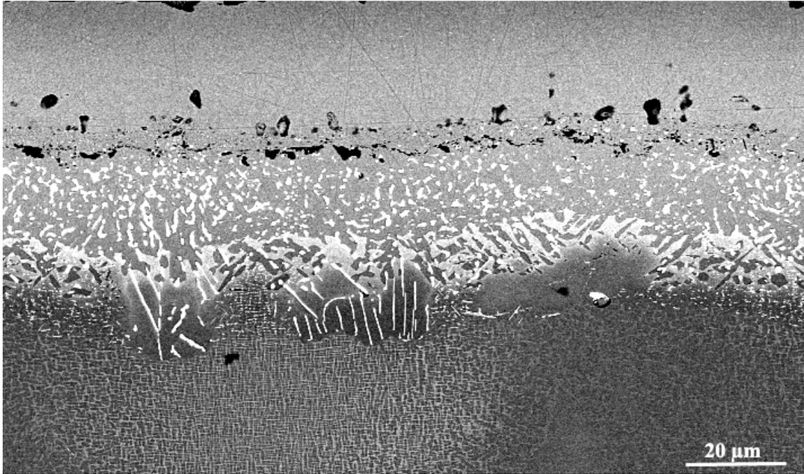
**Figure 7.10** The interdiffusion area below the thermal barrier coating system.
