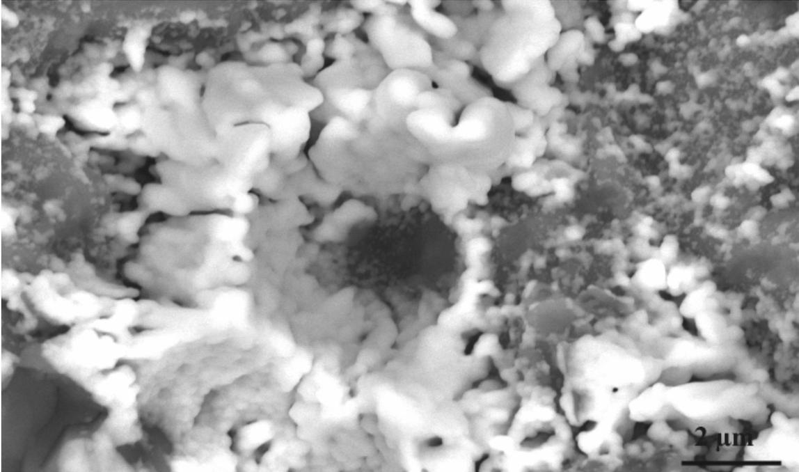
**Figure 7.58** YSZ grains attached to the TGO on the substrate surface after failure.
