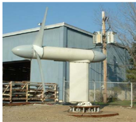
Figure 4: 35 kW turbine with downstream 3-bladed rotor, 5 m diameter that has the ability to yaw to accommodate reversing flow [28].
