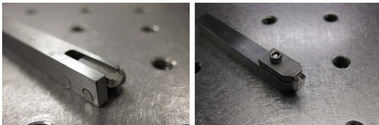
Figure E.2 (left) A sharp-cornered SiC cutting tool utilizing a single crystal of 6H SiC polished to a sharp cutting edge, mounted in a steel holder and shank. (right) A similar tool using single crystal 4H SiC polished to a sharp edge with a large circular radius, also mechanically mounted in a steel holder.
