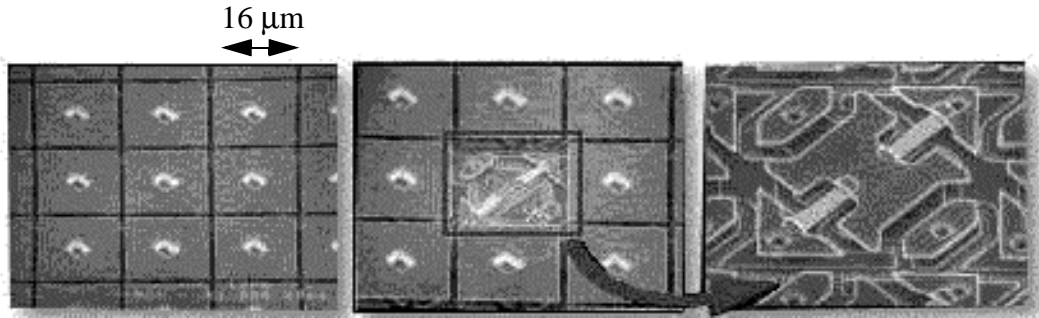
Figure 4 Texas Instruments's Digital Micro-mirror Device (DMD) (10)
