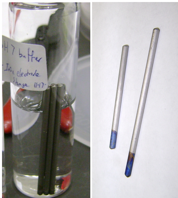
Figure 9: AEIROF electrodes on left have been stored in pH 7 buffer solution, while electrodes on right have been stored in air. Clearly the buffer solution storage has caused fading of blue iridium-oxide deposit, which is at the bottom of Ti rods.
