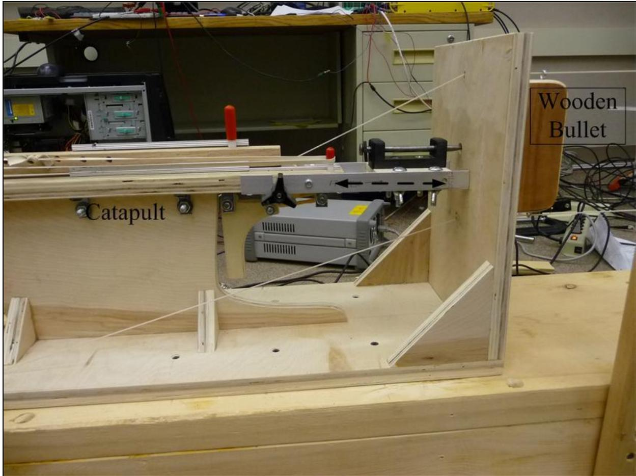
**Figure 76. Wooden Bullet Triggering System**
