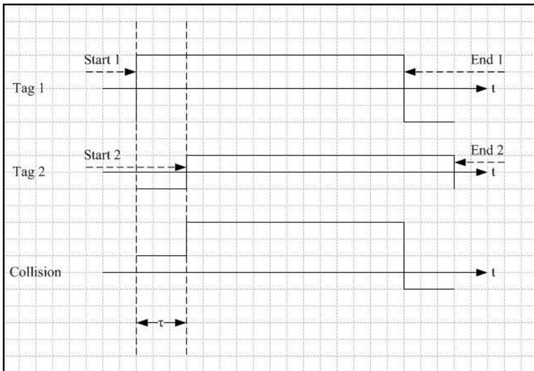
Figure 33. Superposition of Two Formation-1 Symbols
