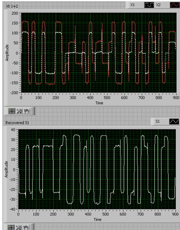
**Figure 103. 2-tag Collision Resolution Result using FastICA in FPGA (BLF=682 kHz)**
