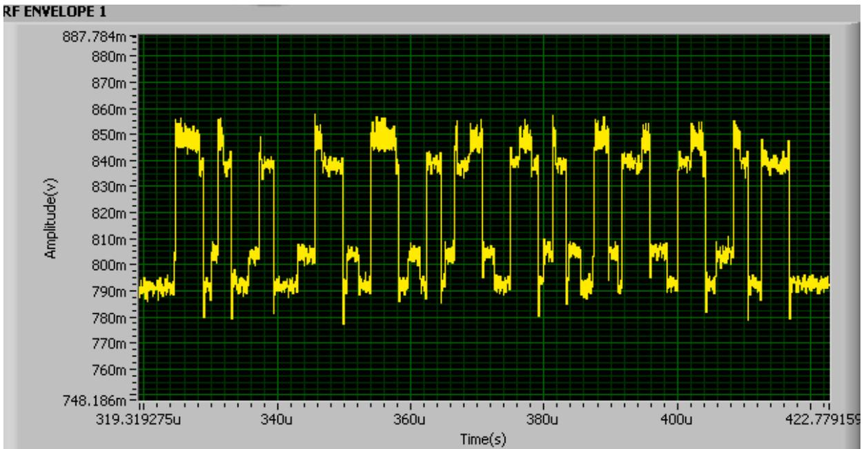
Figure 88. 2-tag Collision Signal (Speed=25miles/hour, BLF=256 kHz)
