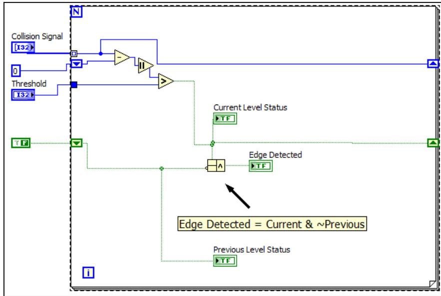
**Figure 43. Collision Signal Edge Detection (LabVIEW Code Segment)**
