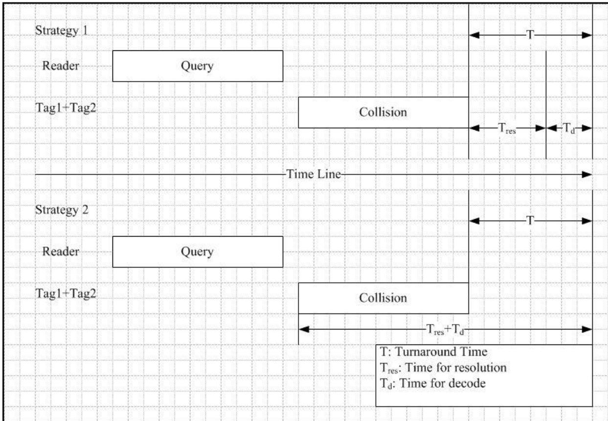
Figure 10. Collision Resolution Timing Strategy
