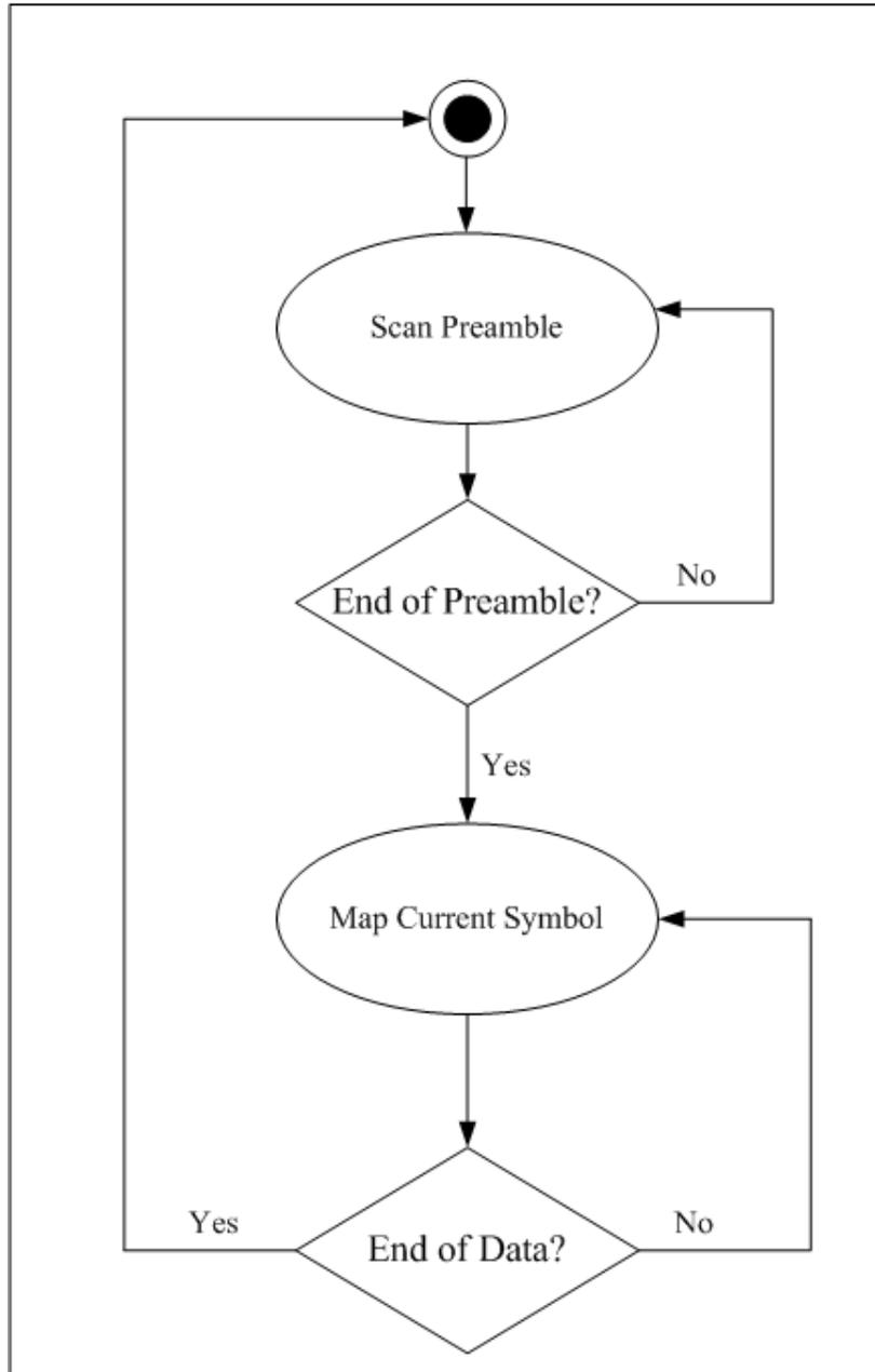
**Figure 61. State Transition of FSM**
