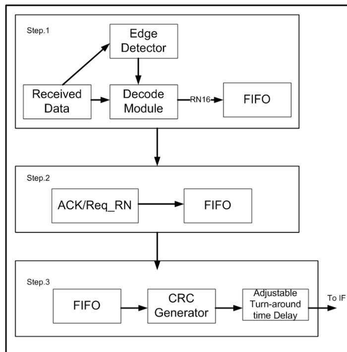
Figure 17. Handshake Processing Unit
