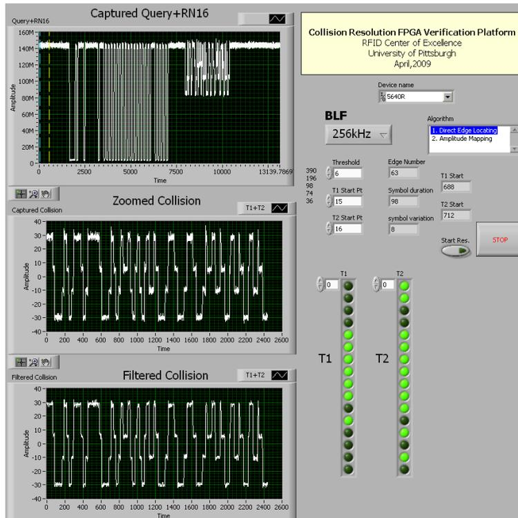
Figure 52. Resolution Result When BLF=256 kHz
