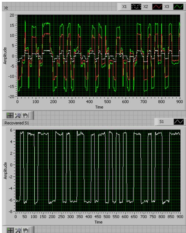
**Figure 109. 3-tag Collision Resolution Result using FastICA in FPGA (BLF=341 kHz)**
