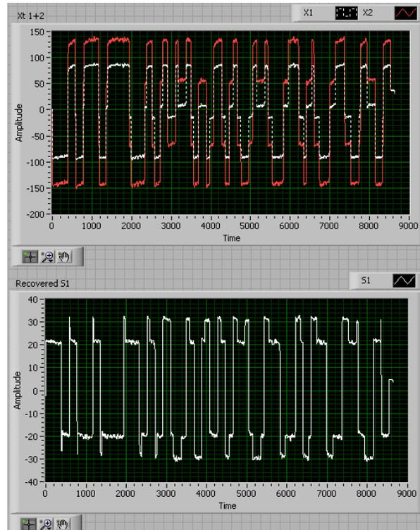
**Figure 99. 2-tag Collision Resolution Result using FastICA in FPGA (BLF=64 kHz)**
