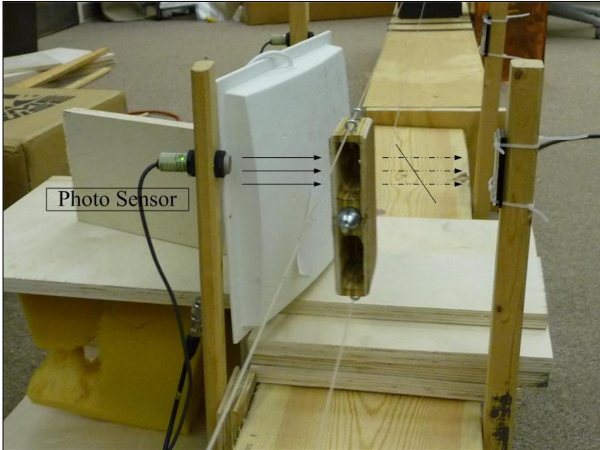
Figure 77. Wooden Bullet Blocking the Sensor Light
