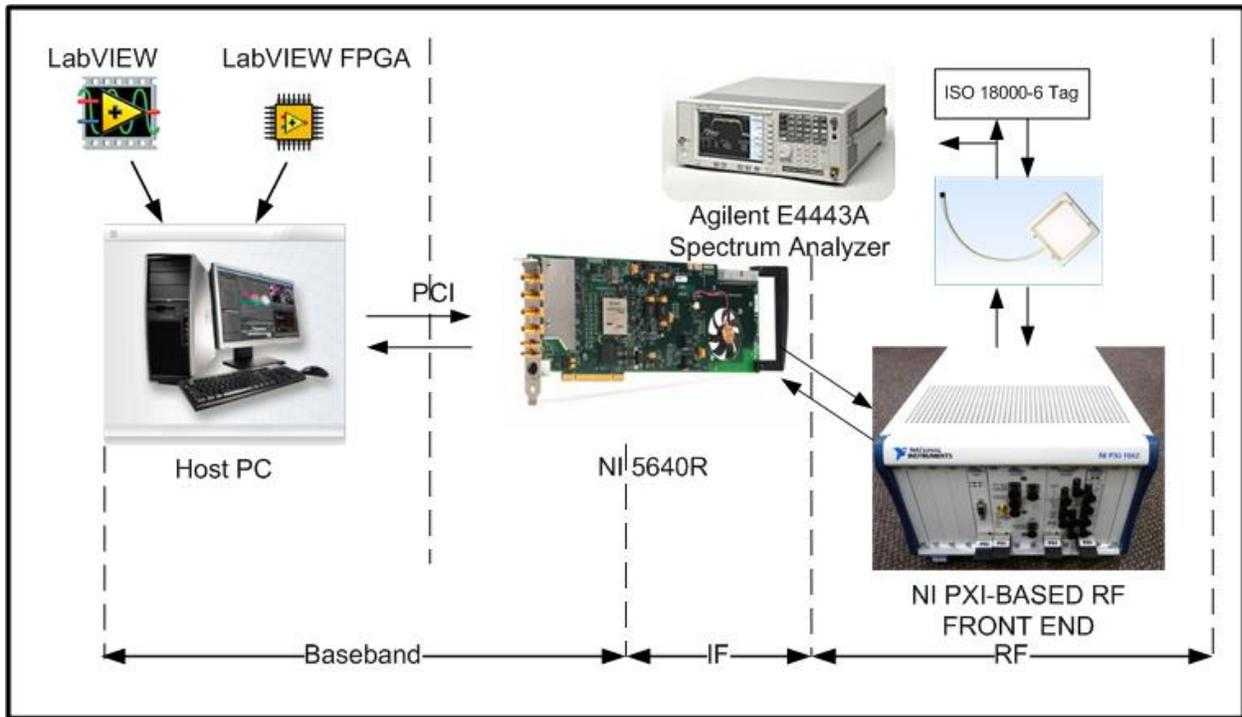
**Figure 11. Platform Hardware Architecture**
