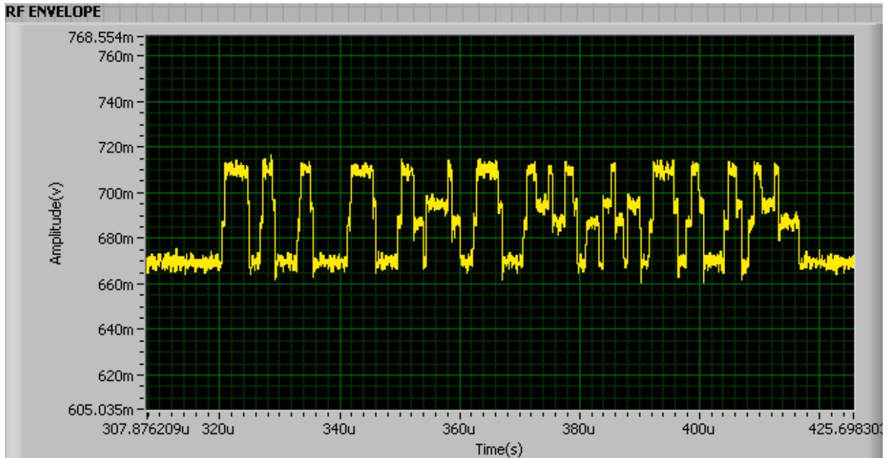
**Figure 81. 2-tag Collision Signal (Speed=12miles/hour, BLF=64 kHz)**
