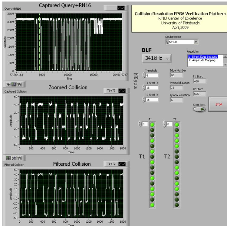
Figure 53. Resolution Result When BLF=341 kHz
