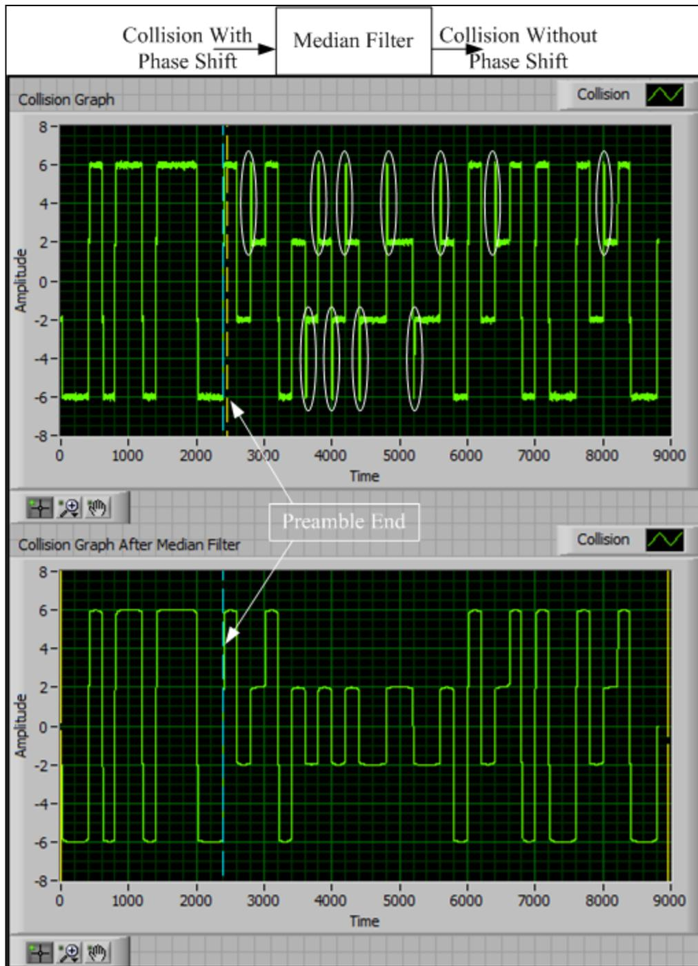
**Figure 70. The Effect of Median Filter**
