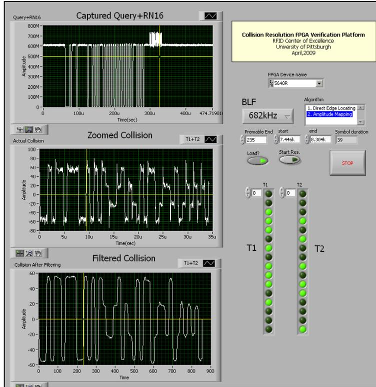
**Figure 68. Collision and Resolved data (BLF=682 kHz)**
