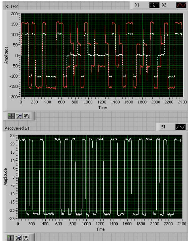
**Figure 101. 2-tag Collision Resolution Result using FastICA in FPGA (BLF=256 kHz)**
