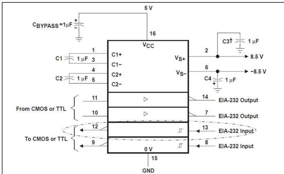
Figure 78. Max232 Port Connections
