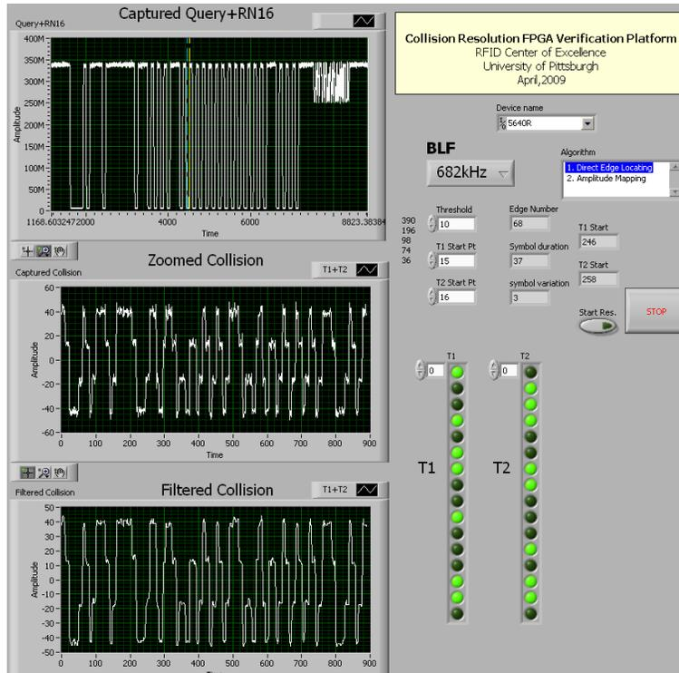
**Figure 54. Resolution Result When BLF=682 kHz**
