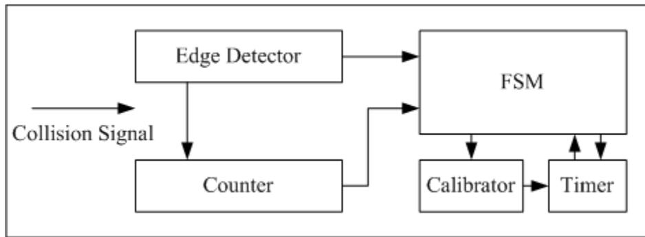
**Figure 39. Implementation of the Algorithm using FSM**
