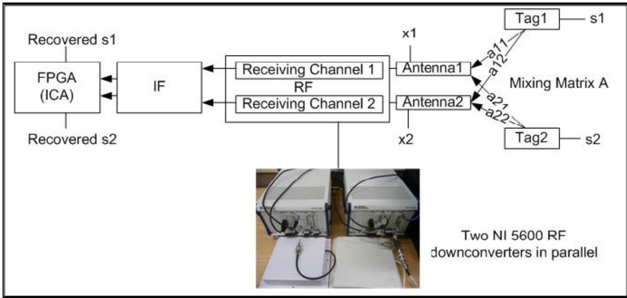
Figure 97. 2-Tag Collision Signal Acquisition Setup for ICA
