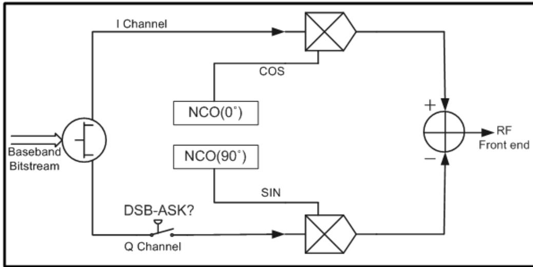
**Figure 13. ASK Modulation Block**
