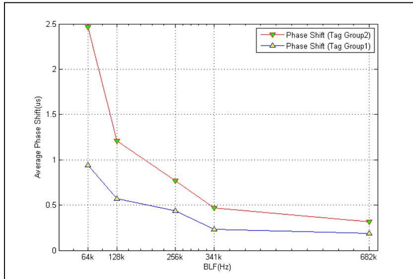
**Figure 27. Tag Phase shift vs. BLF (Manufacturer 1 and Manufacturer 2)**
