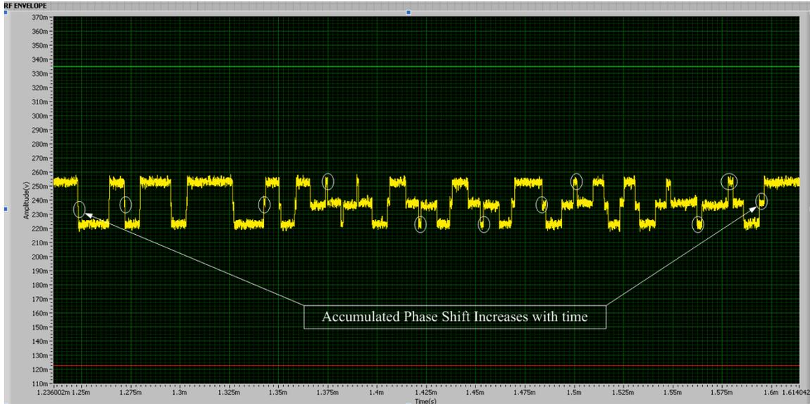
**Figure 26. Accumulated Phase Shift**
