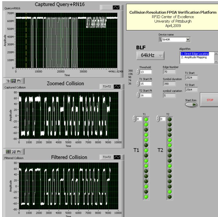
Figure 50. Resolution Result When BLF=64 kHz
