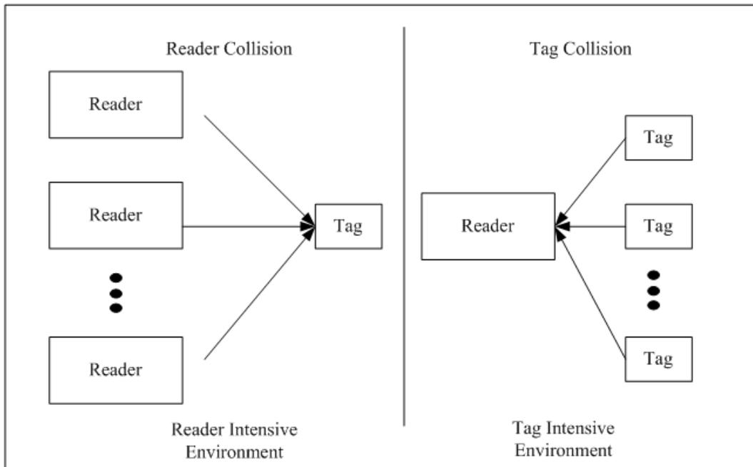
**Figure 1. Passive RFID Collision Situations**
