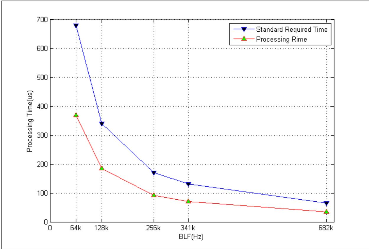
**Figure 105. 2-tag Collision Resolution Processing Time vs. Standard Specification**
