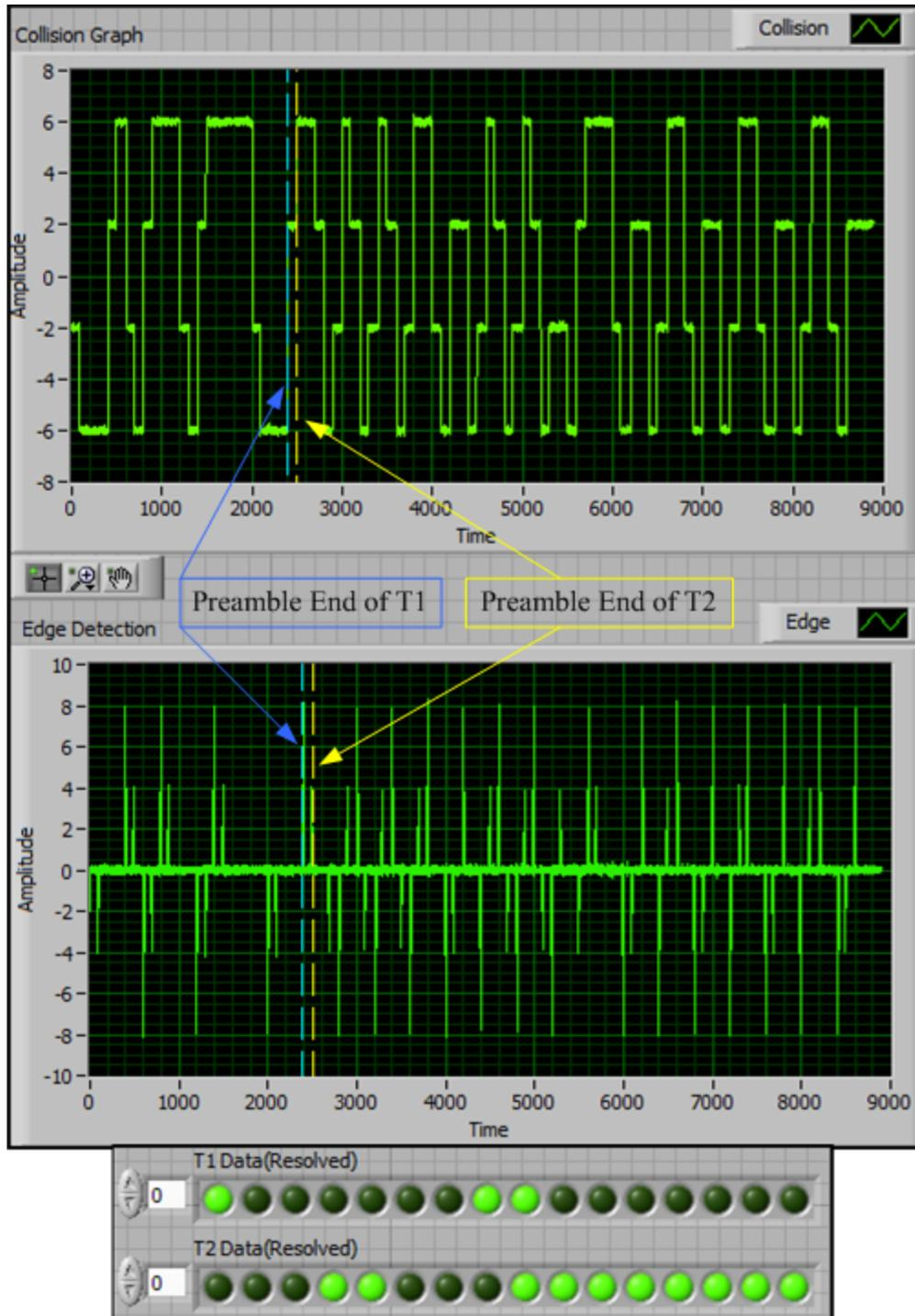
Figure 46. Collision Signal and its Differentiation
