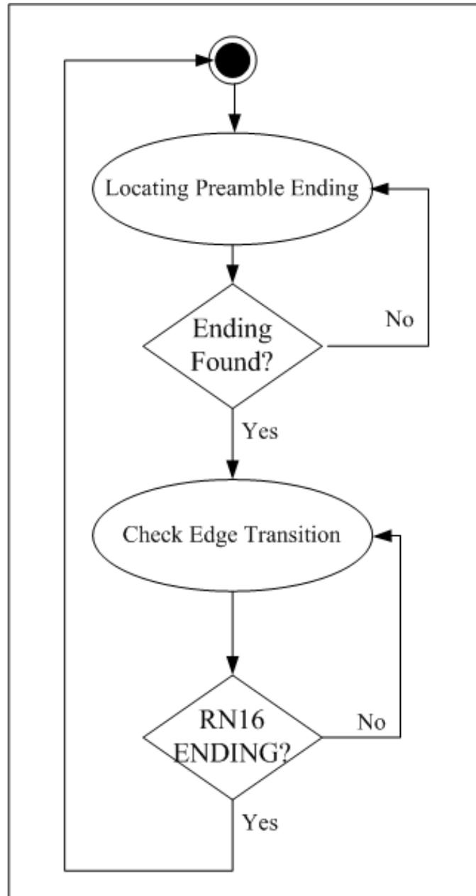
**Figure 40. State Transition of the FSM**
