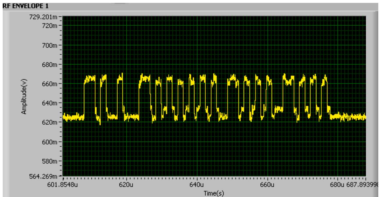
Figure 84. 2-tag Collision Signal (Speed=12miles/hour, BLF=341 kHz)
