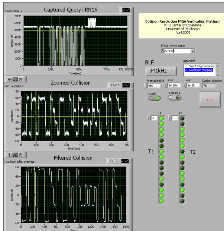
Figure 67. Collision and Resolved data (BLF=341 kHz)
