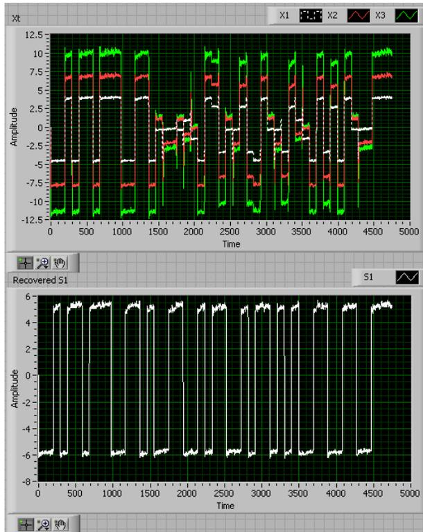
**Figure 106. 3-tag Collision Resolution Result using FastICA in FPGA (BLF=64 kHz)**
