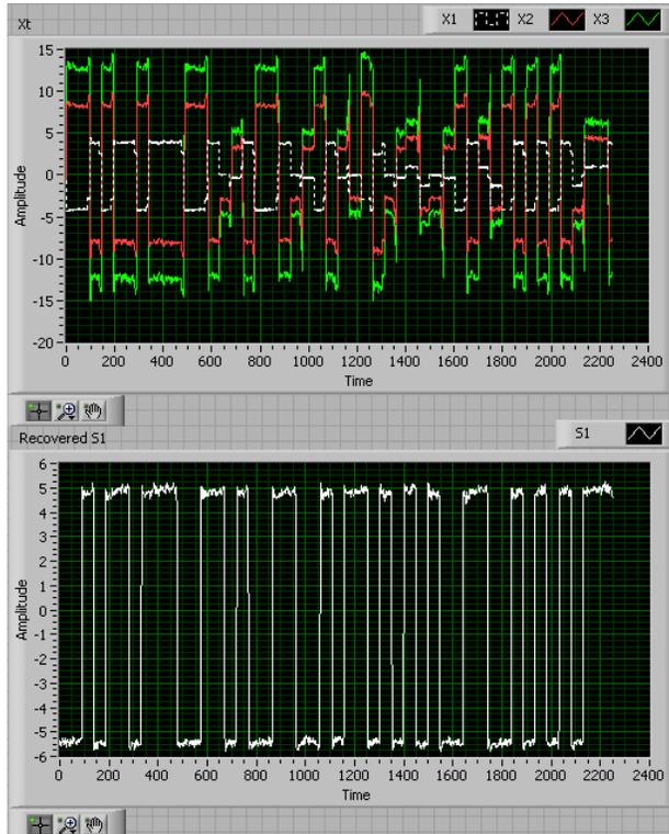
**Figure 107. 3-tag Collision Resolution Result using FastICA in FPGA (BLF=128 kHz)**
