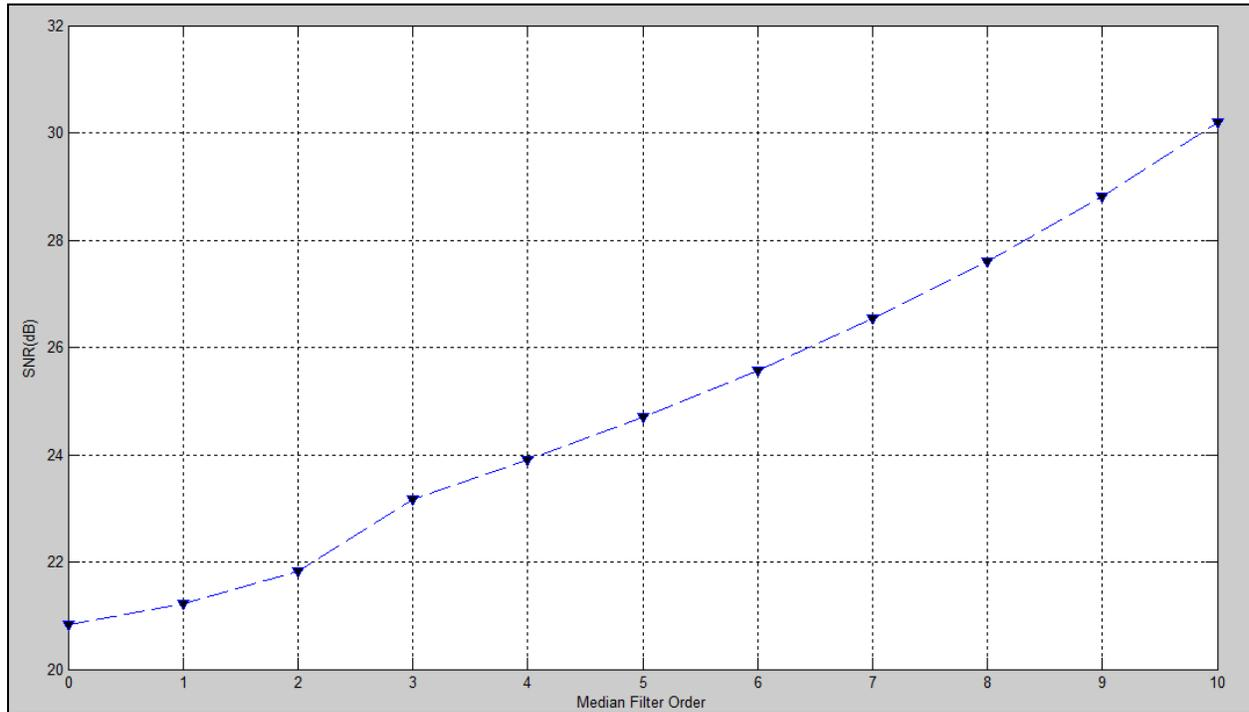
**Figure 31. Median Filter order vs. Processed Signal SNR**
