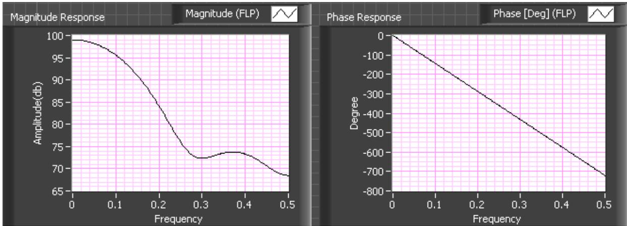
**Figure 14. FIR Filter Magnitude and Phase Response**
