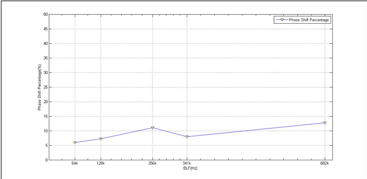
**Figure 28. Tag Phase shift Percentage in Symbol duration vs. BLF (Manufacturer 1)**
