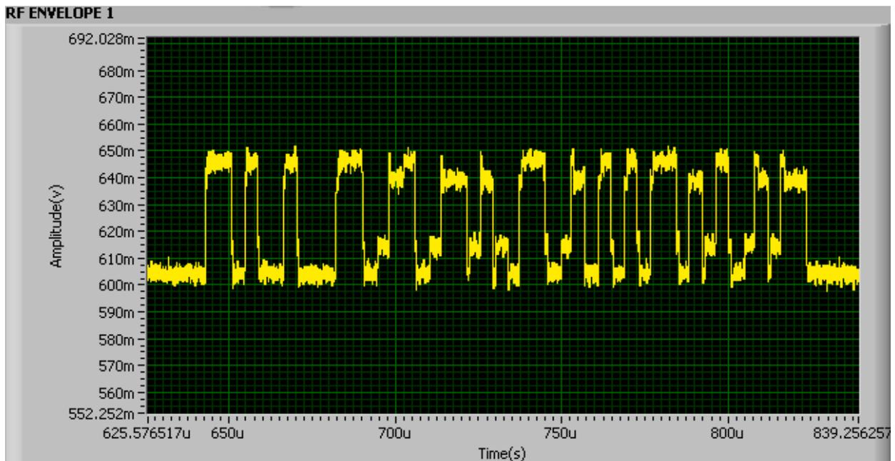
**Figure 82. 2-tag Collision Signal (Speed=12miles/hour, BLF=128 kHz)**
