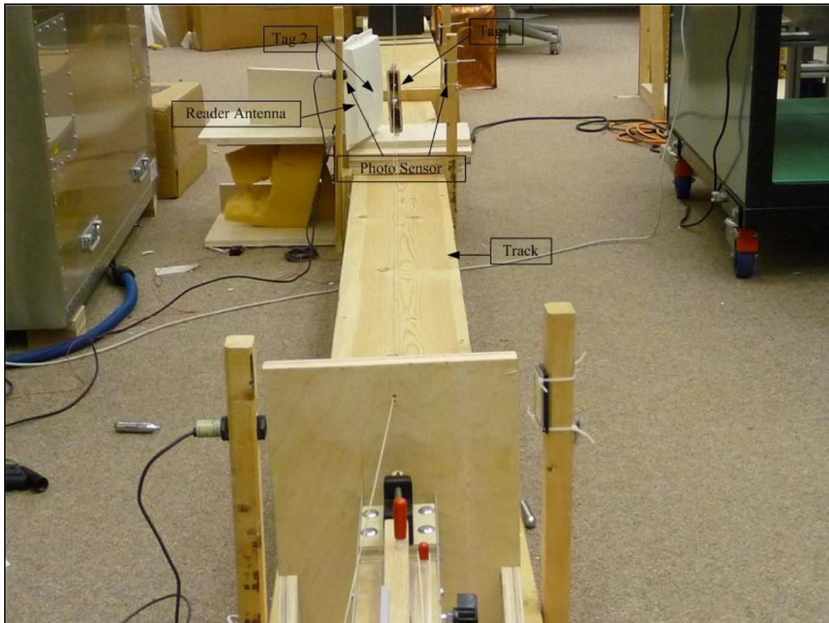
**Figure 74. Moving Tag Data Acquisition Platform (Picture)**
