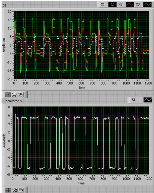
**Figure 108. 3-tag Collision Resolution Result using FastICA in FPGA (BLF=256 kHz)**
