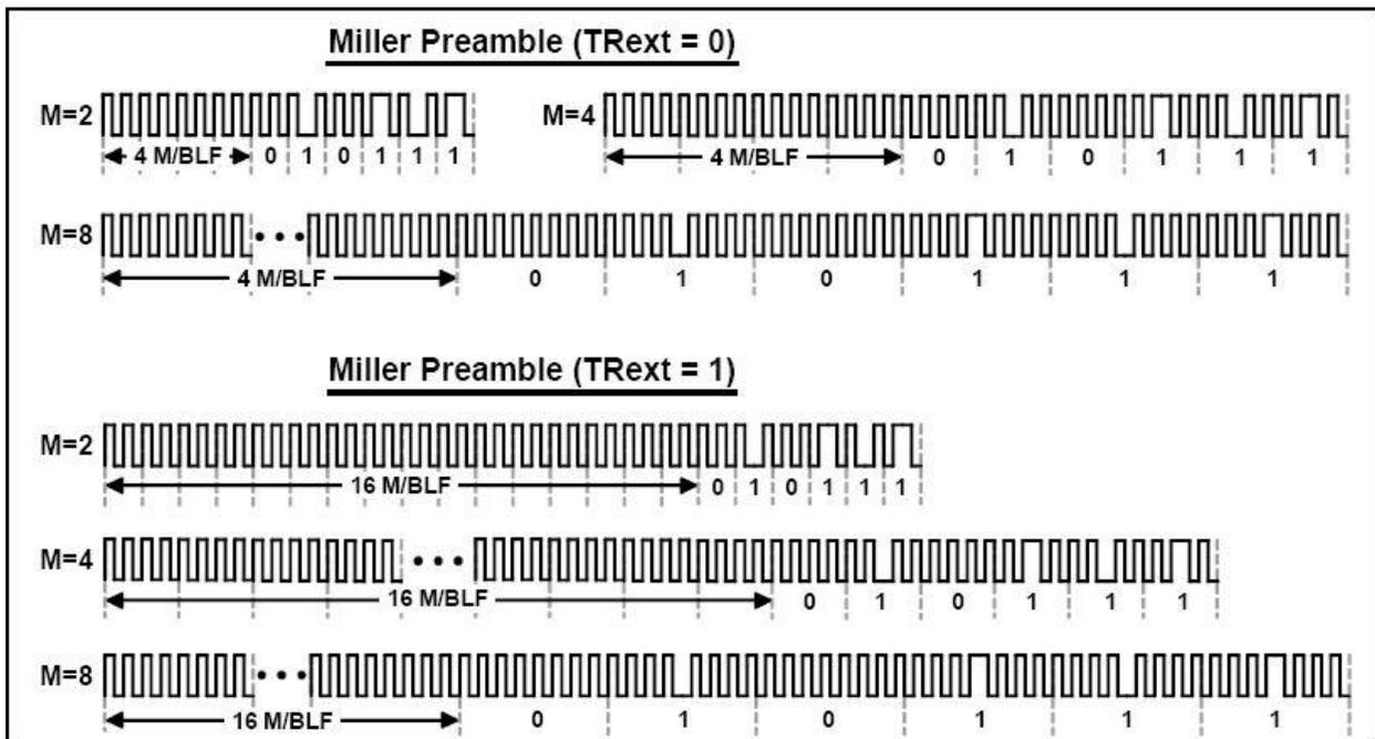
Figure 37. Tag Response Preamble in Miller Subcarrier
