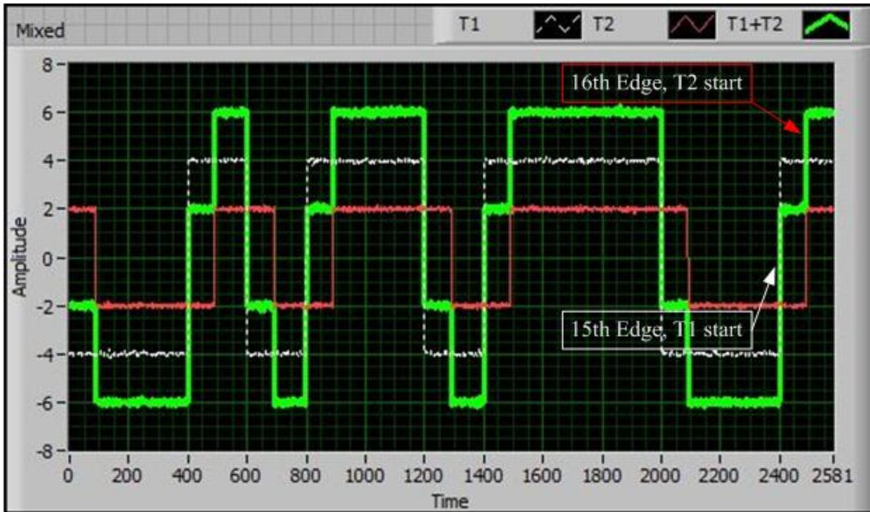
Figure 38. Ending Location of Preambles in Collision
