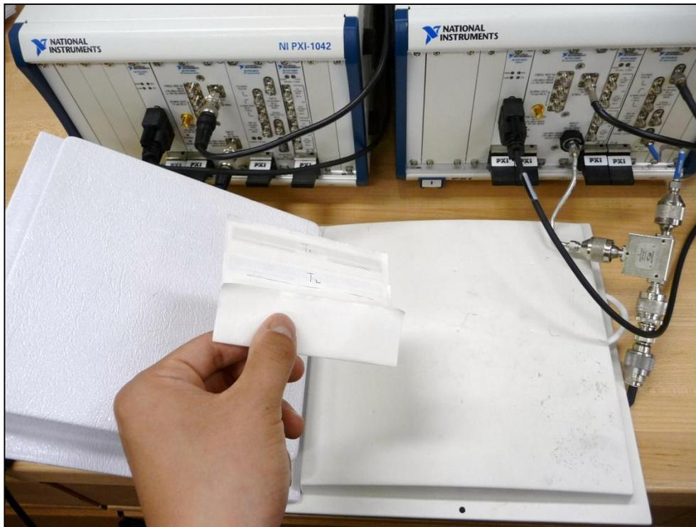
Figure 98. Tag and Antenna Positioning
