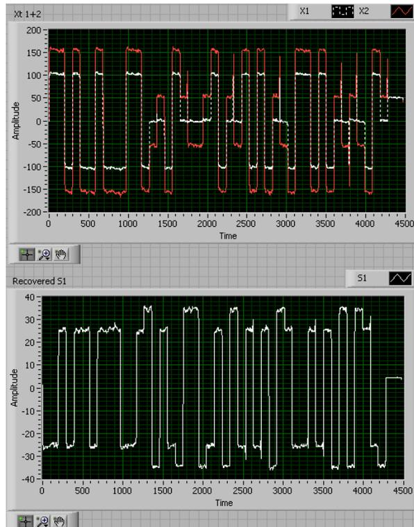
**Figure 100. 2-tag Collision Resolution Result using FastICA in FPGA (BLF=128 kHz)**
