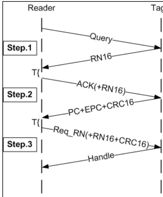
Figure 3. The Three Step Handshake
