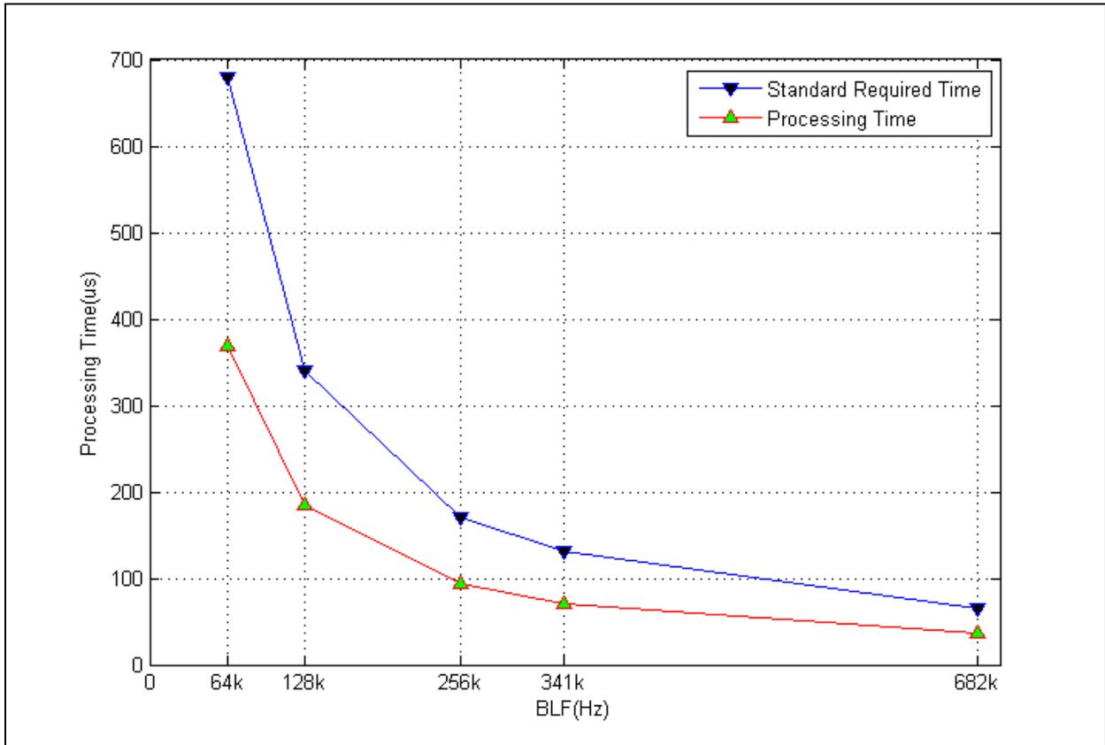
**Figure 111. 3-tag Collision Resolution Processing Time vs. Standard Specification**
