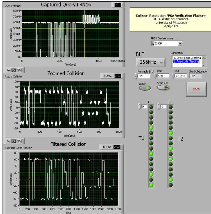
Figure 66. Collision and Resolved data (BLF=256 kHz)
