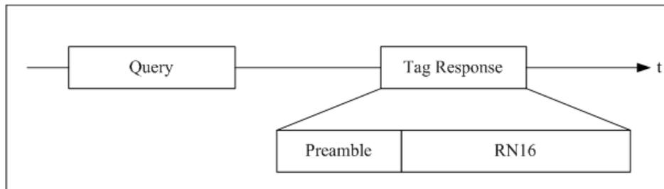
Figure 35. Tag Response Frame Architecture
