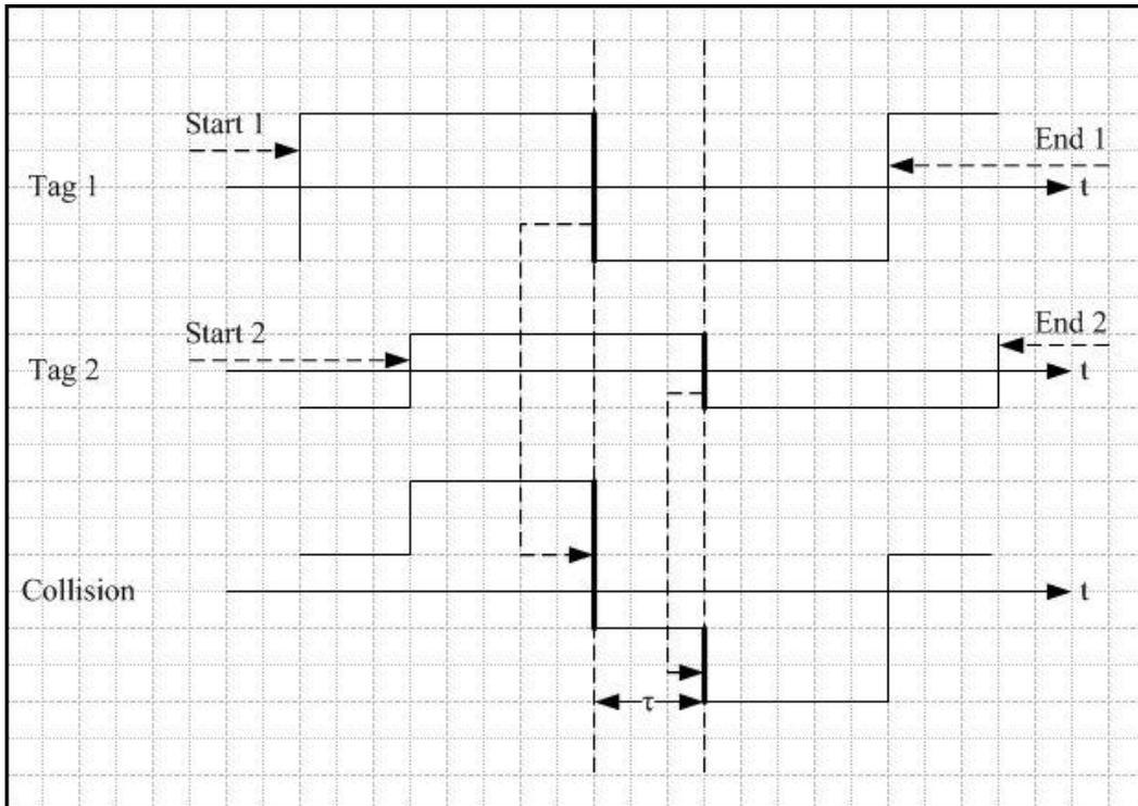
Figure 32. Superposition of Two Formation-0 Symbols
