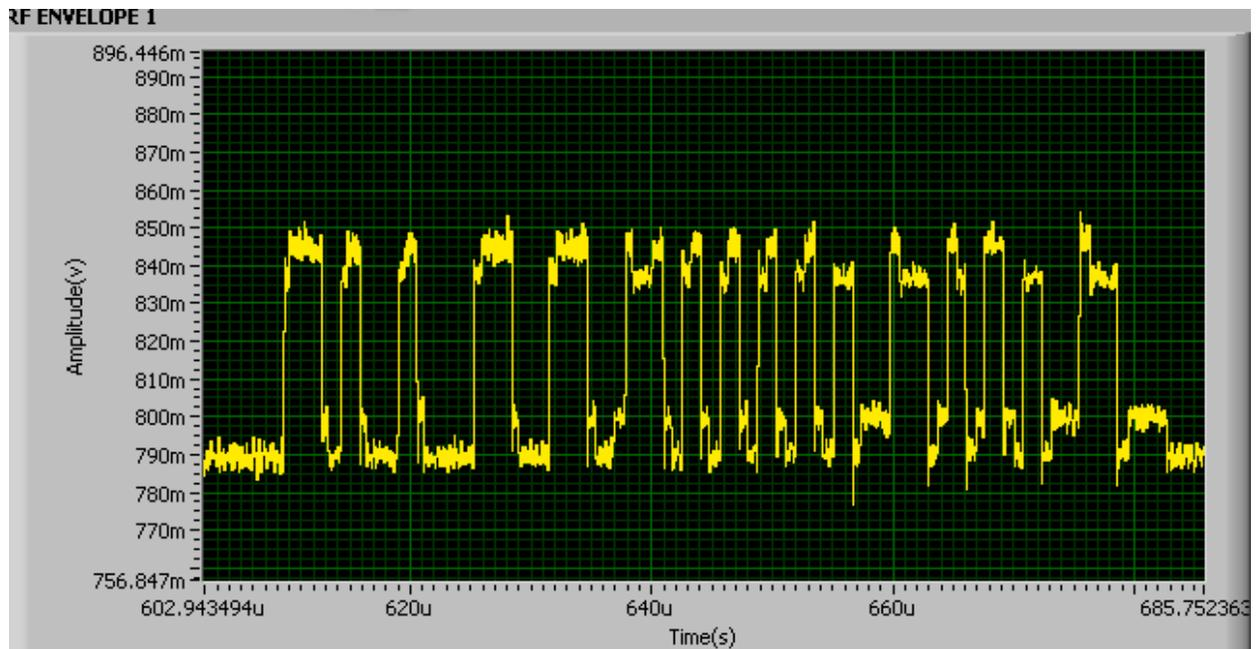
**Figure 89. 2-tag Collision Signal (Speed=25miles/hour, BLF=341 kHz)**
