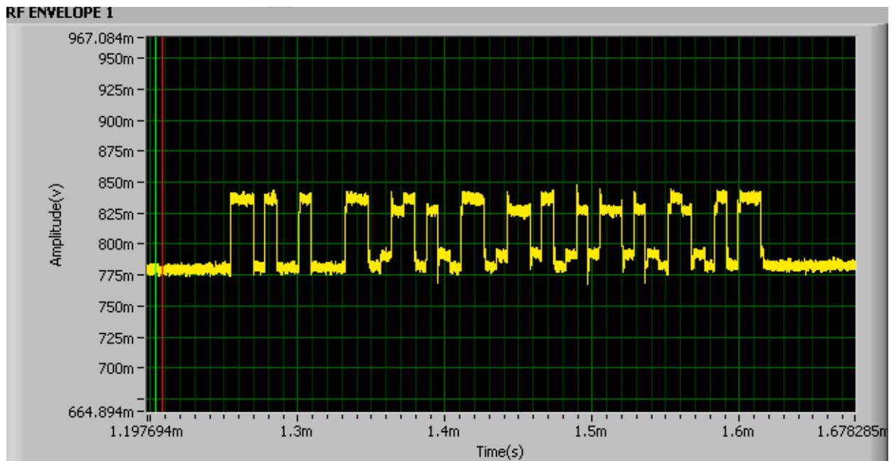
**Figure 86. 2-tag Collision Signal (Speed=25miles/hour, BLF=64 kHz)**
