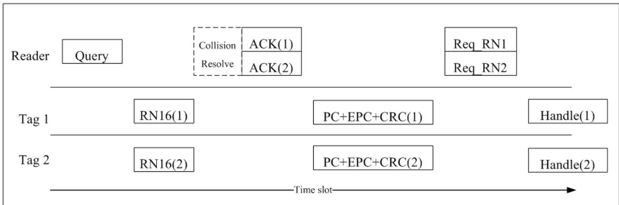
**Figure 9. Simultaneous Tag Access with Collision Resolution**
