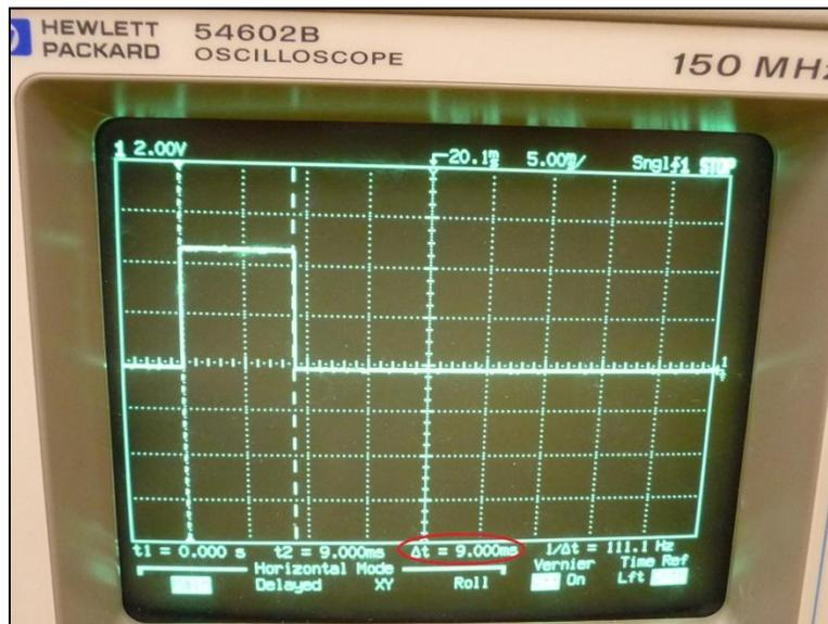
Figure 80. Pulse Width corresponding to 25 miles/hour
