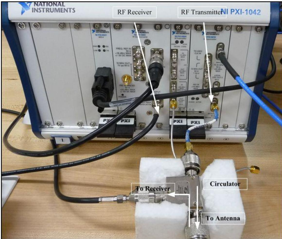
**Figure 25. RF Front End Connection with Circulator**
