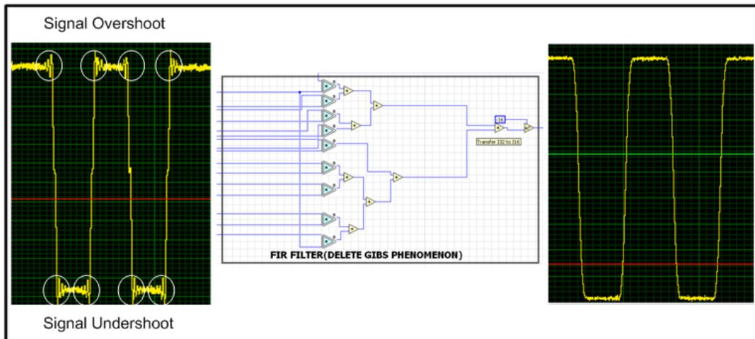
**Figure 15. Signal Smoothing with 8-order FIR Filter**
