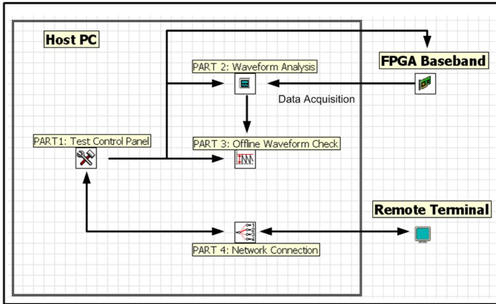
Figure 12. Platform Software Architecture
