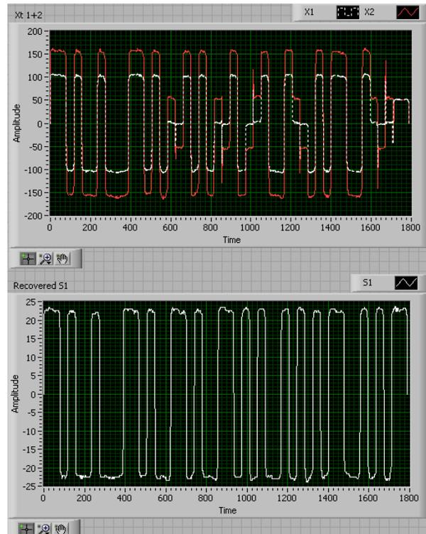
**Figure 102. 2-tag Collision Resolution Result using FastICA in FPGA (BLF=341 kHz)**
