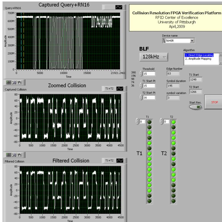
Figure 51. Resolution Result When BLF=128 kHz
