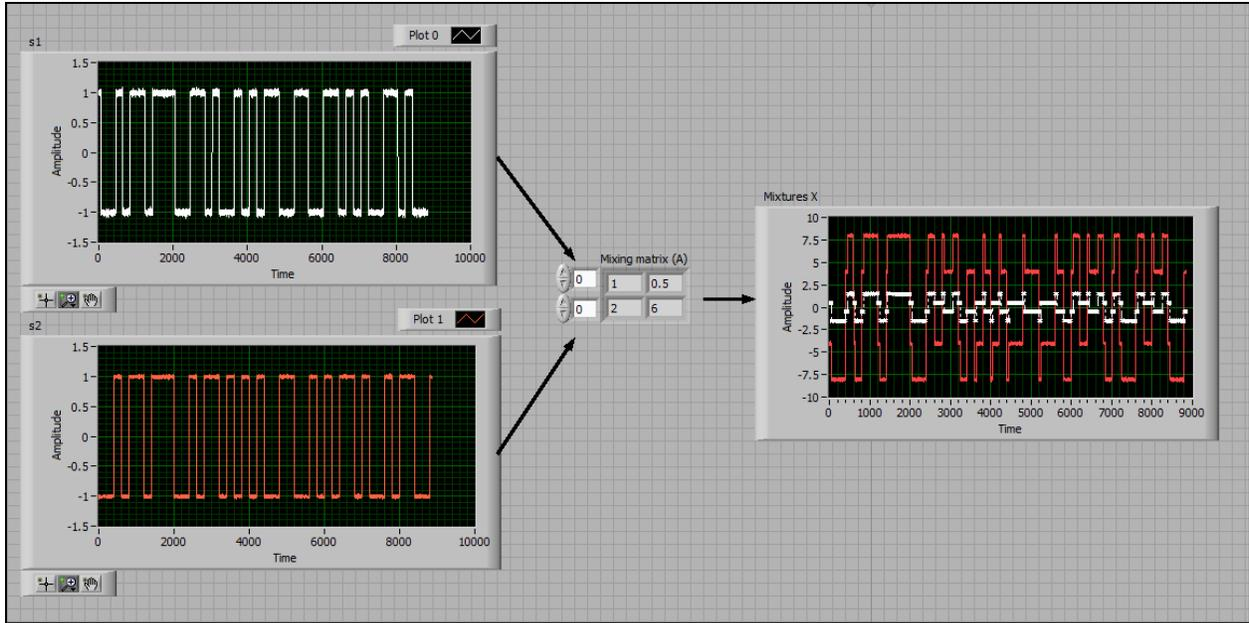
Figure 92. Simulated Tag Signal Mixing
