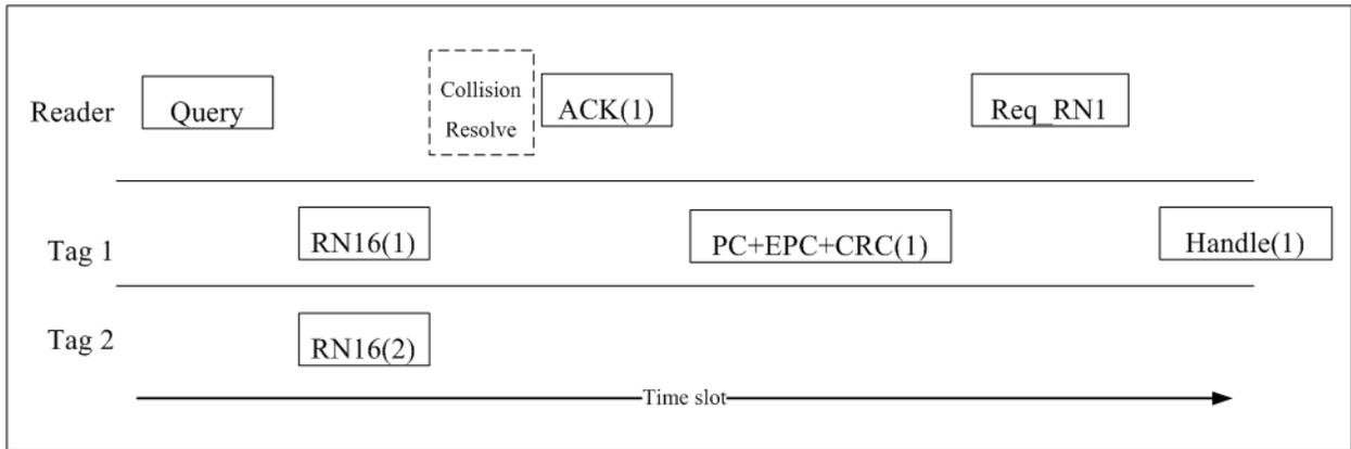
**Figure 8. Selective Tag Access with Collision Resolution**
