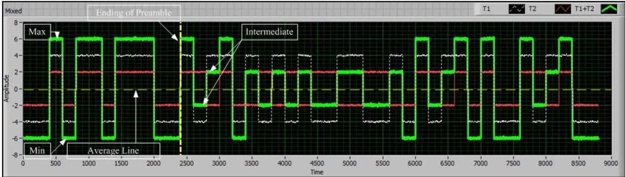
**Figure 58. Example Superposition of Tag Responses without Phase shift**
