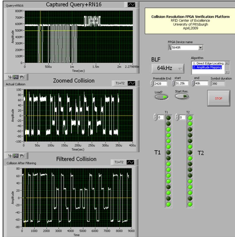
Figure 64. Collision and Resolved data (BLF=64 kHz)
