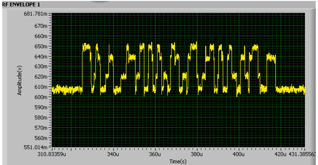
Figure 83. 2-tag Collision Signal (Speed=12miles/hour, BLF=256 kHz)
