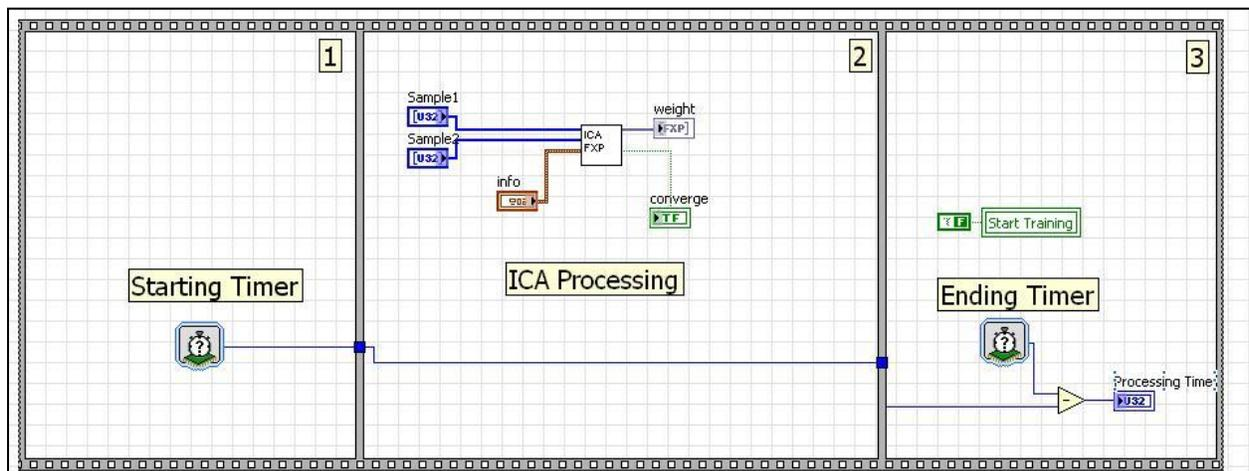
**Figure 104. Processing Time Recording (LabVIEW FPGA code Segment)**
