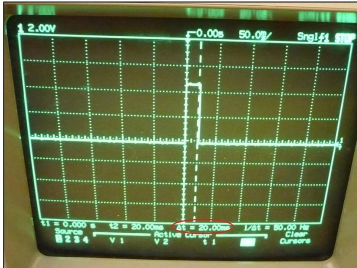
Figure 79. Trigger Pulse Width Corresponding to 12 miles/hour
