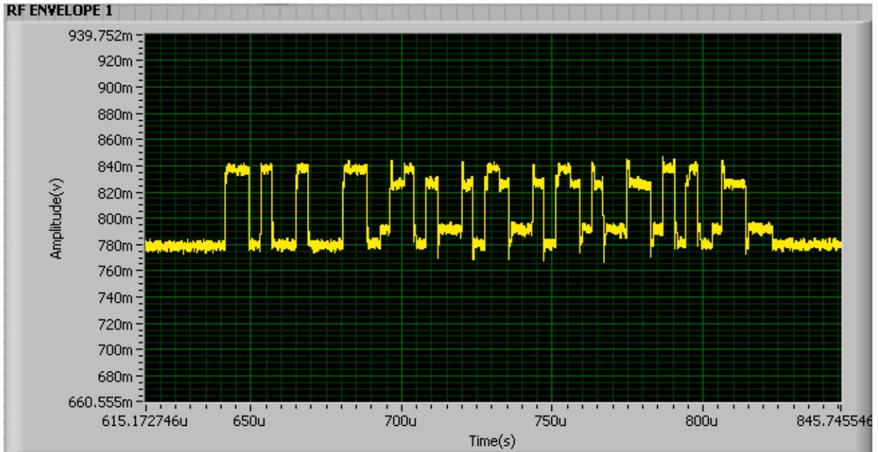
Figure 87. 2-tag Collision Signal (Speed=25miles/hour, BLF=128 kHz)
