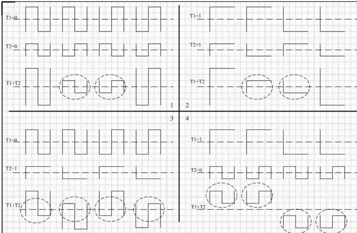
**Figure 57. Collision Patterns**
