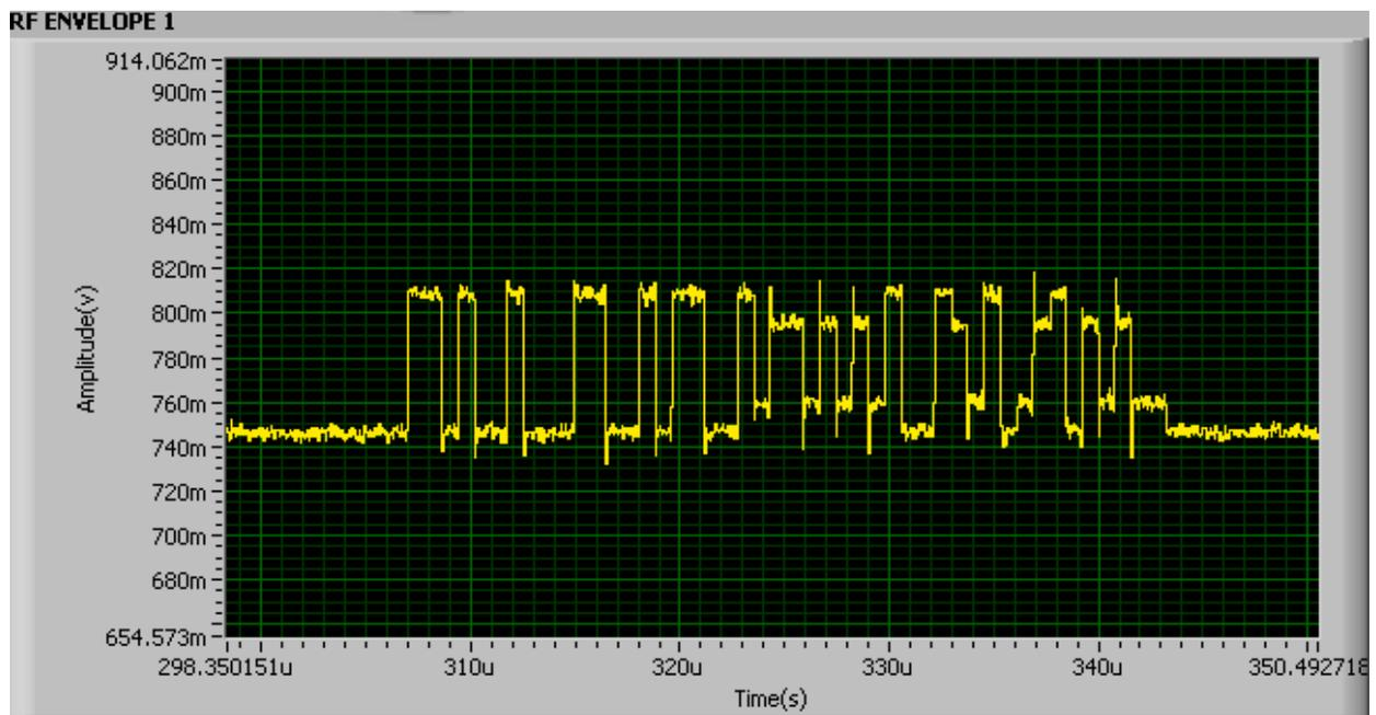
**Figure 90. 2-tag Collision Signal (Speed=25miles/hour, BLF=682 kHz)**
