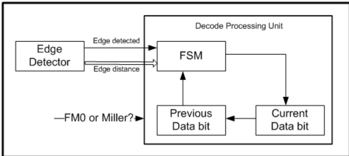
Figure 16. Decode Module Architecture
