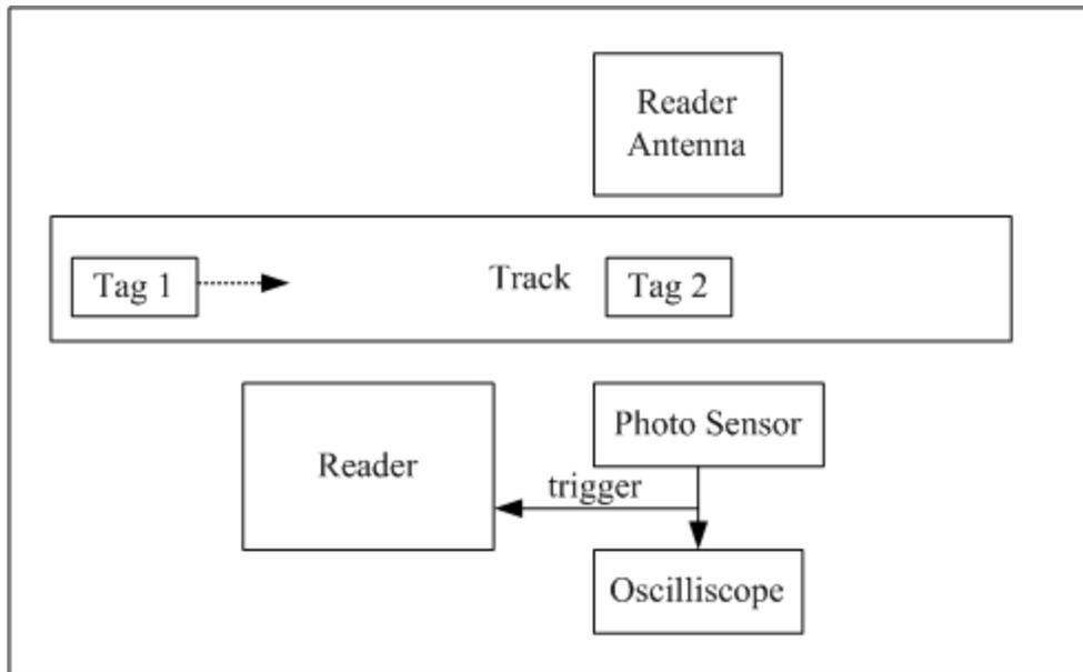
**Figure 73. Moving Tag Data Acquisition Platform**
