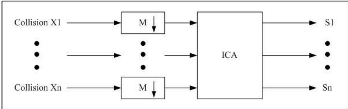
**Figure 96. Collision Signal down Sampling**
