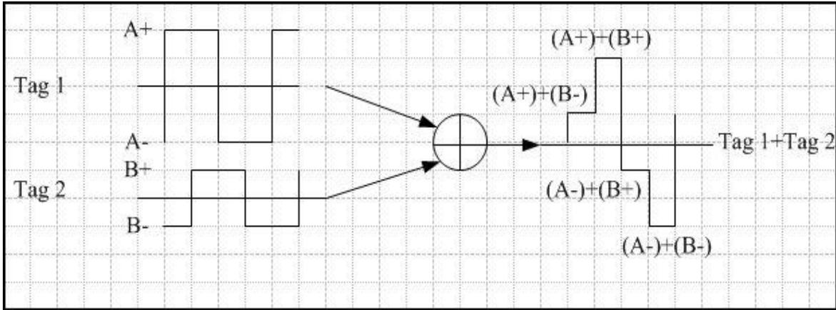
**Figure 24. Linear Additive Model of Tag Responses**
