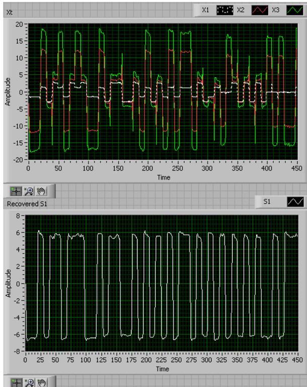
**Figure 110. 3-tag Collision Resolution Result using FastICA in FPGA (BLF=682 kHz)**
