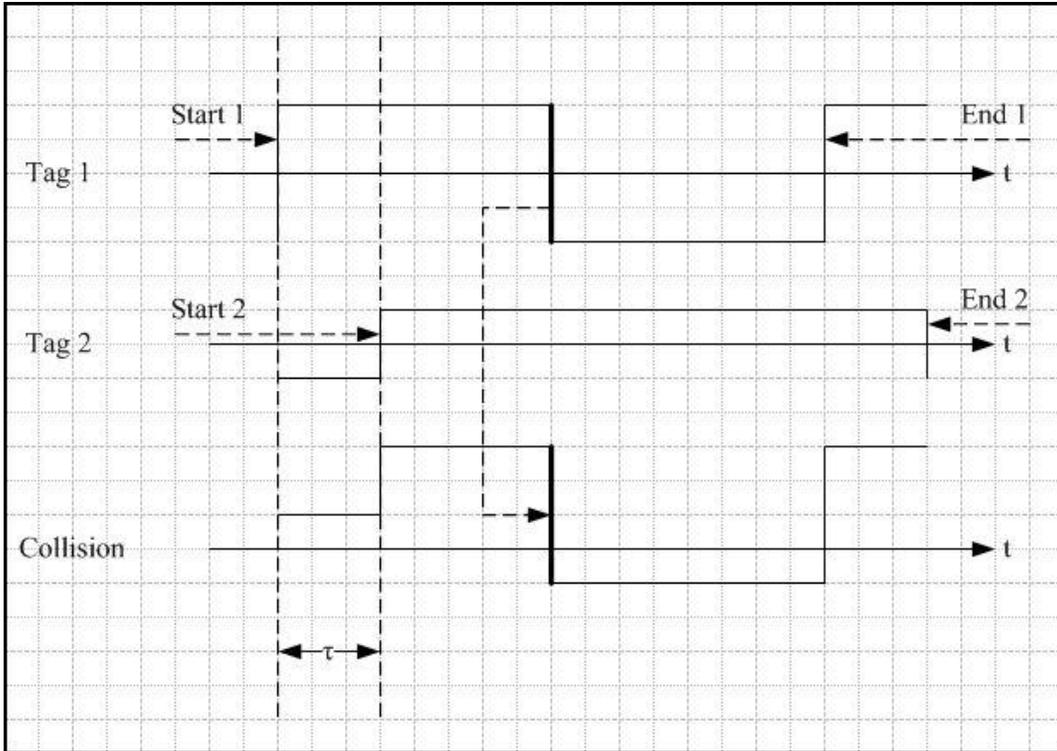
Figure 34. Superposition of Formation-0 Symbol and Formation-1 Symbol
