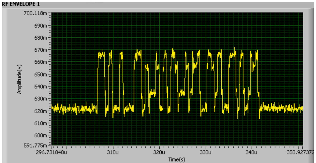
**Figure 85. 2-tag Collision Signal (Speed=12miles/hour, BLF=682 kHz)**
