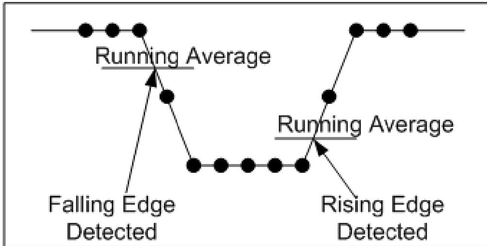
Figure 41. The Running Mean Calculation
