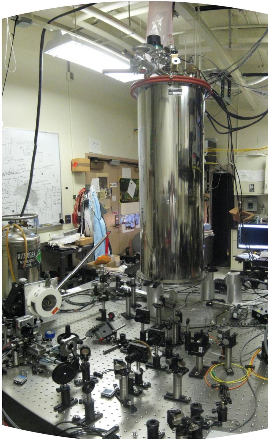
Figure C1: Photograph of cryostats. The continuous flow cryostat is on left. The magneto-optical cryostat is on the right. The plastic bag used for sample exchanges is visible at the top of the magneto-optical cryostat. Miscellaneous optics are visible in the foreground.
