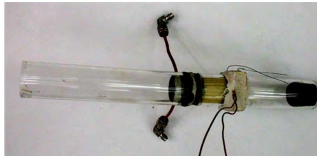
Figure 16: Assembled TAE test bed.
