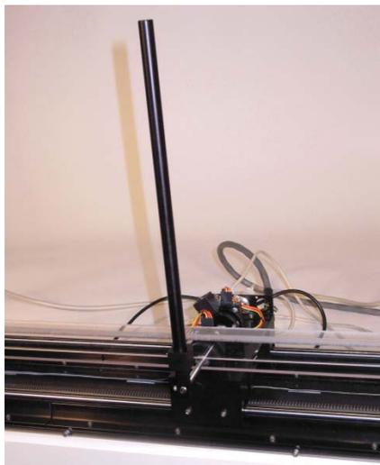
**Figure 1.** Inverted Pendulum
