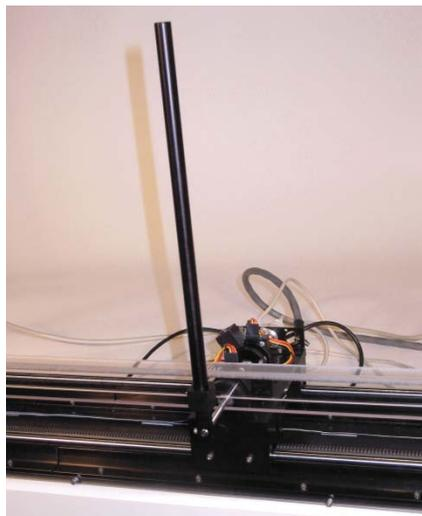
**Figure 1.** Inverted Pendulum
