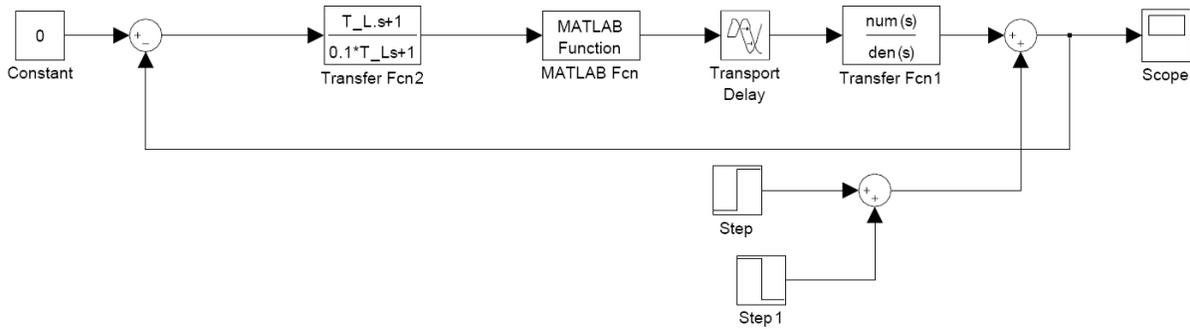
**Figure 3.** Simulink Model of On-Off Controller
