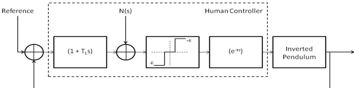
**Figure 2.** On-Off controller model
