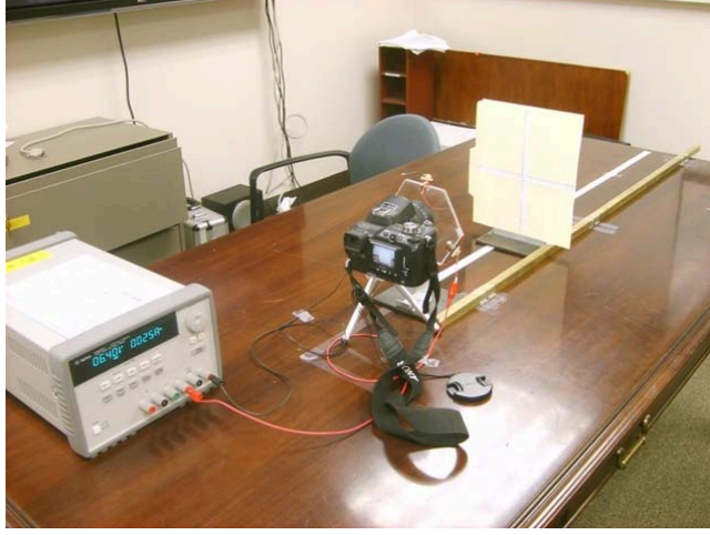
Figure 35: Prototype with laser beams structured light and high resolution digital camera used in our experiment.
