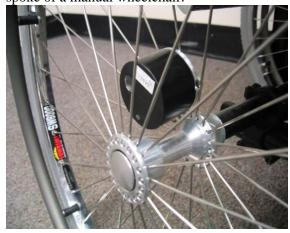
Figure 7. Illustrates the power data logger device.
